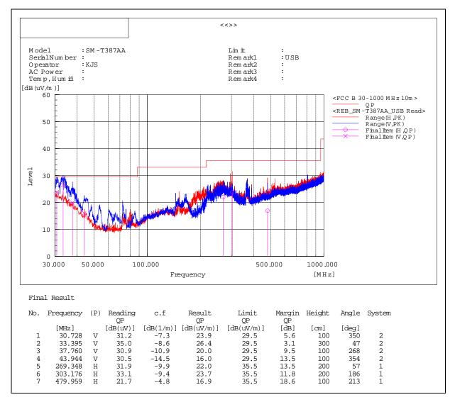
Note 1) Receiving antenna polarization : Horizontal, Vertical Test Distance : 10 m, Antenna Height : 1 to 4 meters Level (QP) = Reading (QP) + c.f (Antenna Factor + Cable Loss - Amp. Gain) Margin (QP) = Limit – Level (QP) QP = Quasi-Peak, c.f = Correction Factor
