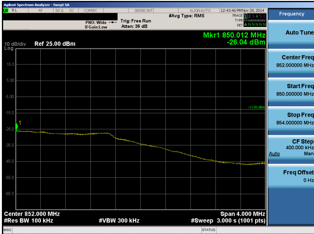
Plot 6-74. Upper Extended Band Edge Plot (Band 5 – Band 5 – 3.0MHz QPSK – RB Size 15)
