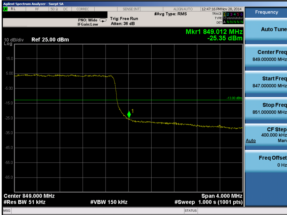
Plot 6-77. Upper Band Edge Plot (Band 5 – 5.0MHz QPSK – RB Size 25)
