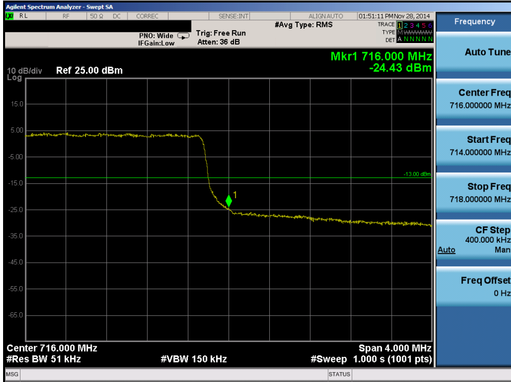
Plot 6-63. Upper Band Edge Plot (Band 17 – 5.0MHz QPSK – RB Size 25)
