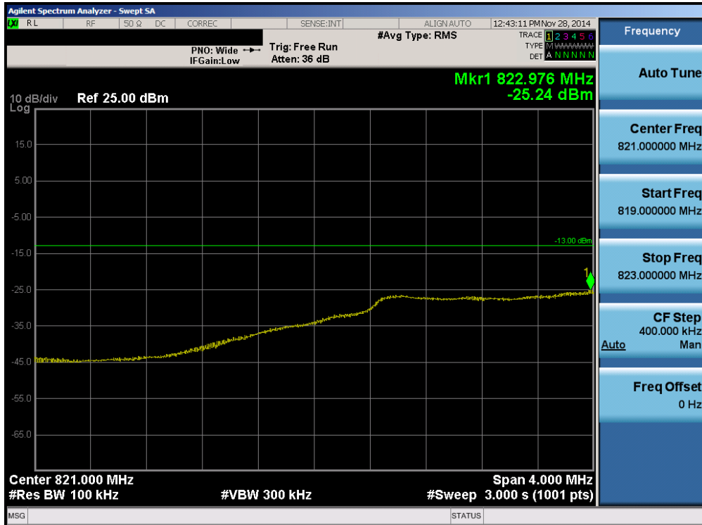
Plot 6-72. Lower Extended Band Edge Plot (Band 5 – 3.0MHz QPSK – RB Size 15)
