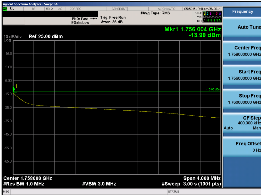
Plot 6-92. Upper Extended Band Edge Plot (Band 4 – 5.0MHz QPSK – RB Size 25)
