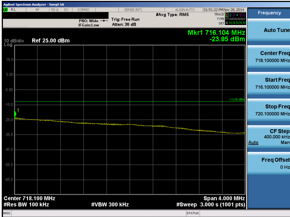
Plot 6-64. Upper Extended Band Edge Plot (Band 17 – 5.0MHz QPSK – RB Size 25)
