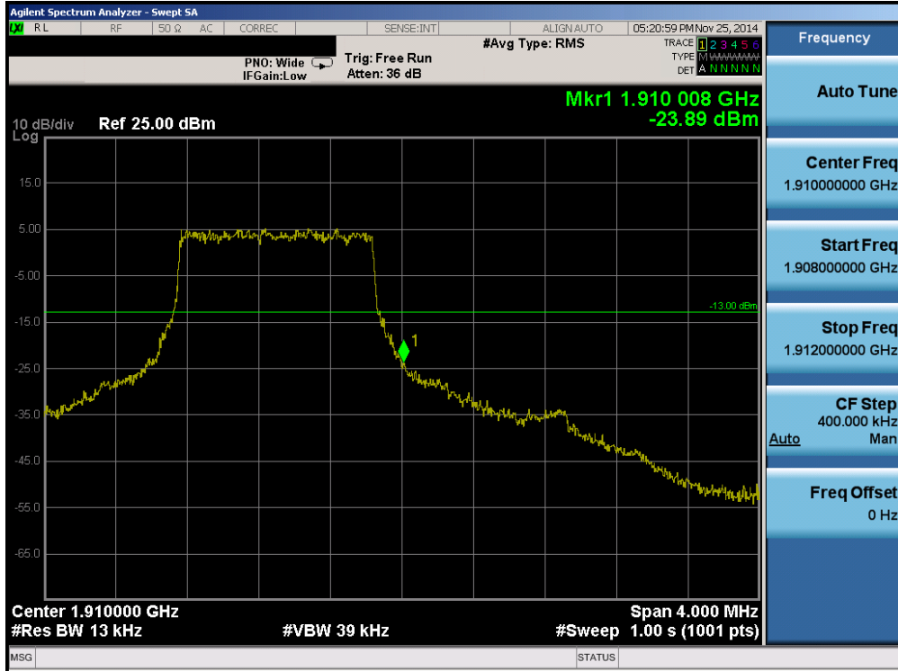
Plot 6-107. Upper Band Edge Plot (Band 2 – 1.4MHz QPSK – RB Size 6)
