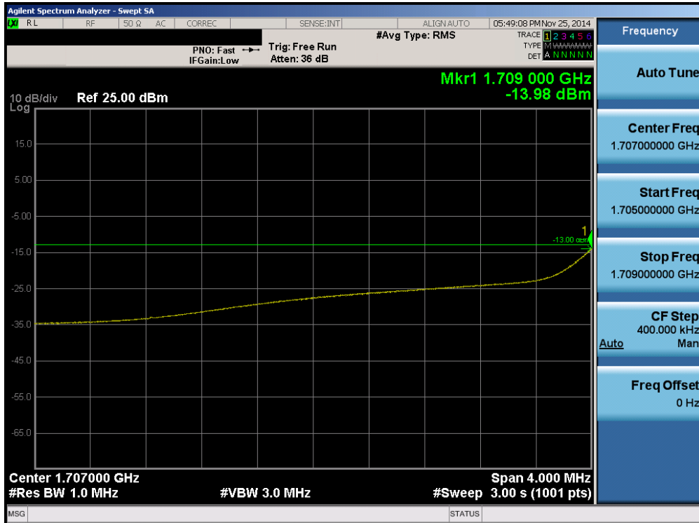
Plot 6-90. Lower Extended Band Edge Plot (Band 4 – 5.0MHz QPSK – RB Size 25)
