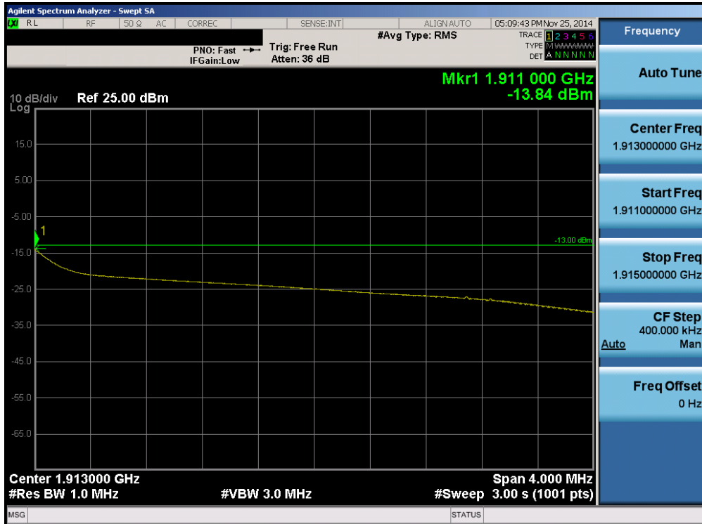
Plot 6-116. Upper Extended Band Edge Plot (Band 2 – 5.0MHz QPSK – RB Size 25)
