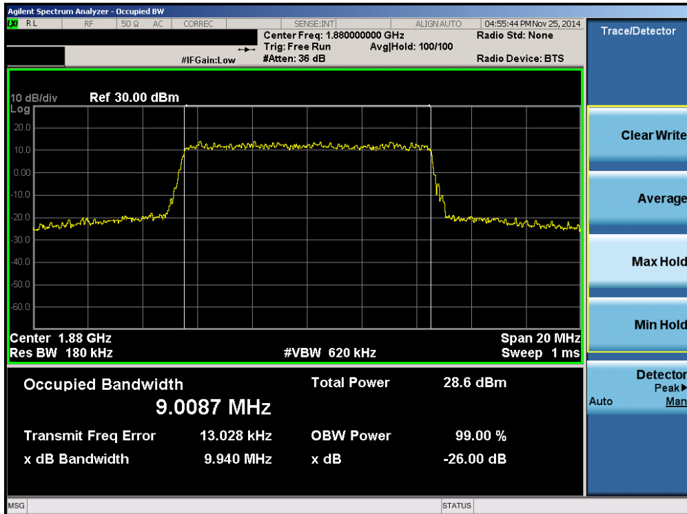
Plot 6-32. Occupied Bandwidth Plot (Band 2 – 10.0MHz 16-QAM – RB Size 50)
