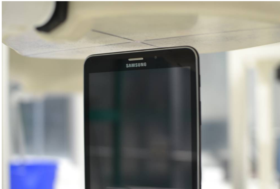
SAR Test Setup Photo 8 – Top Edge at 0.9 cm
