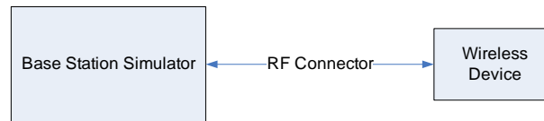
Figure 9-1 Power Measurement Setup
