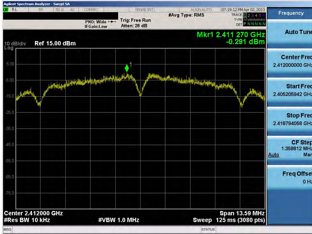
Plot 6-18. Power Spectral Density Plot (802.11b – Ch. 1)
