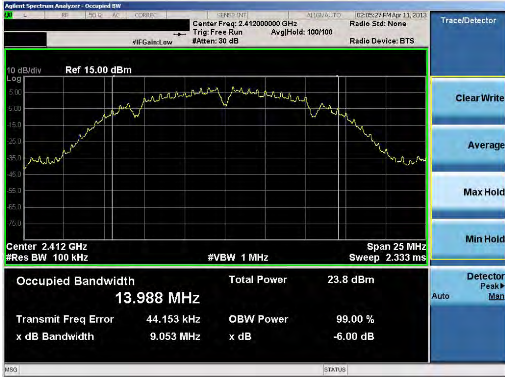
Plot 6-1. 6dB Bandwidth Plot (802.11b – Ch. 1)
