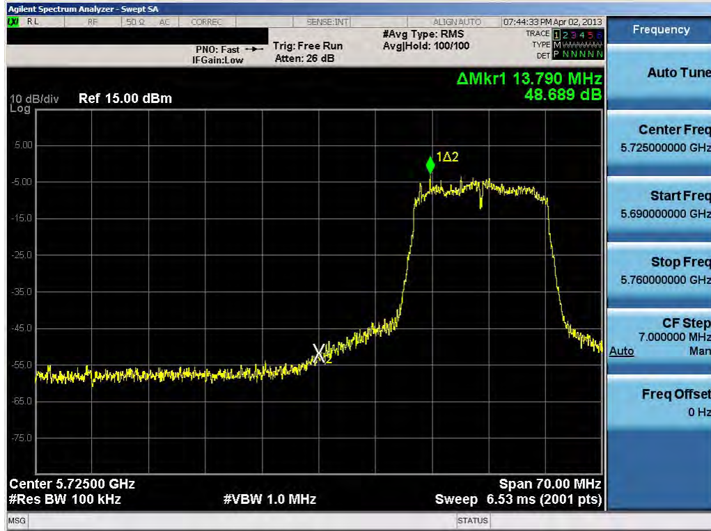
Plot 6-41. Band Edge Plot (802.11a – Ch. 149)
