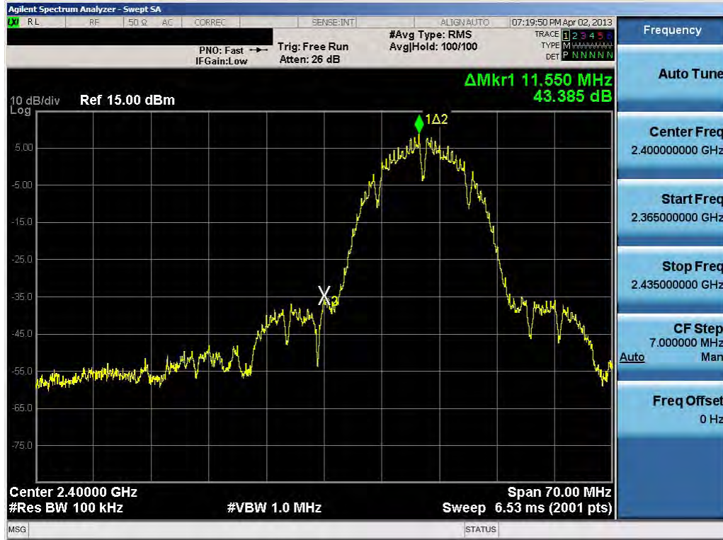
Plot 6-35. Band Edge Plot (802.11b – Ch. 1)
