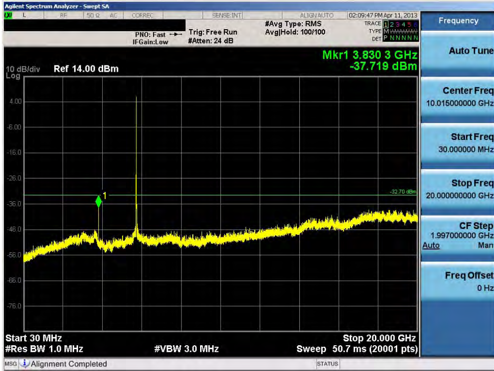
Plot 6-53. Conducted Spurious Plot (802.11a – Ch. 149)
