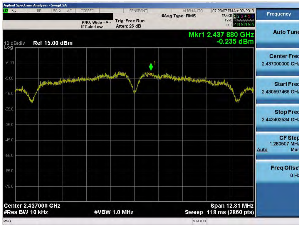
Plot 6-19. Power Spectral Density Plot (802.11b – Ch. 6)
