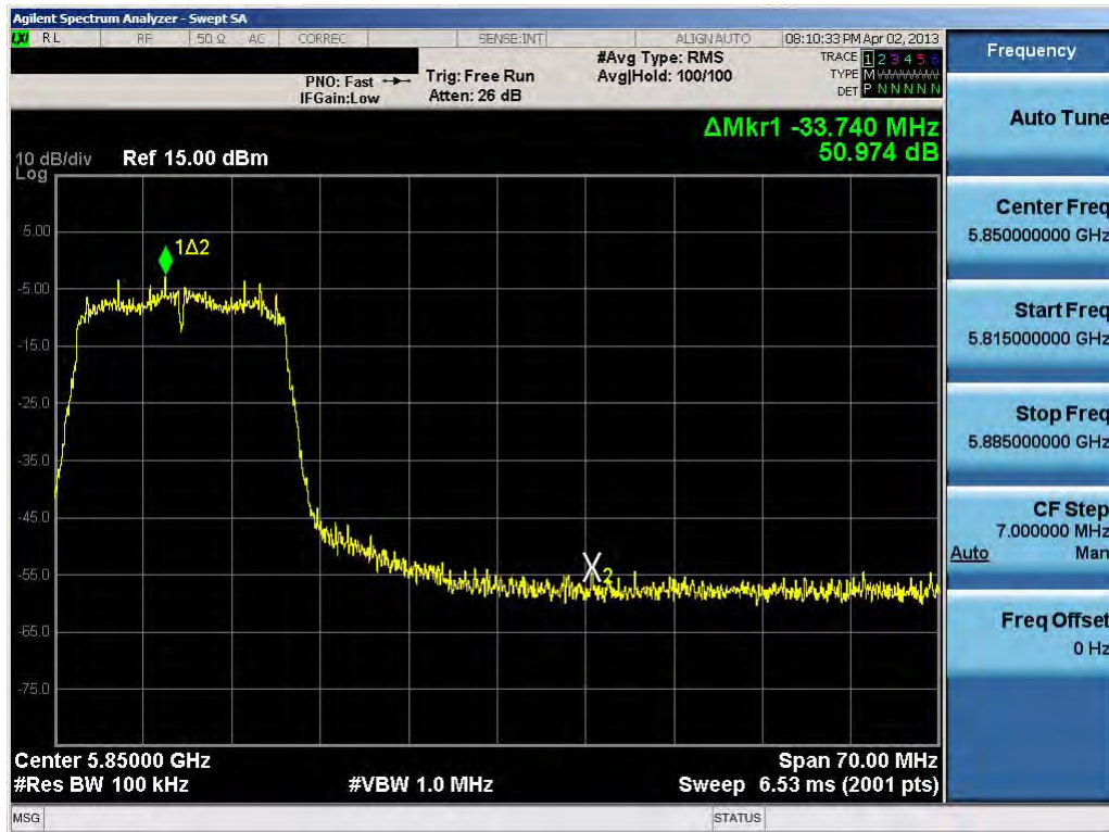
Plot 6-42. Band Edge Plot (802.11a – Ch. 165)
