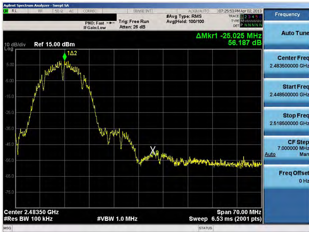
Plot 6-36. Band Edge Plot (802.11b – Ch. 11)
