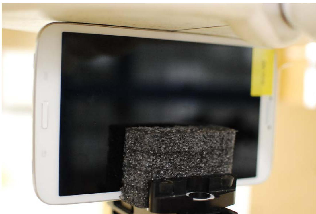
SAR Test Setup Photo 2 - Left Side at 0.0 cm
