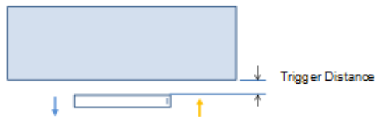
Proximity Sensor Trigger Distance Assessment KDB 616217 §6.2, Rear
