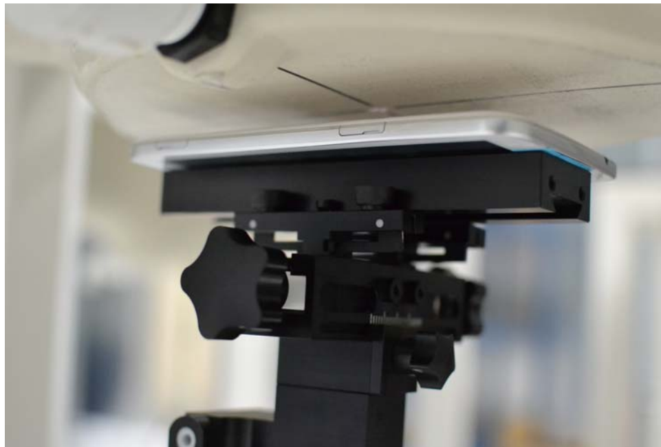
SAR Test Setup Photo 2 – Back Side at 1.5 cm
