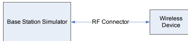
Figure 9-1 Power Measurement Setup
