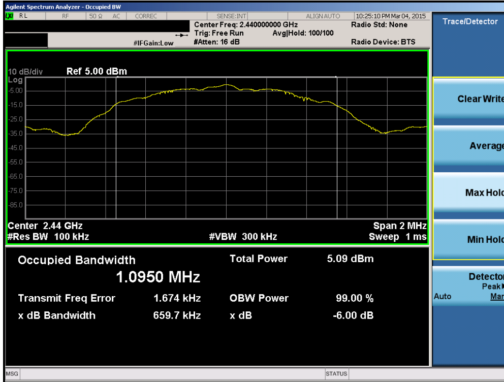
Plot 6-2. 6dB Bandwidth Plot (Bluetooth (LE) – Ch. 19)
