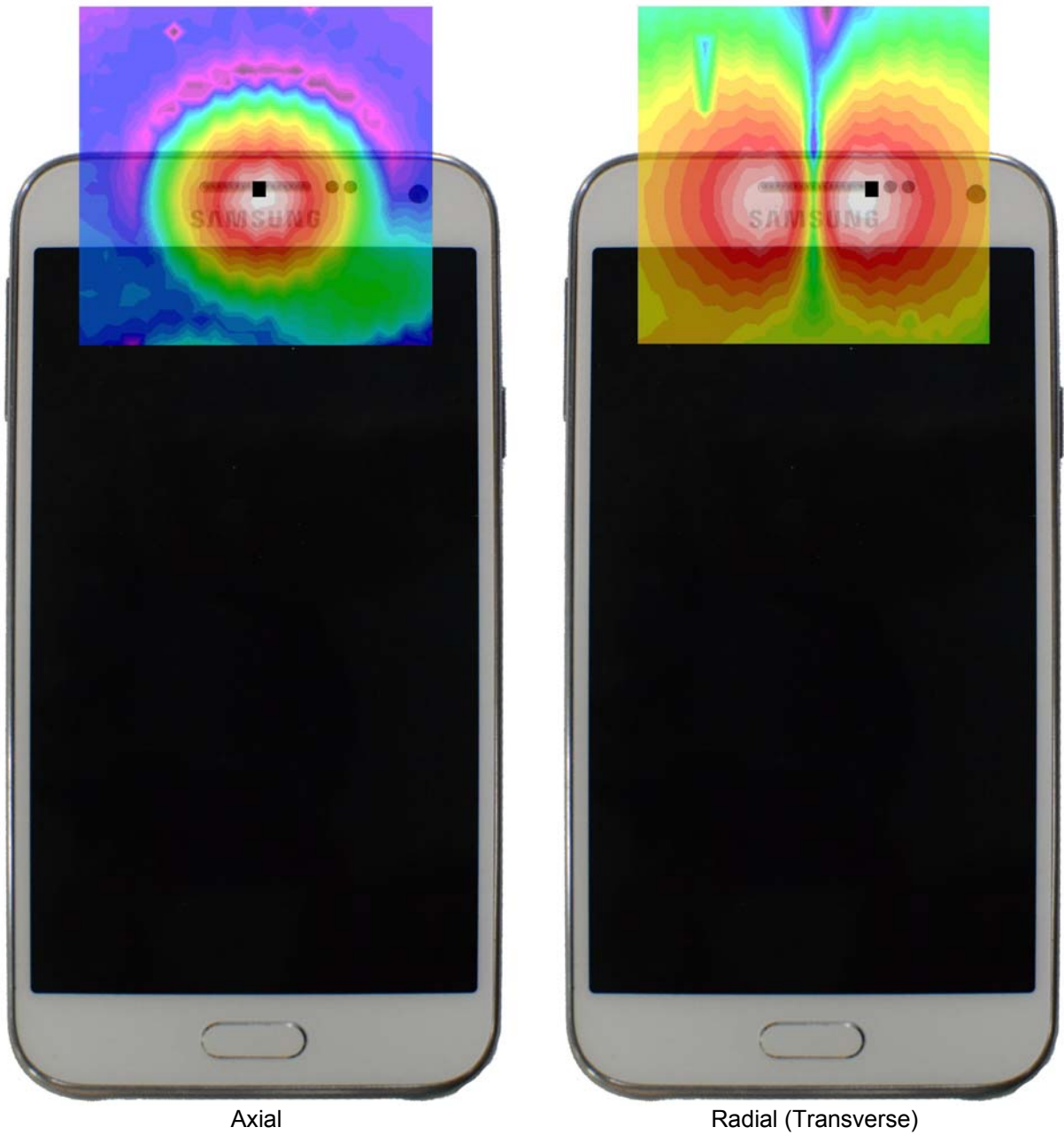
Figure 12-3 T-Coil Scan Overlay Magnetic Field Distributions
