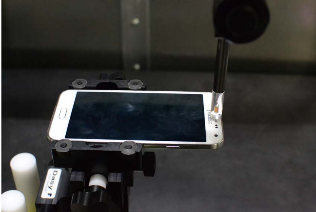
Figure 12-1 Test Setup for Wireless Device
