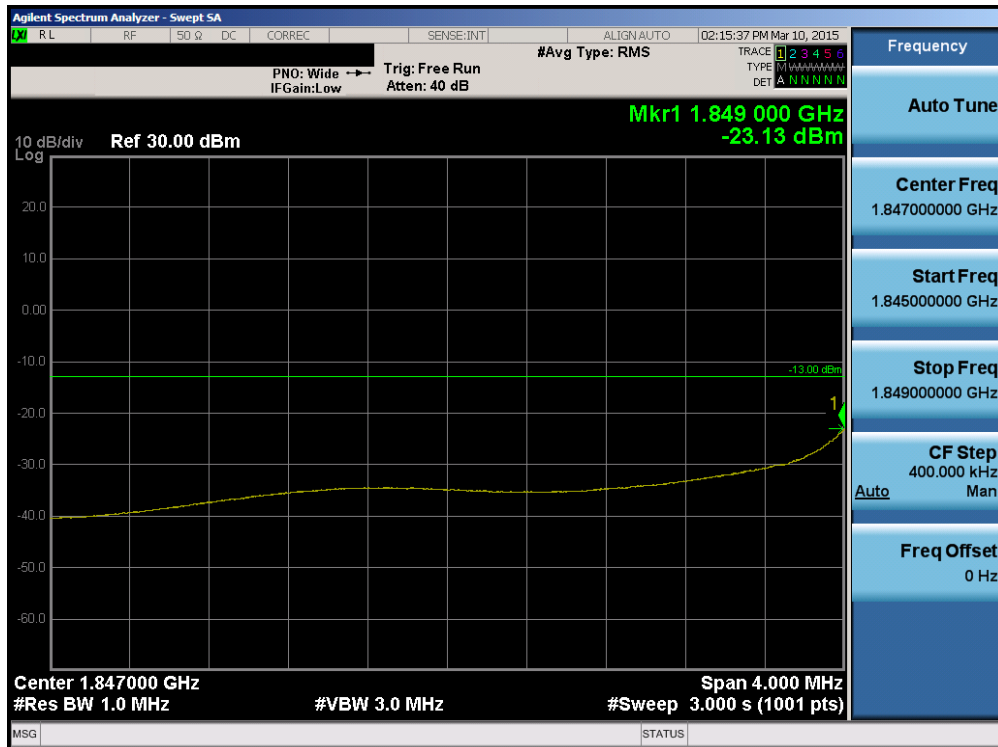
Plot 6-26. 4MHz Span Plot (PCS CDMA Mode – Ch. 25)
