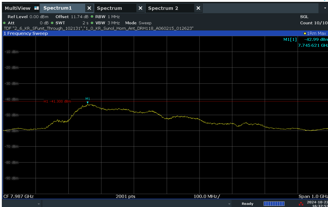
Plot 7-35. UWB Average Power Measurement - CH.9 – BPRF
