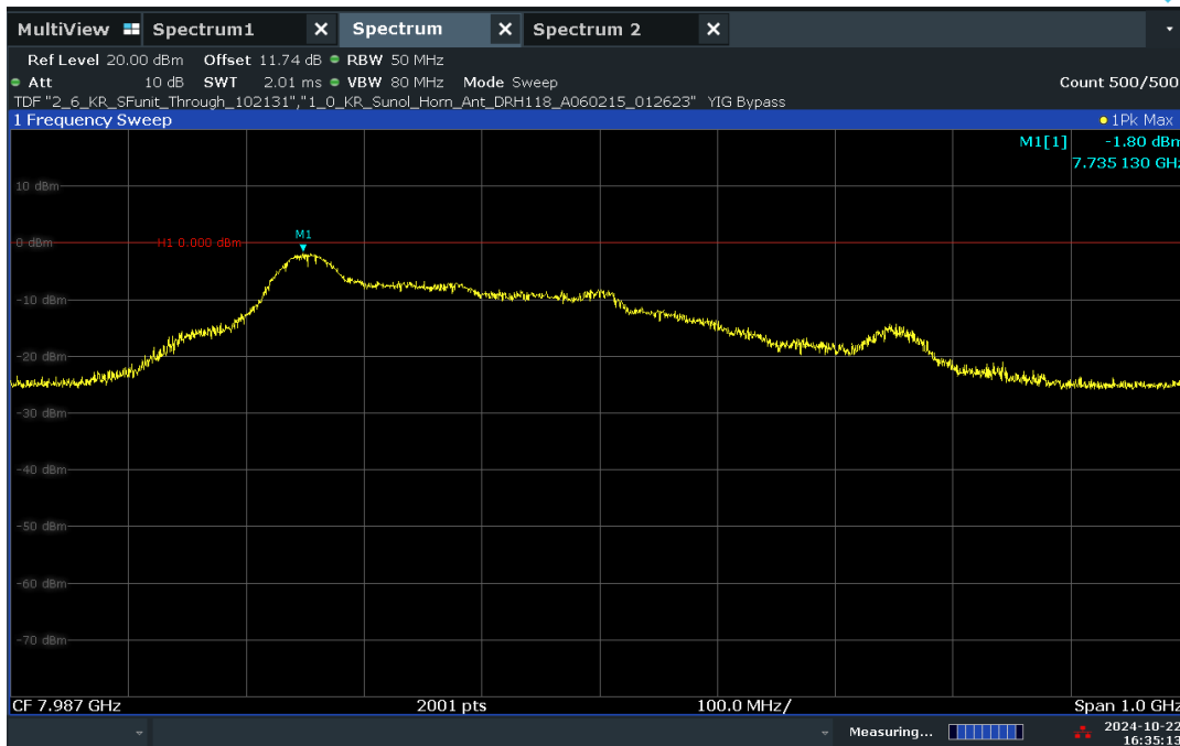
Plot 7-33. UWB Peak Power Measurement - CH.9 – BPRF
