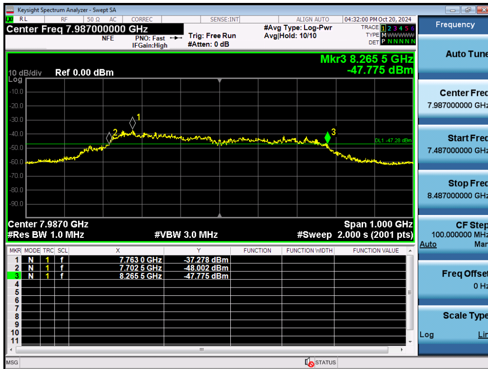
Plot 7-23. 10dBc Bandwidth - CH.9 - SP1 - Preamble 11
