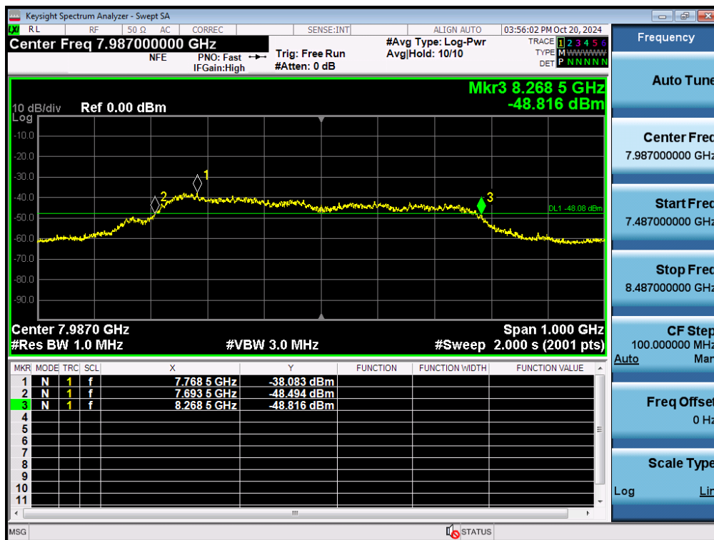
Plot 7-18. 10dBc Bandwidth – CH.9 – SP3 – Preamble 9
