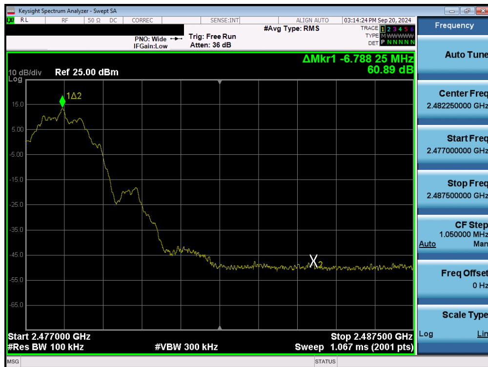
Plot 7-134. Band Edge Plot (Bluetooth (LE), 2Mbps – Ch. 36) – Dual Ant 2
