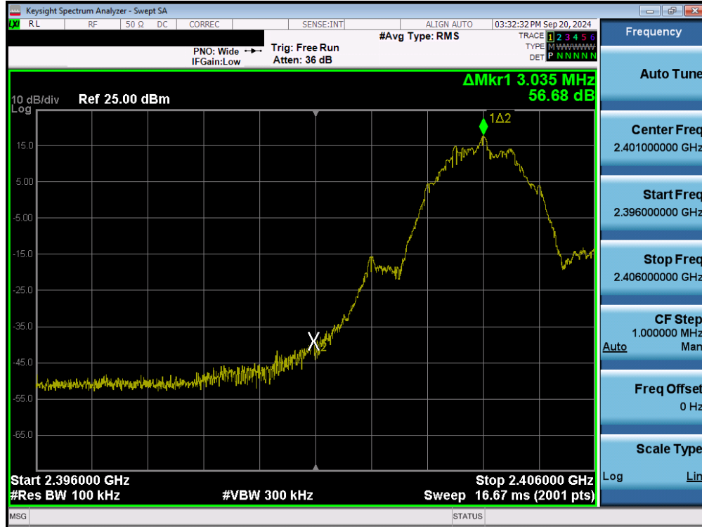
Plot 7-117. Band Edge Plot (Bluetooth (LE), 2Mbps – Ch. 0) – Ant 1
