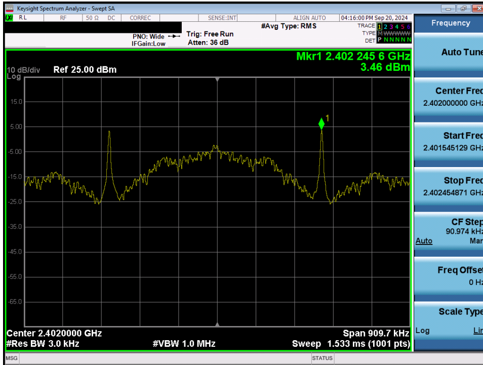
Plot 7-87. Power Spectral Density Plot (Bluetooth (LE), 125kbps – Ch. 37) – Ant 2
