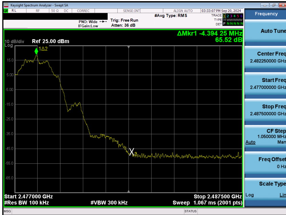
Plot 7-118. Band Edge Plot (Bluetooth (LE), 2Mbps – Ch. 36) – Ant 1
