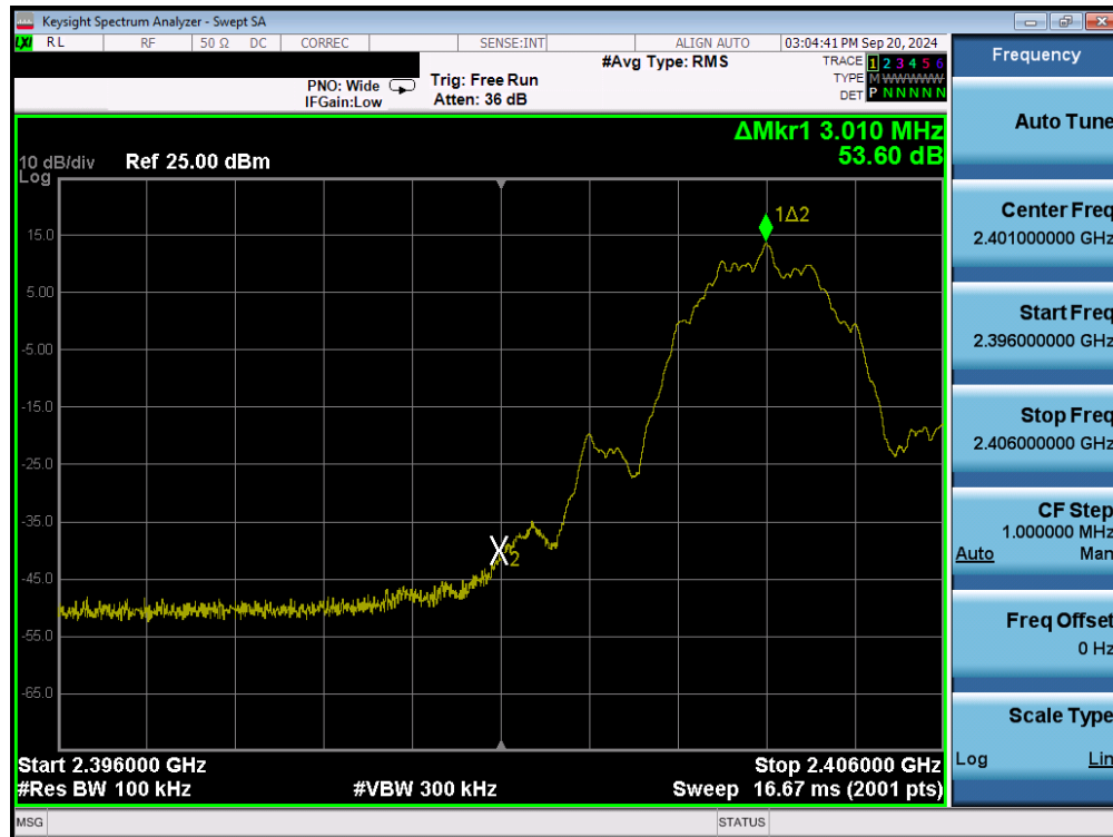
Plot 7-133. Band Edge Plot (Bluetooth (LE), 2Mbps – Ch. 0) – Dual Ant 2
