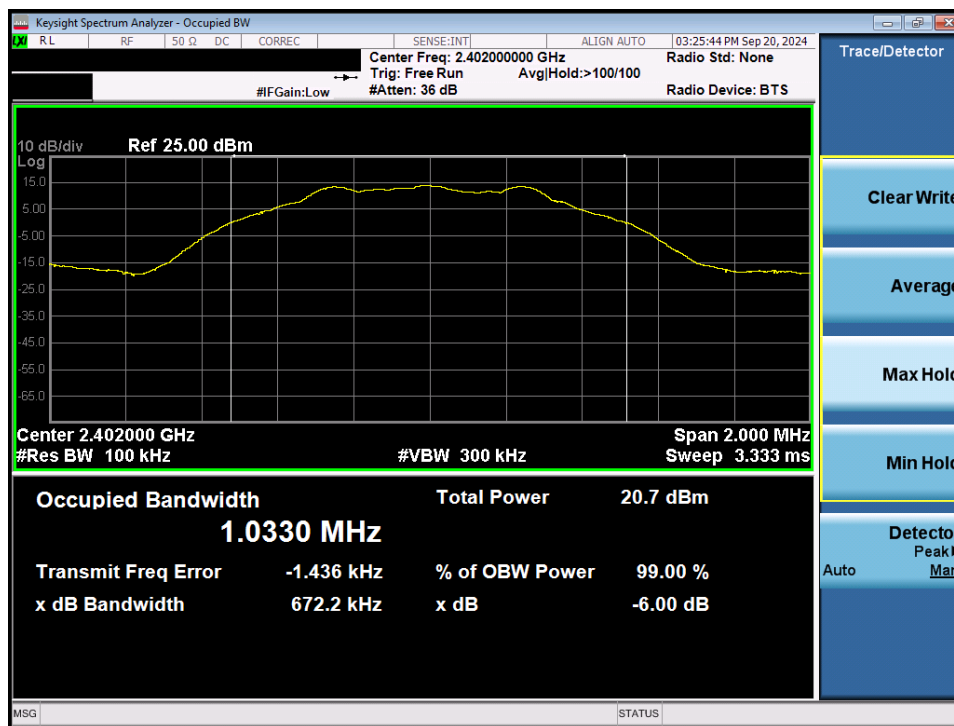
Plot 7-27. 6dB Bandwidth Plot (Bluetooth (LE), 1Mbps – Ch. 37) – Dual Ant 1
