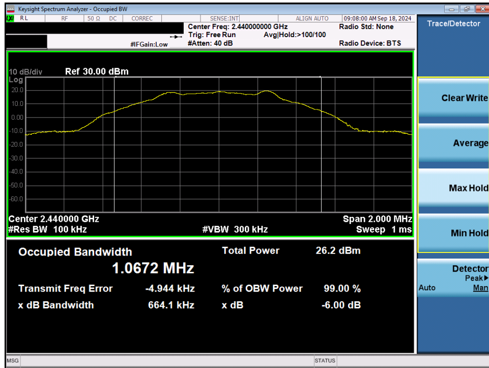
Plot 7-10. 6dB Bandwidth Plot (Bluetooth (LE), 1Mbps – Ch. 17) – Ant 1
