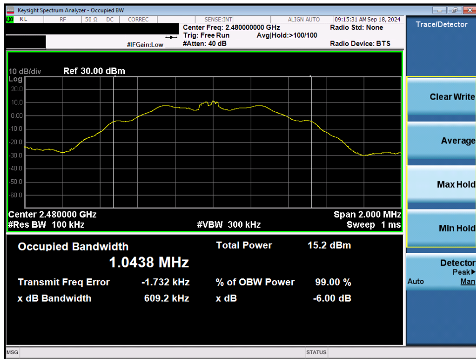
Plot 7-5. 6dB Bandwidth Plot (Bluetooth (LE), 125kbps – Ch. 39) – Ant 1
