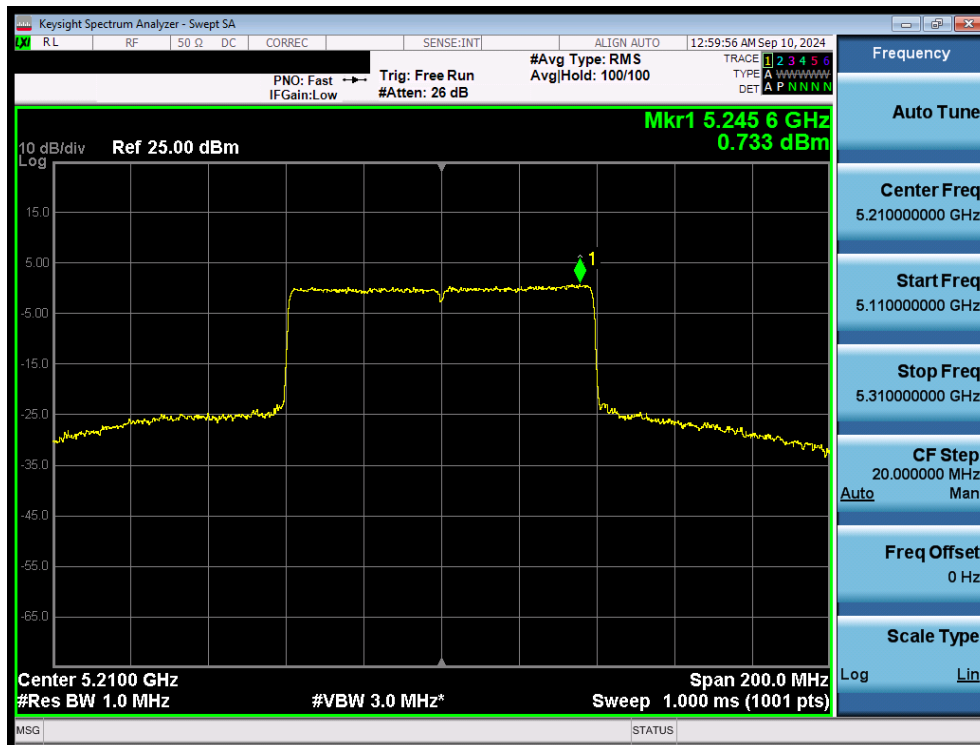
Plot 7-68. Power Spectral Density Plot MIMO ANT2 (80MHz 802.11ax/be (Full Tones) (UNII Band 1) – Ch. 42)
