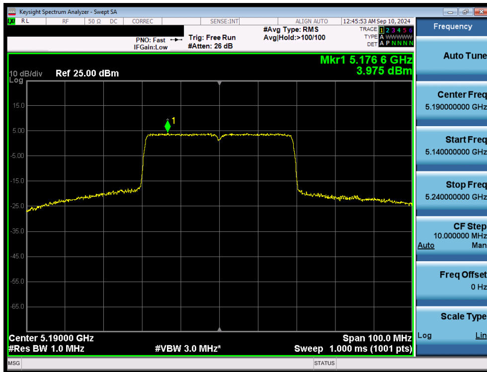
Plot 7-67. Power Spectral Density Plot MIMO ANT2 (40MHz 802.11ax/be (Full Tones) (UNII Band 1) – Ch. 38)
