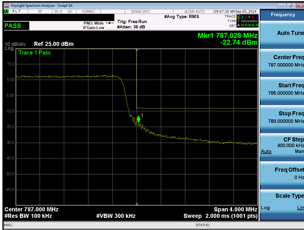
Plot 7-139. Upper Band Edge Plot (LTE Band 13 - 5MHz QPSK - Full RB - ANT1)
