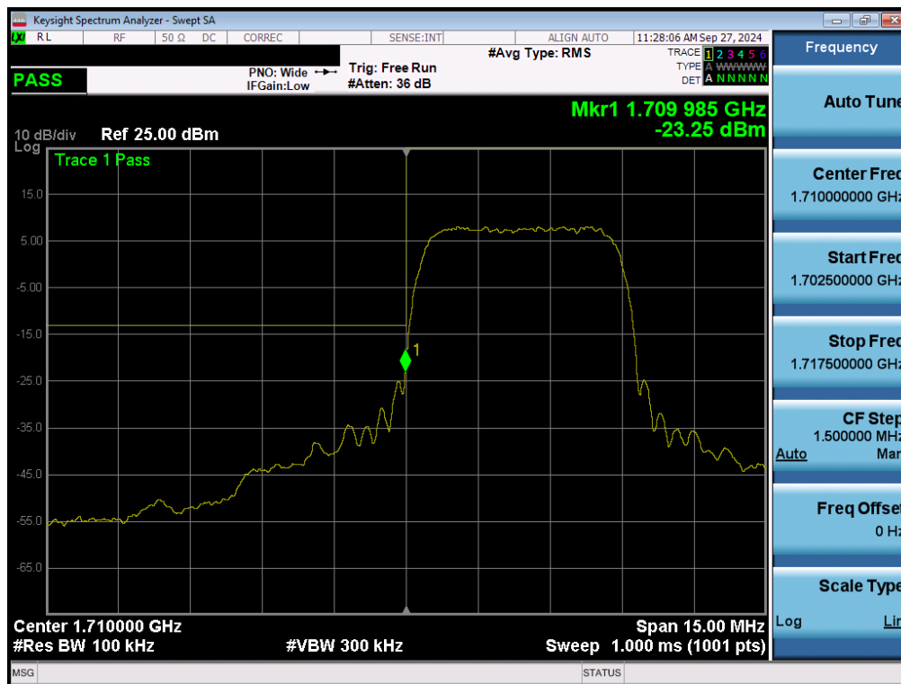
Plot 7-133. Lower Band Edge Plot (WCDMA AWS – Ch. 1312 – ANT1)
