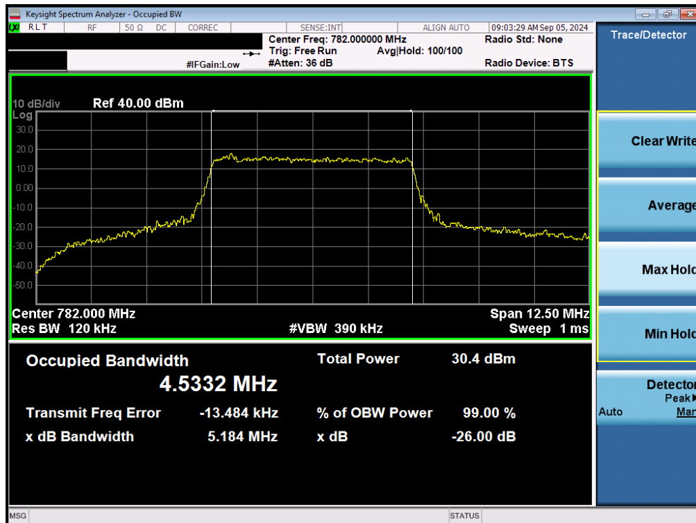
Plot 7-15. Occupied Bandwidth Plot (LTE Band 13 - 5MHz 16-QAM - Full RB – ANT1)
