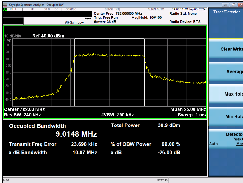
Plot 7-13. Occupied Bandwidth Plot (LTE Band 13 - 10MHz 16-QAM - Full RB – ANT1)
