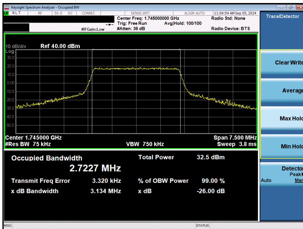
Plot 7-24. Occupied Bandwidth Plot (LTE Band 66/4 - 3MHz QPSK - Full RB - ANT1)
