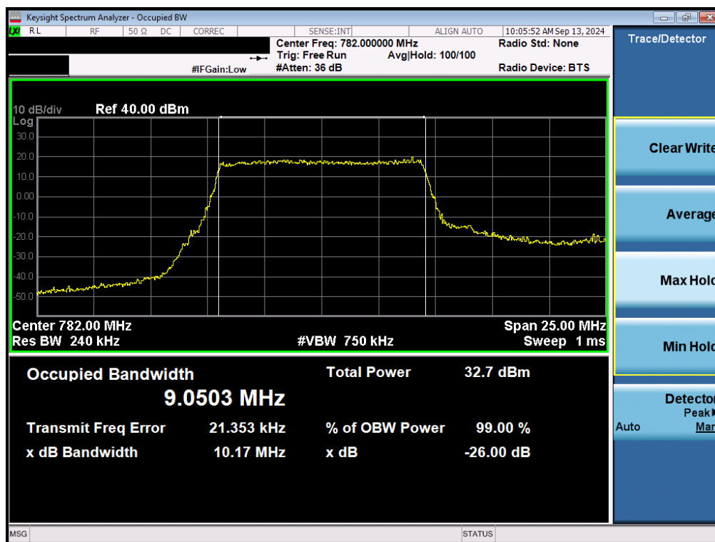
Plot 7-63. Occupied Bandwidth Plot (LTE Band 13 - 10MHz QPSK - Full RB – ANT2)
