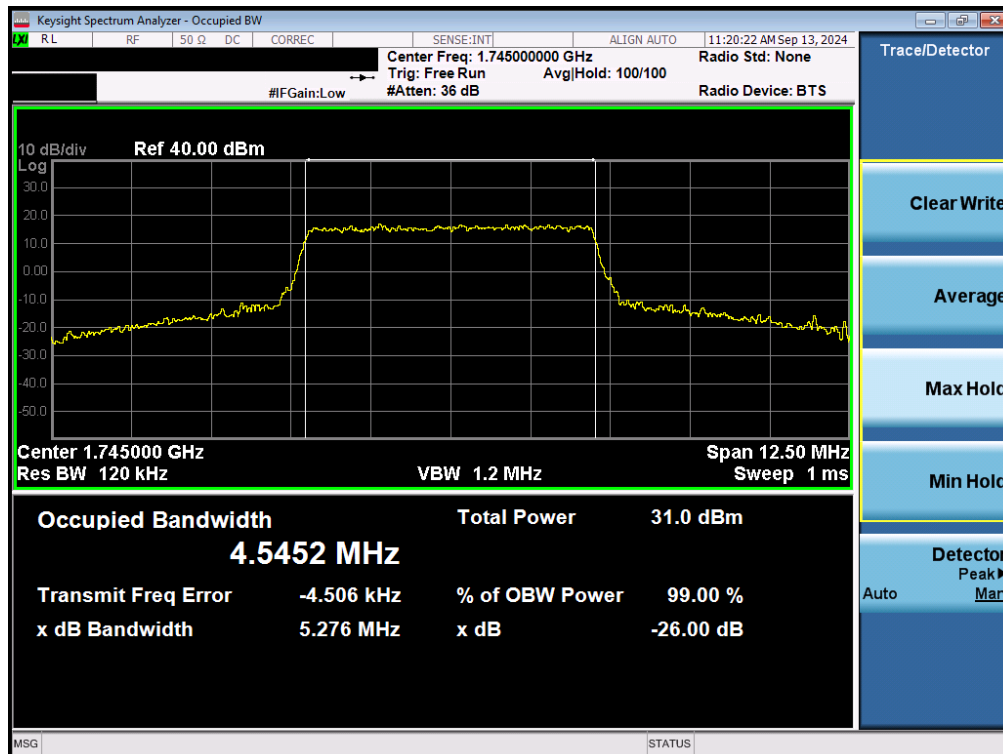
Plot 7-74. Occupied Bandwidth Plot (LTE Band 66/4 - 5MHz 16-QAM - Full RB - ANT2)
