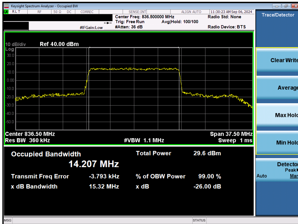
Plot 7-44. Occupied Bandwidth Plot (NR Band n26/5 - 15MHz QPSK - Full RB - Ant2)
