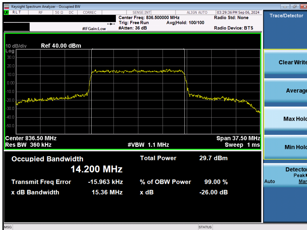
Plot 7-20. Occupied Bandwidth Plot (NR Band n26/5 - 15MHz 16-QAM - Full RB - Ant1)
