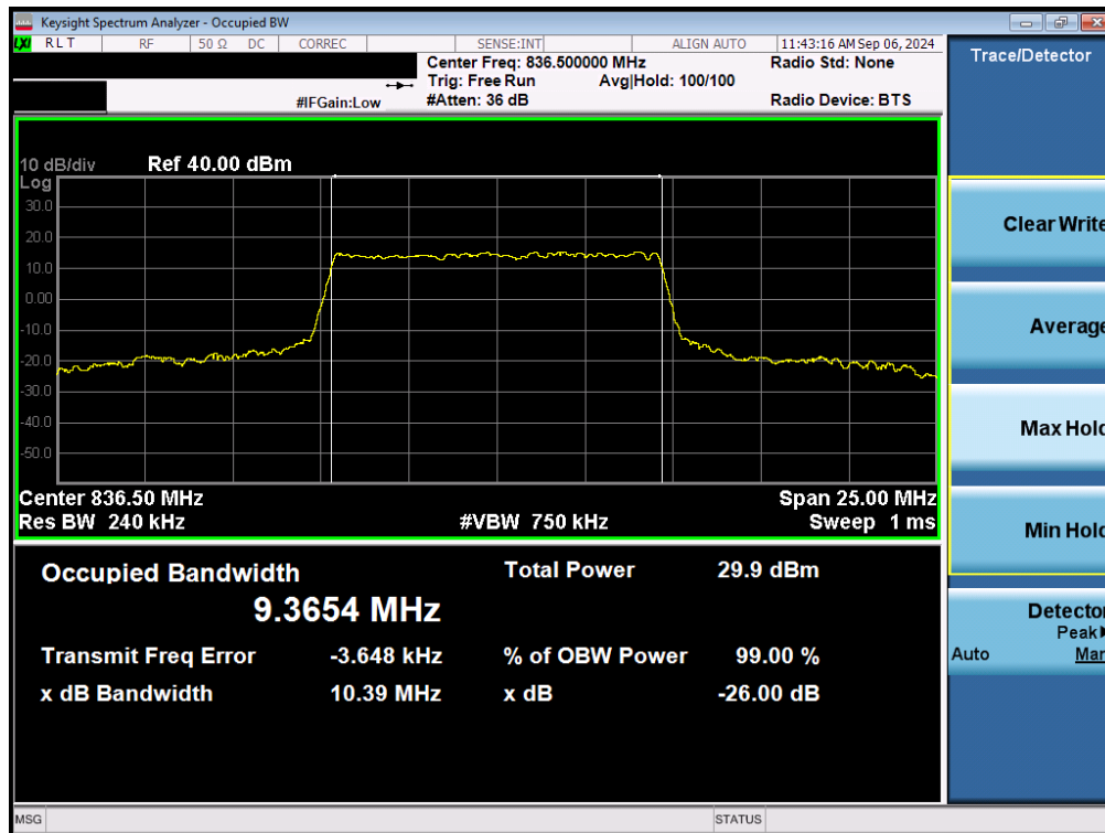
Plot 7-48. Occupied Bandwidth Plot (NR Band n26/5 - 10MHz 16-QAM - Full RB - Ant2)
