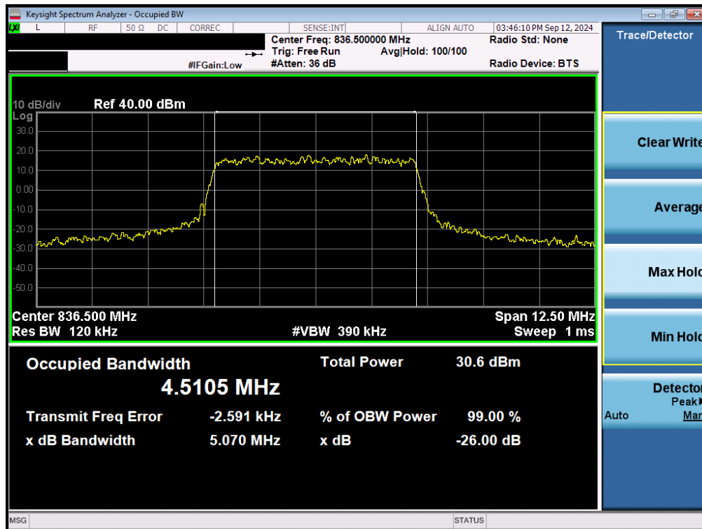
Plot 7-34. Occupied Bandwidth Plot (LTE Band 26/5 - 5MHz QPSK - Full RB - Ant2)
