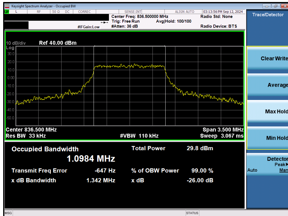
Plot 7-14. Occupied Bandwidth Plot (LTE Band 26/5 - 1.4MHz 16-QAM - Full RB - Ant1)
