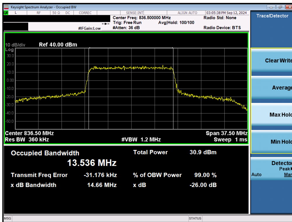
Plot 7-5. Occupied Bandwidth Plot (LTE Band 26 - 15MHz QPSK - Full RB - Ant1)
