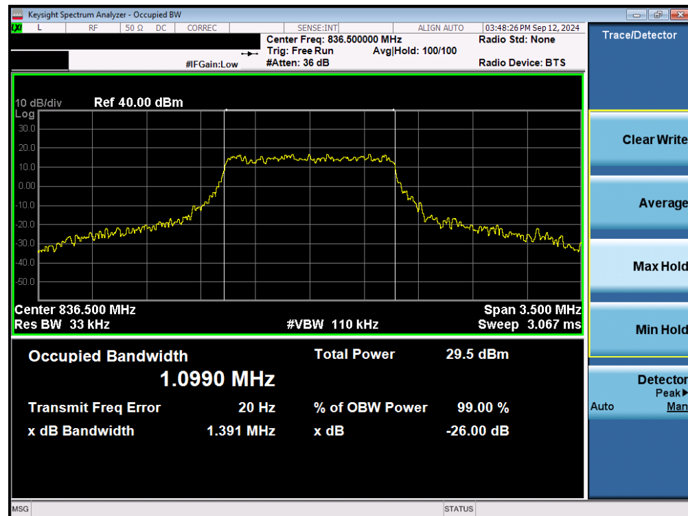
Plot 7-39. Occupied Bandwidth Plot (LTE Band 26/5 - 1.4MHz 16-QAM - Full RB - Ant2)
