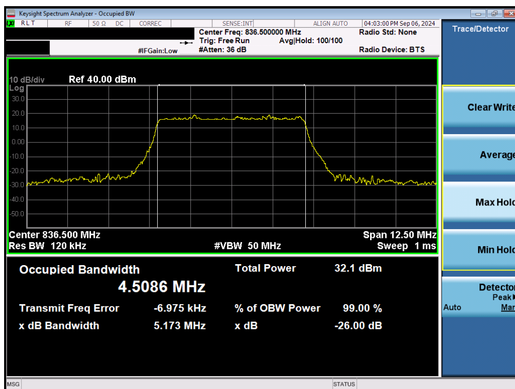
Plot 7-24. Occupied Bandwidth Plot (NR Band n26/5 - 5MHz \pi/2 BPSK - Full RB - Ant1)
