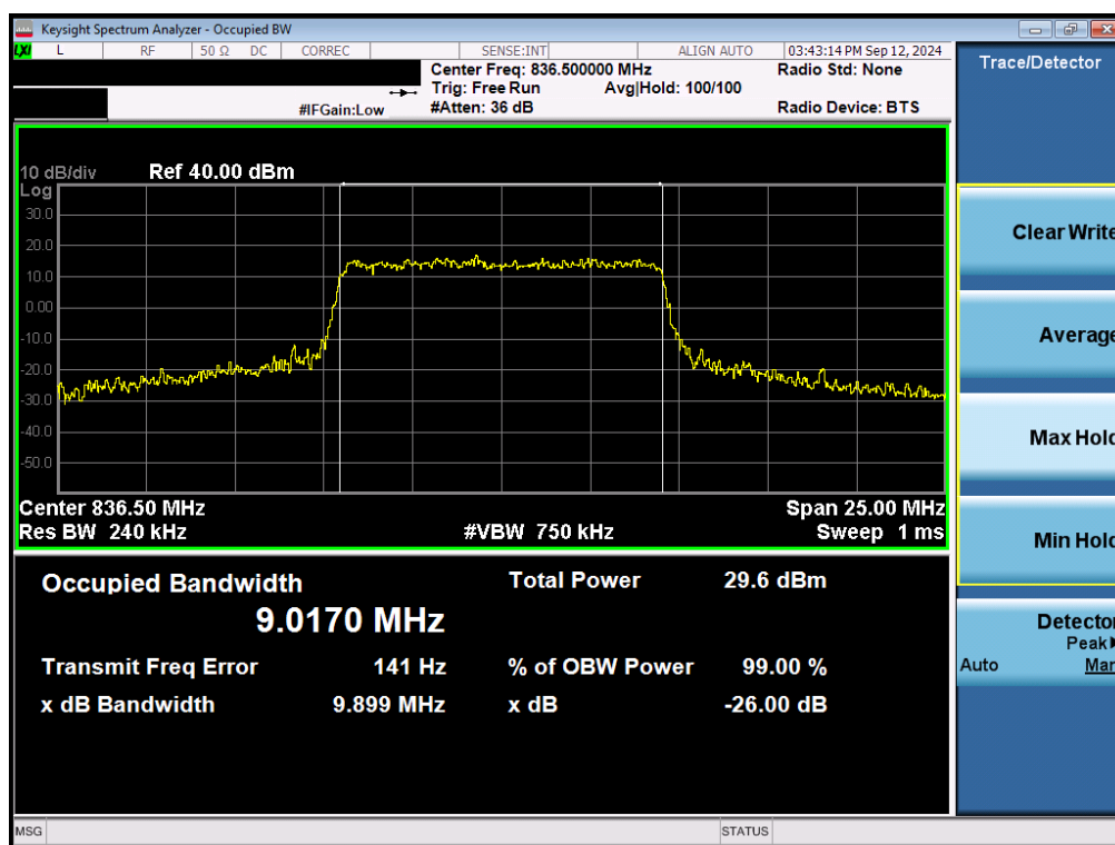
Plot 7-33. Occupied Bandwidth Plot (LTE Band 26/5 - 10MHz 16-QAM - Full RB - Ant2)
