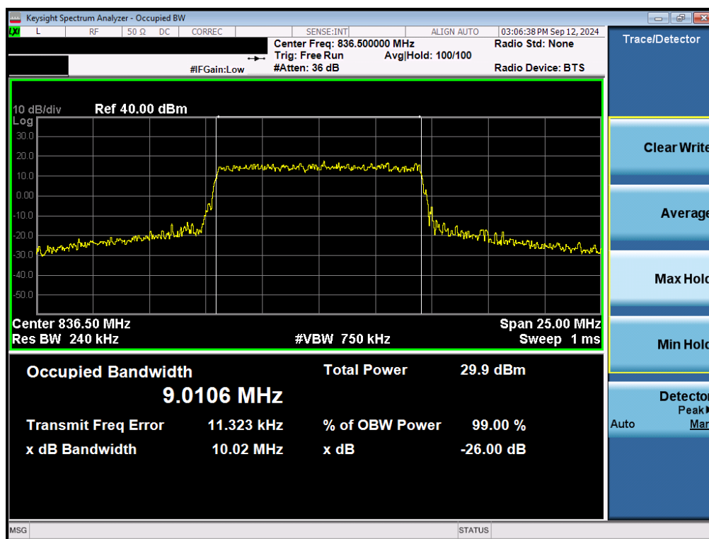
Plot 7-8. Occupied Bandwidth Plot (LTE Band 26/5 - 10MHz 16-QAM - Full RB - Ant1)
