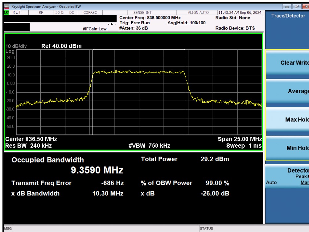
Plot 7-47. Occupied Bandwidth Plot (NR Band n26/5 - 10MHz QPSK - Full RB - Ant2)
