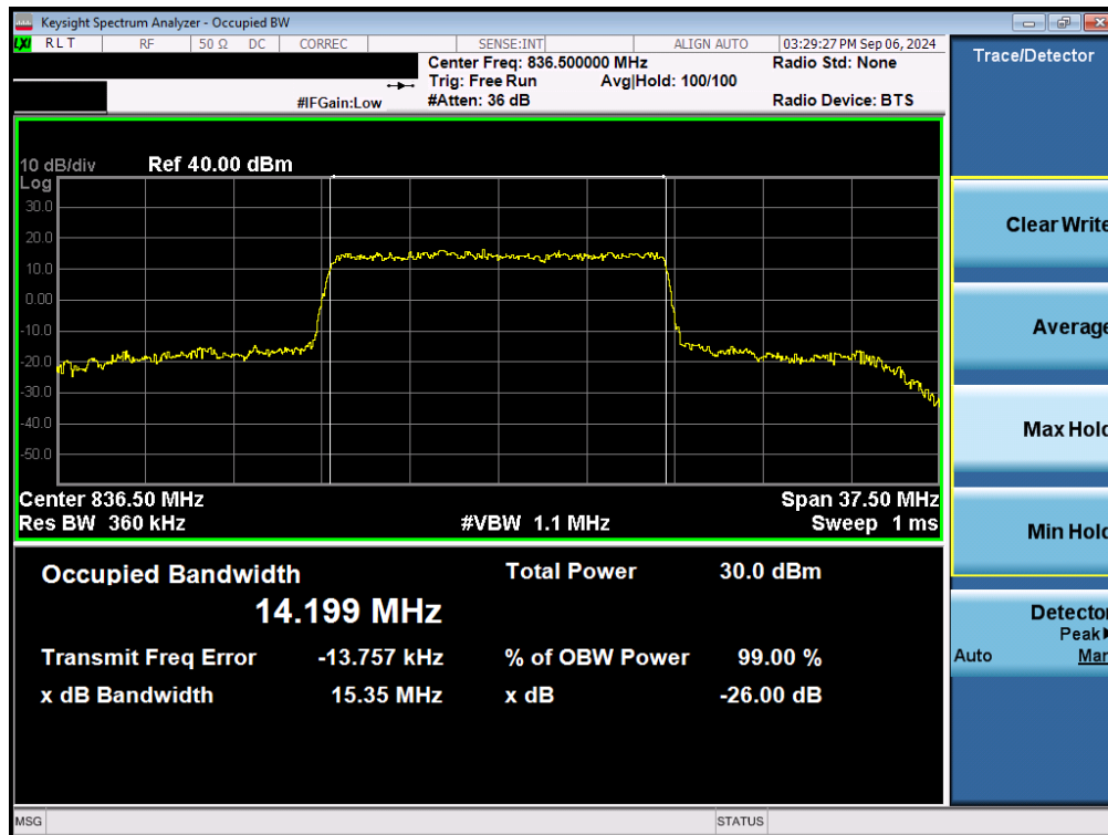
Plot 7-19. Occupied Bandwidth Plot (NR Band n26/5 - 15MHz QPSK - Full RB - Ant1)
