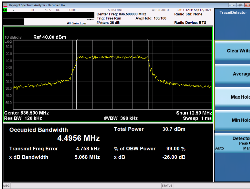
Plot 7-9. Occupied Bandwidth Plot (LTE Band 26/5 - 5MHz QPSK - Full RB - Ant1)
