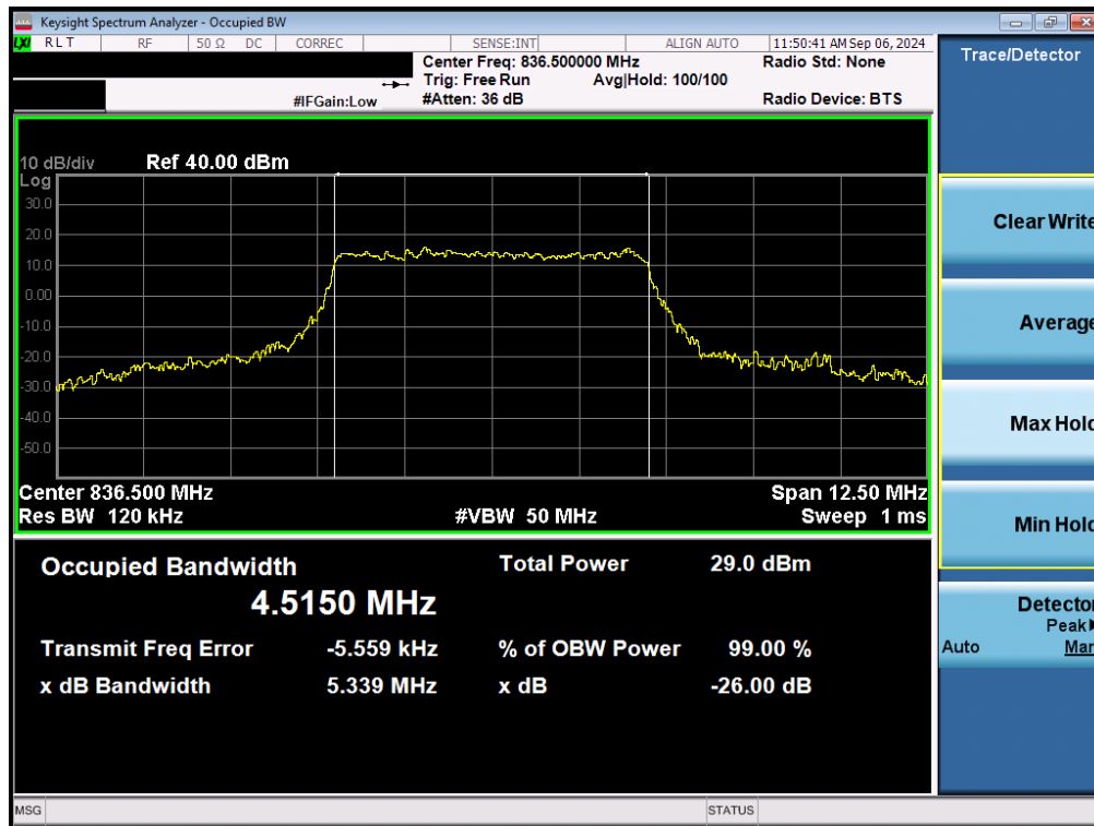
Plot 7-50. Occupied Bandwidth Plot (NR Band n26/5 - 5MHz QPSK - Full RB - Ant2)
