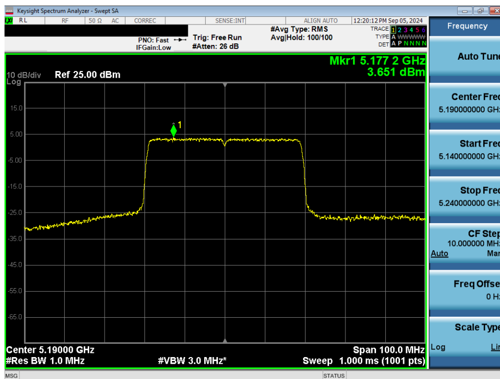
Plot 7-66. Power Spectral Density Plot MIMO ANT1 (40MHz 802.11ax/be (UNII Band 1) – Ch. 38)
