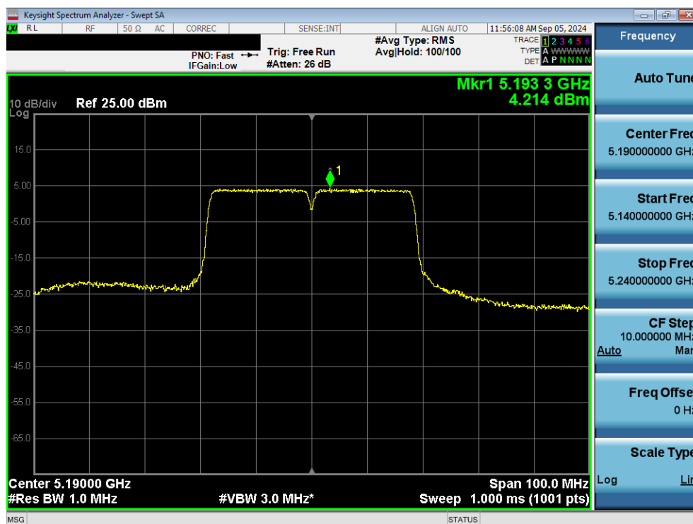
Plot 7-65. Power Spectral Density Plot MIMO ANT1 (40MHz 802.11n (UNII Band 1) – Ch. 38)
