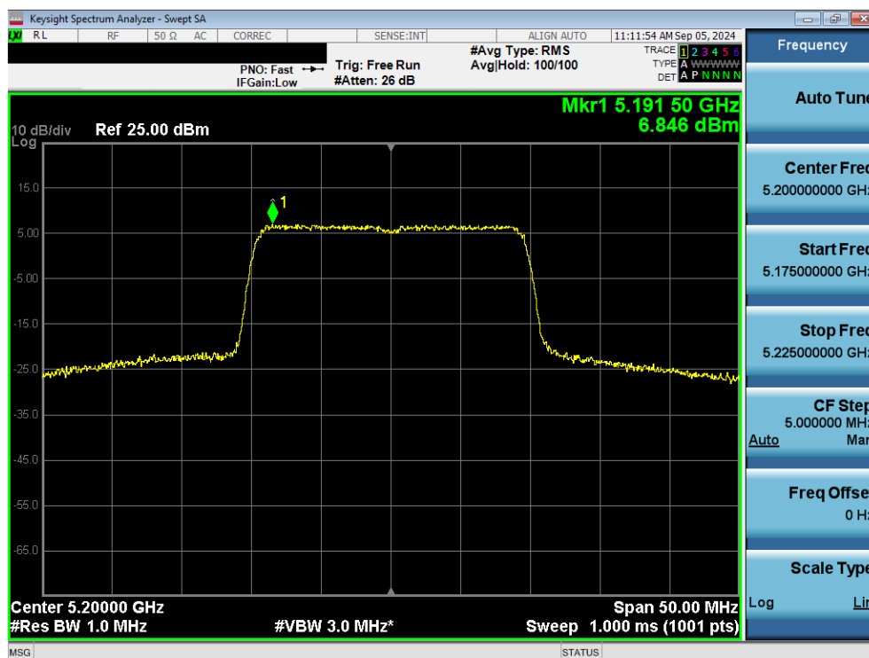
Plot 7-64. Power Spectral Density Plot MIMO ANT1 (20MHz 802.11ax/be (UNII Band 1) – Ch. 40)
