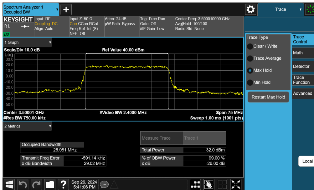
Plot 7-30. Occupied Bandwidth Plot (NR Band n77 DoD - 30MHz \pi/2 BPSK - Full RB - Ant F)
