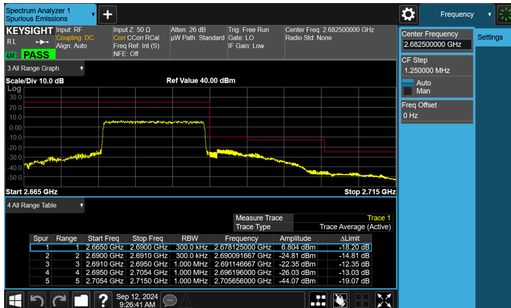
Plot 7-188. Upper ACP Plot (LTE Band 41(PC3) - 15MHz QPSK – Full RB - Ant F)
