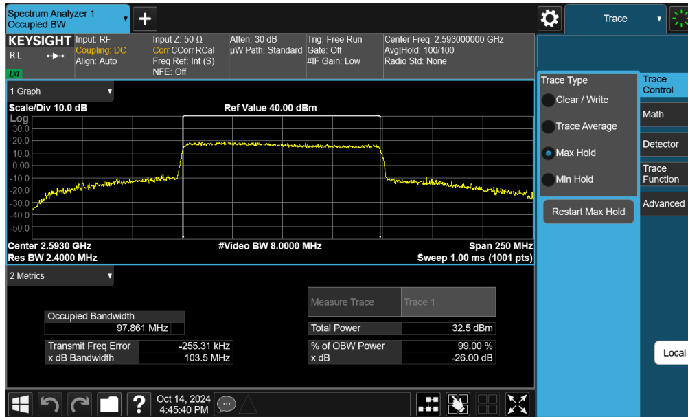
Plot 7-47. Occupied Bandwidth Plot (NR Band n41 - 100MHz 16-QAM - Full RB - Ant F)
