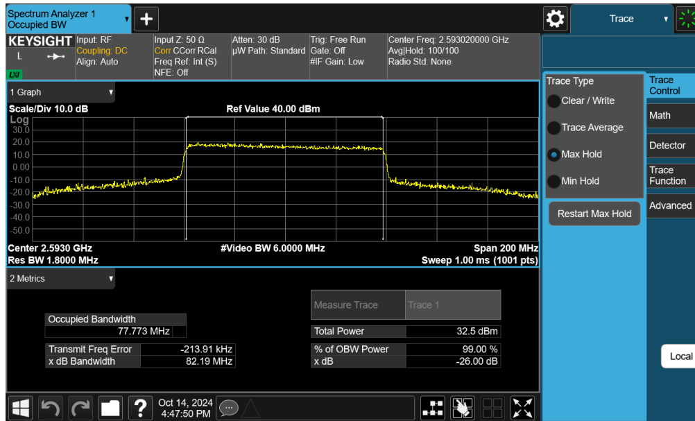
Plot 7-53. Occupied Bandwidth Plot (NR Band n41 - 80MHz 16-QAM - Full RB - Ant F)
