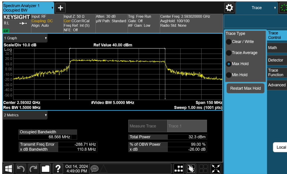
Plot 7-55. Occupied Bandwidth Plot (NR Band n41 - 70MHz QPSK - Full RB - Ant F)
