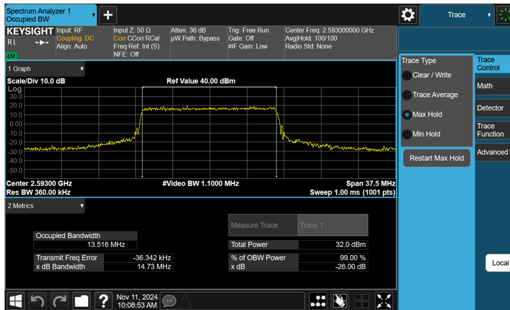
Plot 7-15. Occupied Bandwidth Plot (LTE Band 41(PC2) - 15MHz QPSK - Full RB - Ant F)
