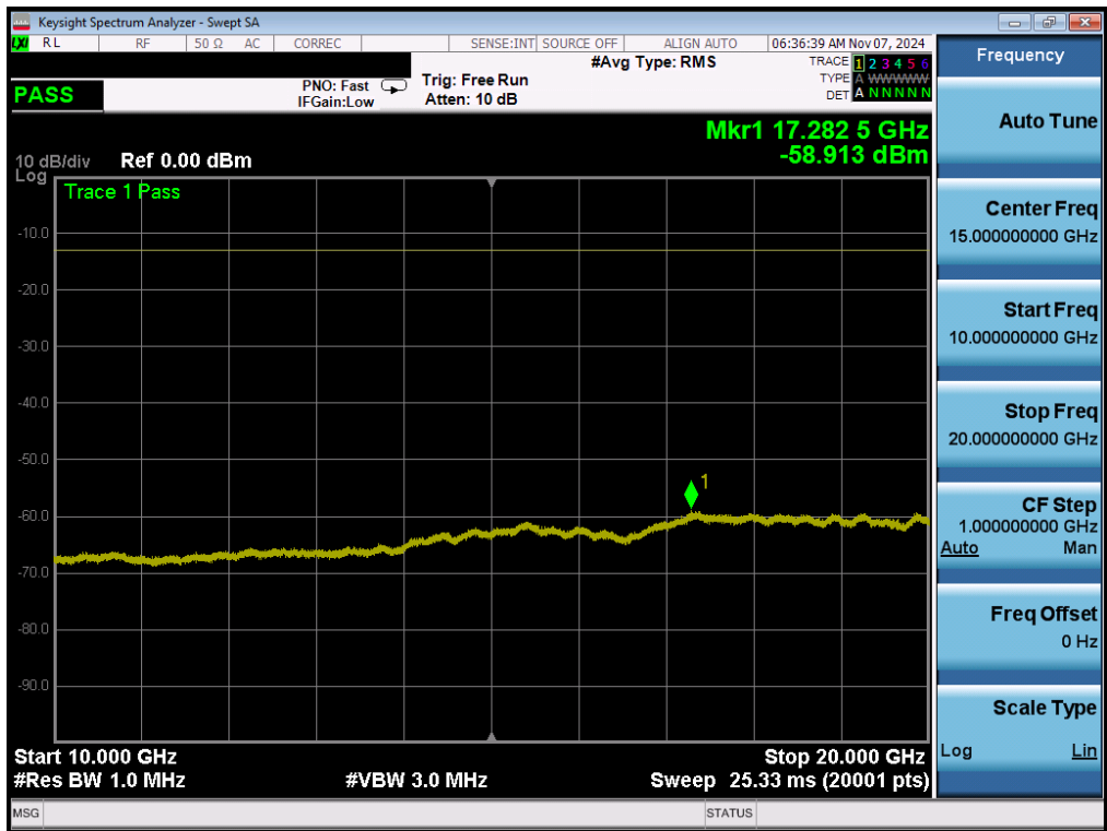
Plot 7-107. Conducted Spurious Plot (WCDMA-AWS - 5MHz QPSK - 1 RB – Low Channel)
