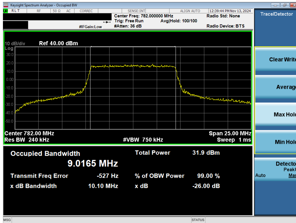
Plot 7-1. Occupied Bandwidth (Spot-check) – LTE Band 13
