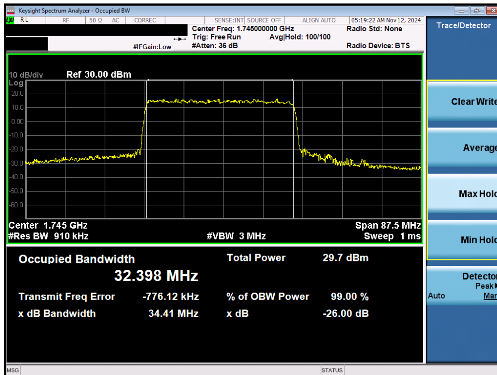
Plot 7-86. Occupied Bandwidth Plot (NR Band n66 - 35.0MHz CP-OFDM 16QAM - Full RB – ANT2)
