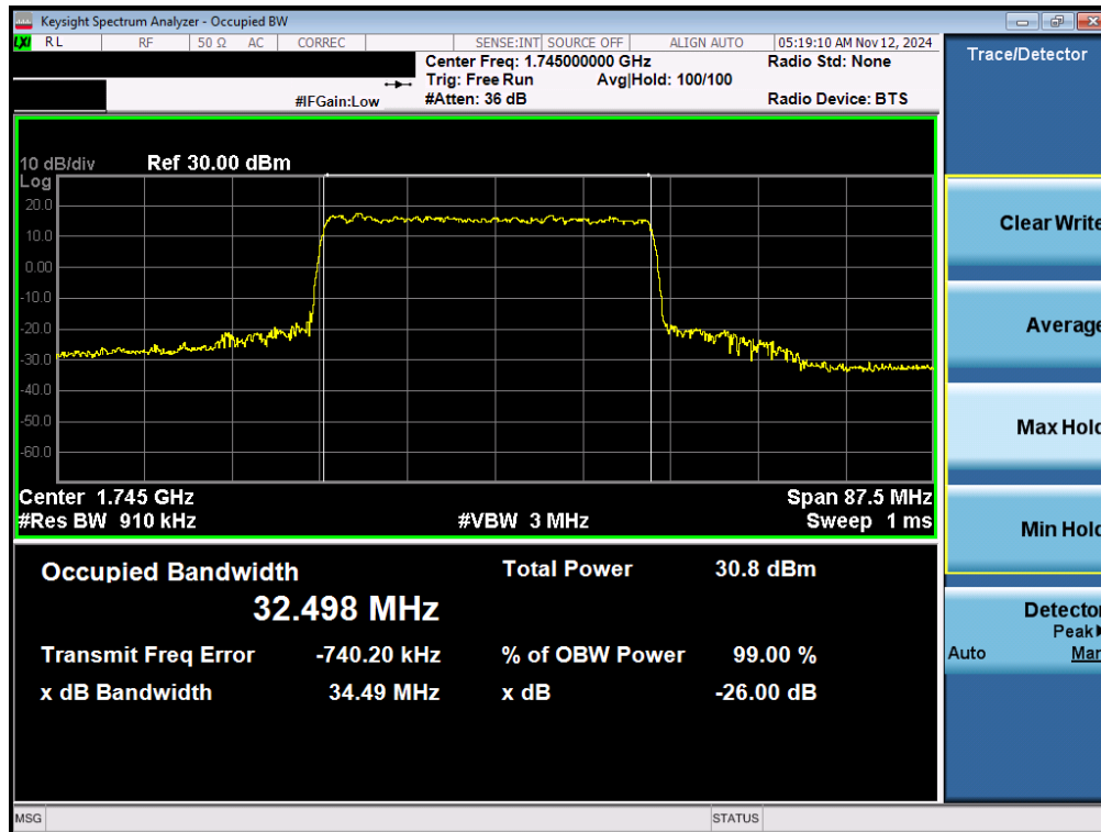
Plot 7-85. Occupied Bandwidth Plot (NR Band n66 - 35.0MHz CP-OFDM QPSK - Full RB – ANT2)
