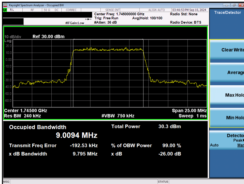
Plot 7-48. Occupied Bandwidth Plot (NR Band n66 - 10.0MHz DFT-s-OFDM BPSK - Full RB - ANT1)
