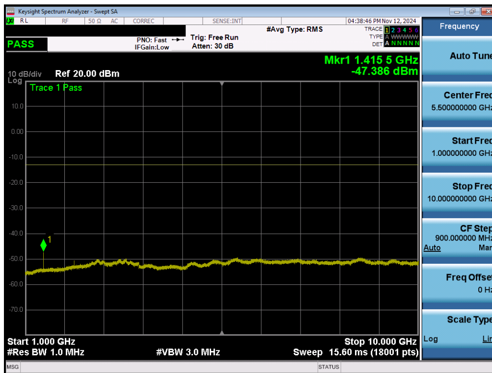
Plot 7-110. Conducted Spurious Plot (LTE Band 12/17 - 10MHz QPSK - 1 RB - Mid Channel - ANT1)
