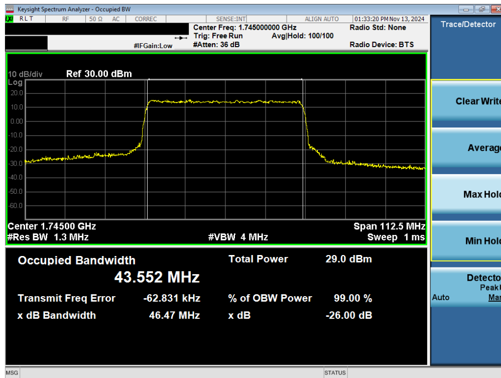
Plot 7-2. Occupied Bandwidth (Spot-check) – NR Band n66
