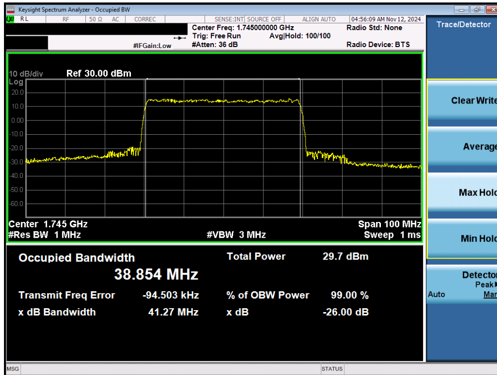
Plot 7-83. Occupied Bandwidth Plot (NR Band n66 - 40.0MHz CP-OFDM 16QAM - Full RB – ANT2)
