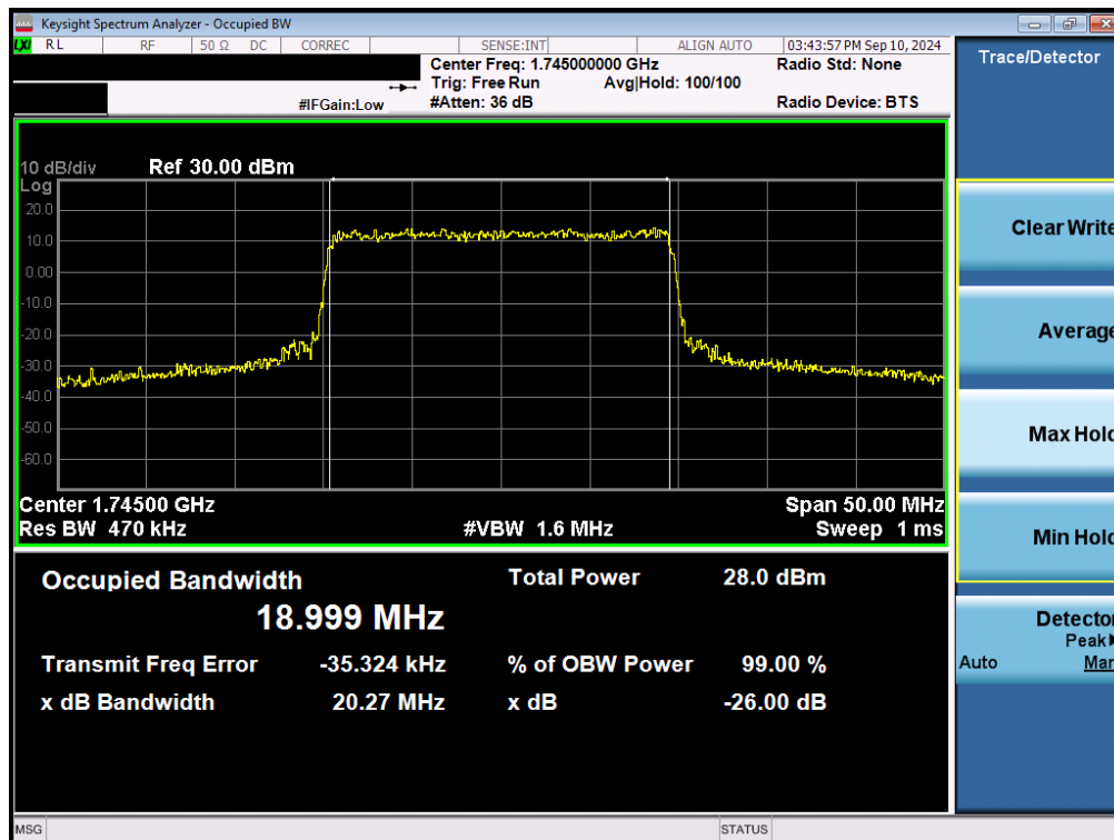
Plot 7-44. Occupied Bandwidth Plot (NR Band n66 - 20.0MHz CP-OFDM 16QAM - Full RB – ANT1)
