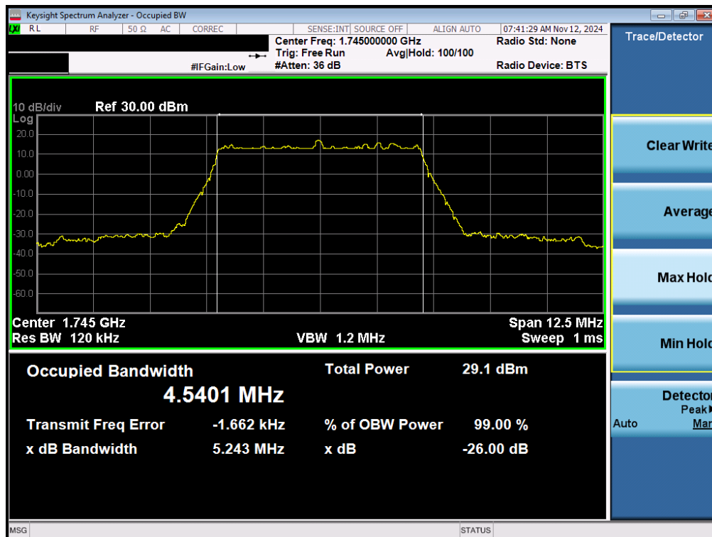
Plot 7-104. Occupied Bandwidth Plot (NR Band n66 - 5.0MHz CP-OFDM 16QAM - Full RB – ANT2)
