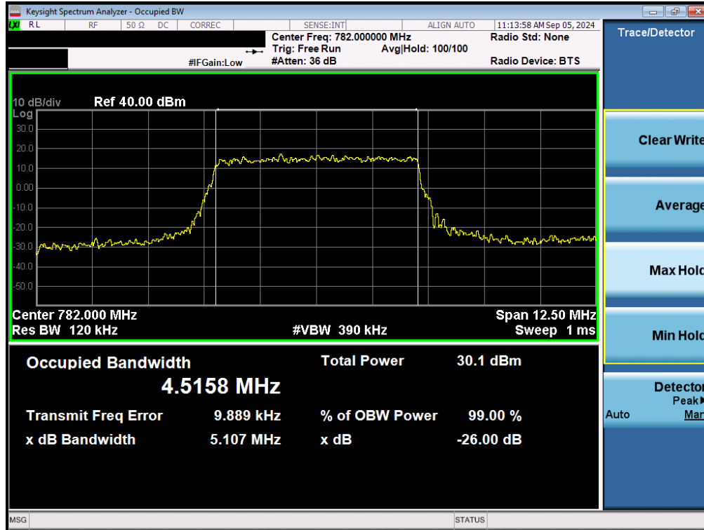
Plot 7-13. Occupied Bandwidth Plot (LTE Band 13 - 5MHz QPSK - Full RB – ANT1)
