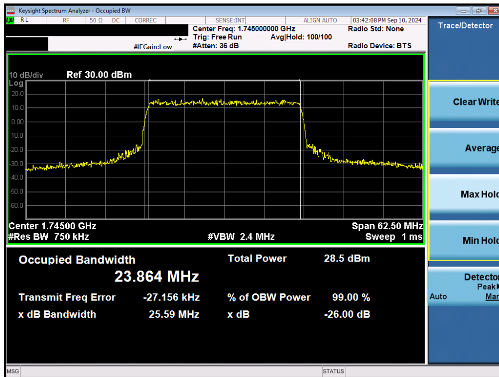
Plot 7-40. Occupied Bandwidth Plot (NR Band n66 - 25.0MHz CP-OFDM QPSK - Full RB – ANT1)
