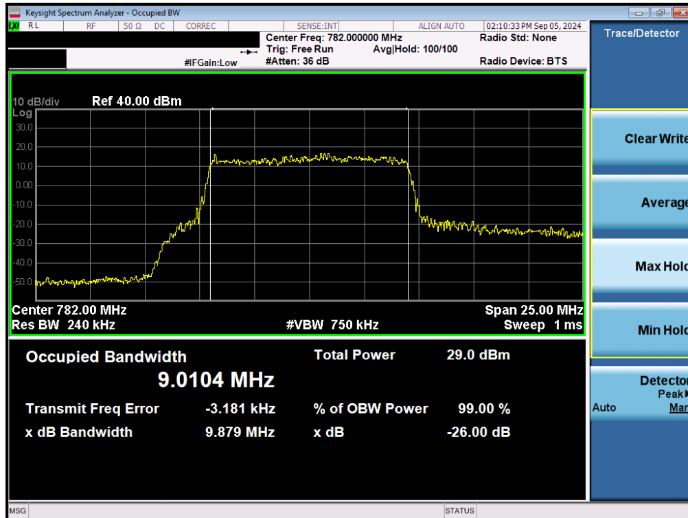
Plot 7-63. Occupied Bandwidth Plot (LTE Band 13 - 10MHz 16-QAM - Full RB – ANT2)
