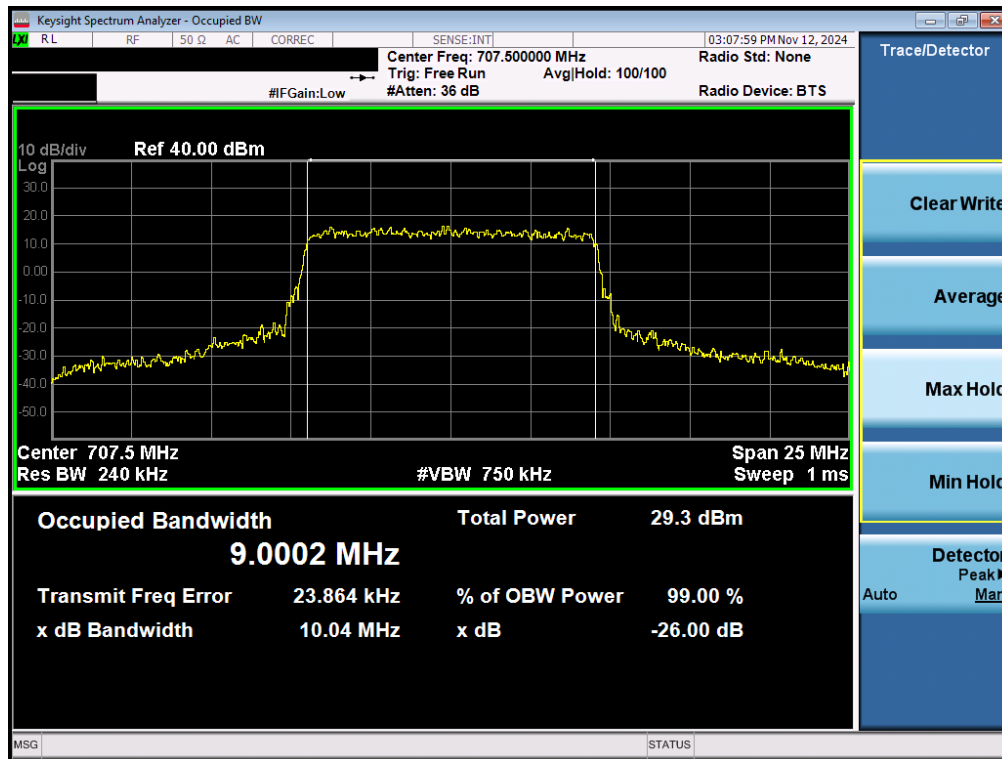
Plot 7-54. Occupied Bandwidth Plot (LTE Band 12/17 - 10MHz QPSK - Full RB – ANT2)
