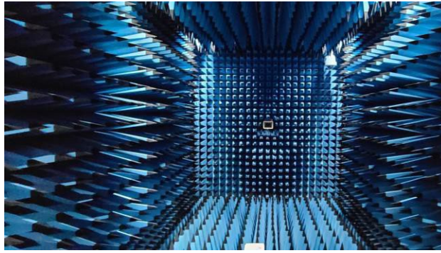
Figure 2: Geometry of Anechoic Chamber for Radiation patterns.
