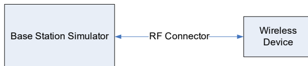
Figure 10-4 Power Measurement Setup – NR FDD
