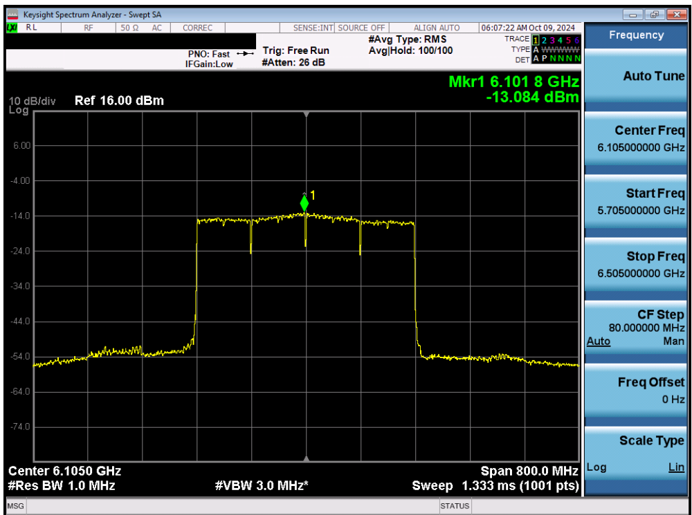
Plot 7-85. Power Spectral Density Plot MIMO ANT1 (320MHz 802.11ax/be (Full Tones) (UNII Band 5) – Ch. 31) - LPI
