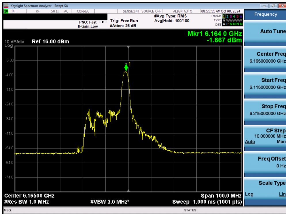
Plot 7-65. Power Spectral Density Plot MIMO ANT1 (40MHz 802.11ax/be (26 Tones) (UNII Band 5) – Ch. 43) - LPI
