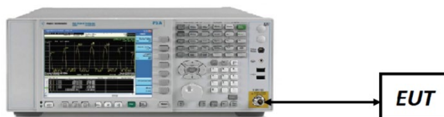
Figure 7-1. Test Instrument & Measurement Setup
