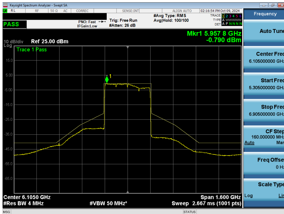
Plot 7-112. In Band Emissions Plot MIMO ANT2 (320MHz 802.11ax/be (UNII Band 5) – Ch. 31) - SP
