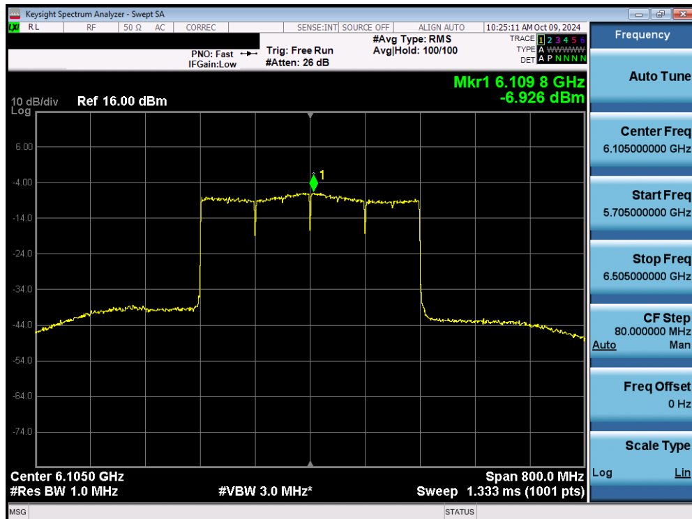
Plot 7-58. Power Spectral Density Plot MIMO ANT1 (320MHz 802.11ax/be (UNII Band 5) – Ch. 31) - SP
