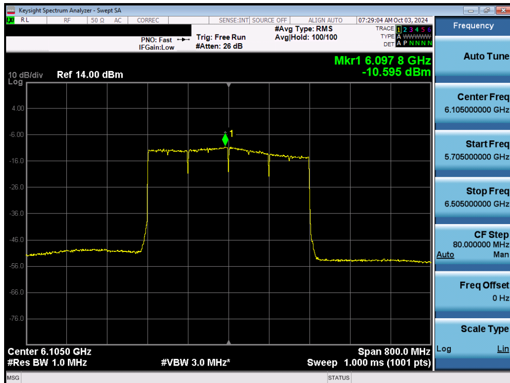
Plot 7-67. Power Spectral Density Plot MIMO ANT2 (320MHz 802.11ax/be (UNII Band 5) – Ch. 31) - LPI
