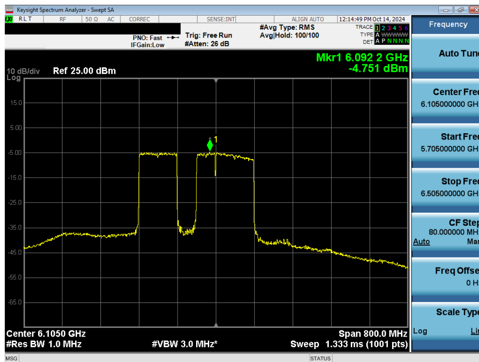
Plot 7-79. Power Spectral Density Plot MIMO ANT2 (320MHz 802.11ax/be (UNII Band 5) – Ch. 31) – 120MHz Punctured - SP
