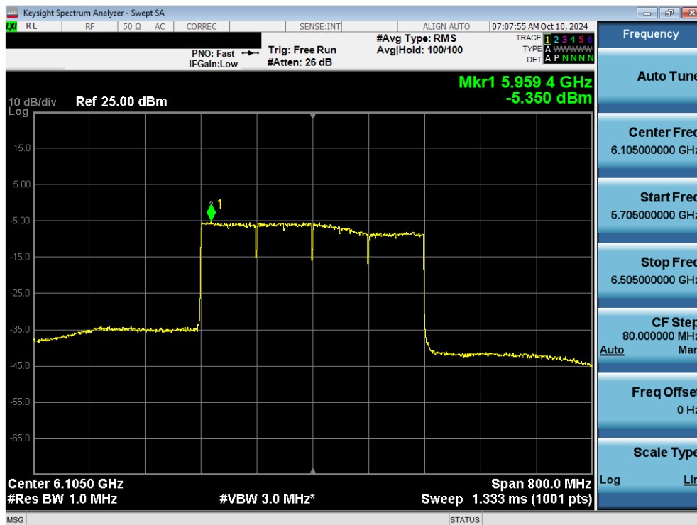
Plot 7-76. Power Spectral Density Plot MIMO ANT2 (320MHz 802.11ax/be (UNII Band 5) – Ch. 31) - SP
