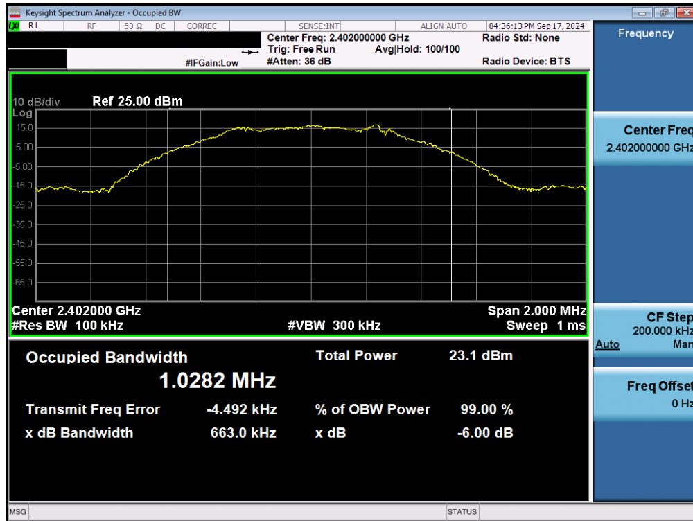
Plot 7-21. 6dB Bandwidth Plot (Bluetooth (LE), 1Mbps – Ch. 0) – Ant 2
