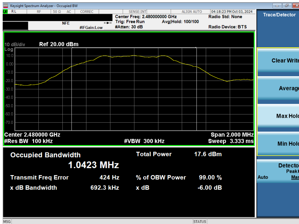
Plot 7-35. 6dB Bandwidth Plot (Bluetooth (LE), 1Mbps - Ch. 39) - Dual Ant 2
