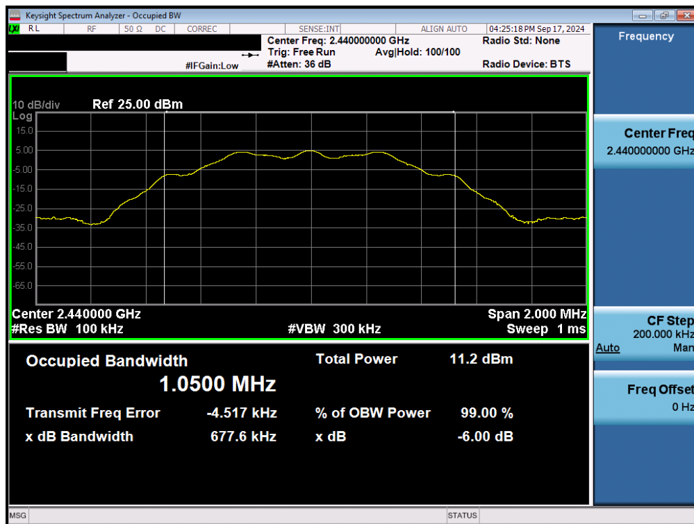
Plot 7-16. 6dB Bandwidth Plot (Bluetooth (LE), 125kbps – Ch. 19) – Ant 2
