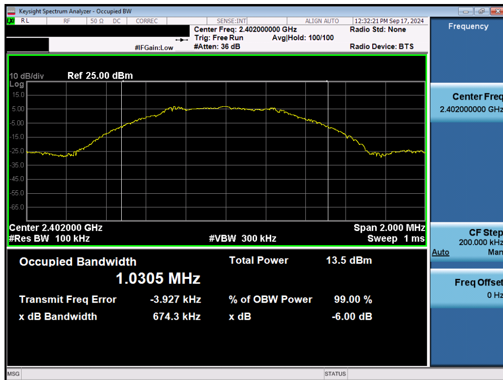
Plot 7-6. 6dB Bandwidth Plot (Bluetooth (LE), 500kbps – Ch. 0) – Ant 1
