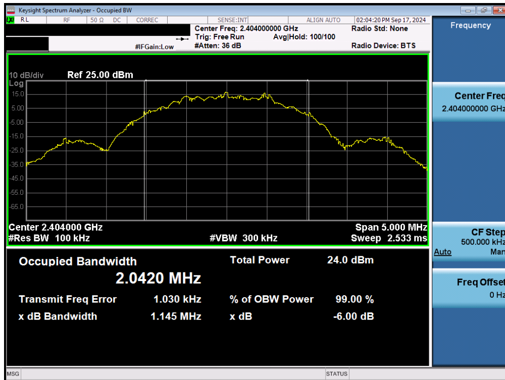
Plot 7-24. 6dB Bandwidth Plot (Bluetooth (LE), 2Mbps – Ch. 0) – Ant 2
