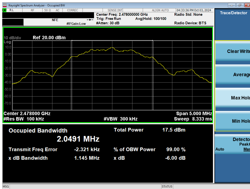
Plot 7-38. 6dB Bandwidth Plot (Bluetooth (LE), 2Mbps – Ch. 38) – Dual Ant 2
