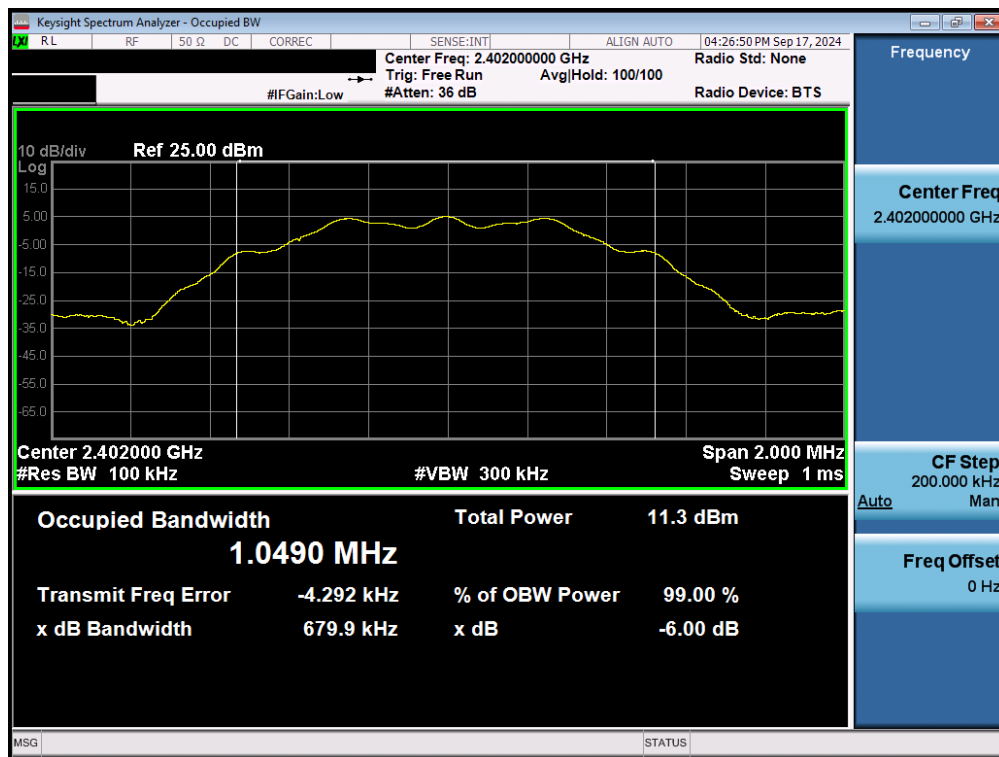
Plot 7-15. 6dB Bandwidth Plot (Bluetooth (LE), 125kbps – Ch. 0) – Ant 2
