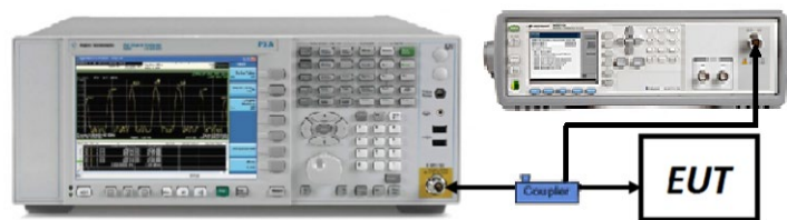
Figure 7-5. Test Instrument & Measurement Setup
