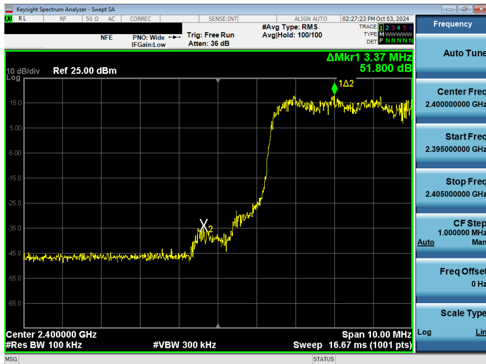
Plot 7-113. Band Edge Plot (Bluetooth with Hopping Enabled, 3 Mbps) – Ant 1
