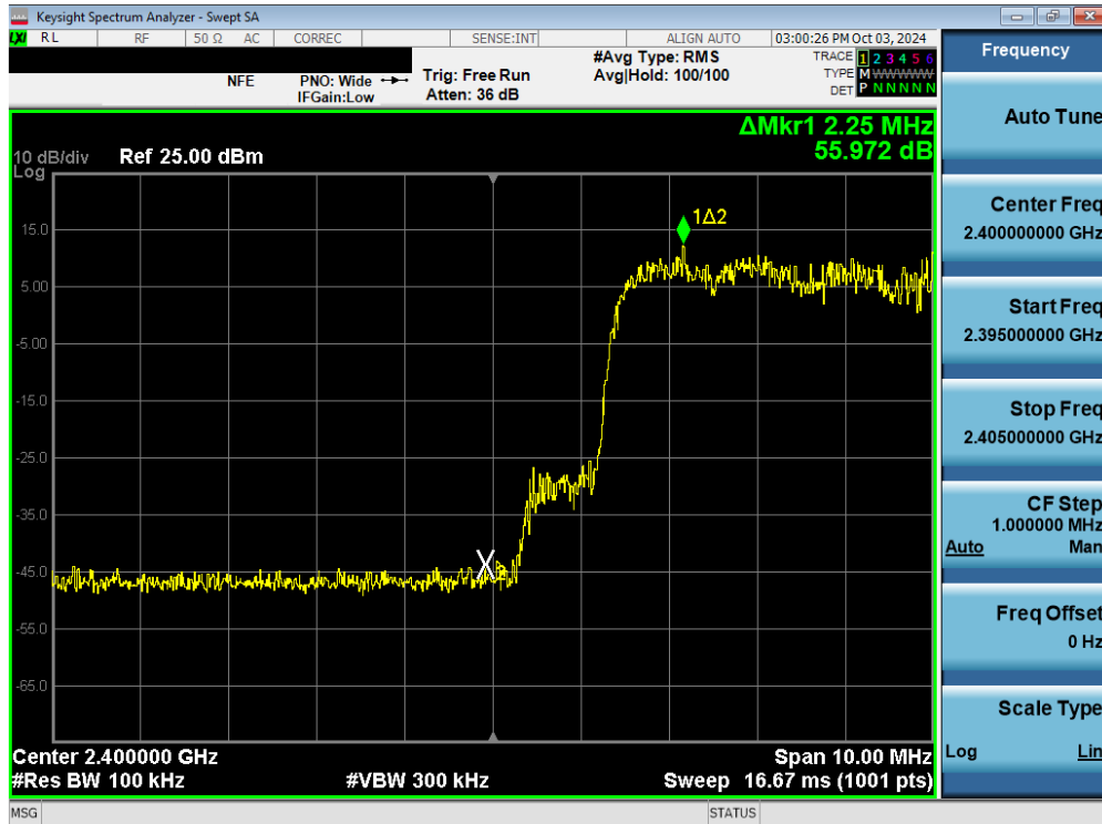
Plot 7-121. Band Edge Plot (Bluetooth with Hopping Enabled, 3 Mbps) – Dual Ant 1
