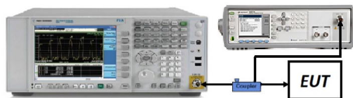
Figure 7-3. Test Instrument & Measurement Setup
