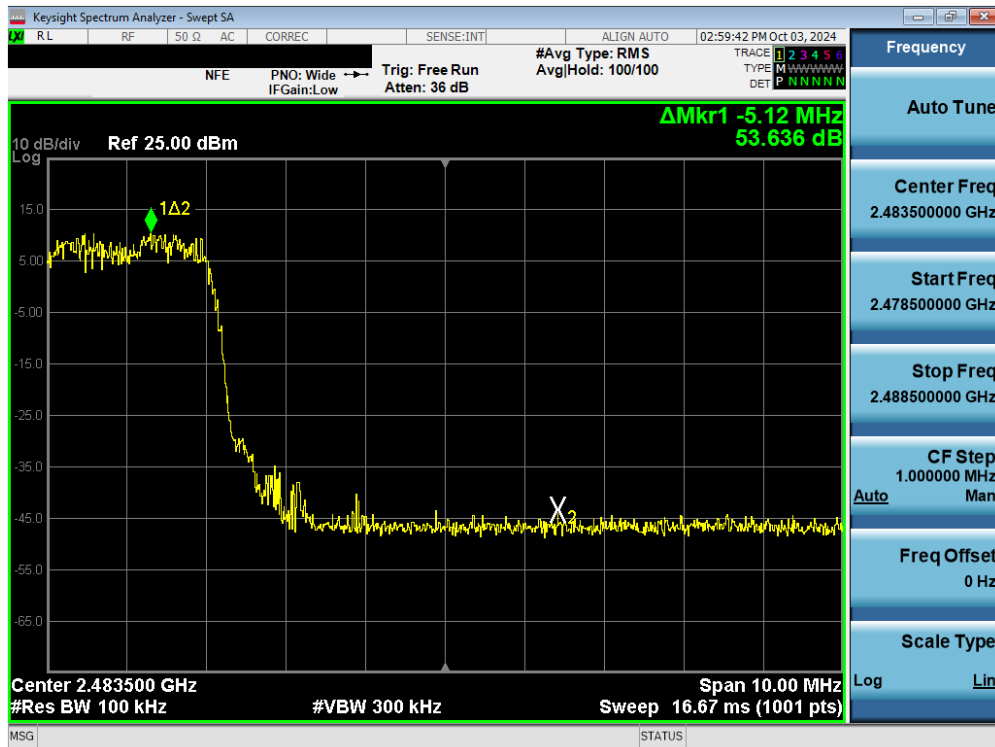
Plot 7-122. Band Edge Plot (Bluetooth with Hopping Enabled, 3 Mbps) – Dual Ant 1
