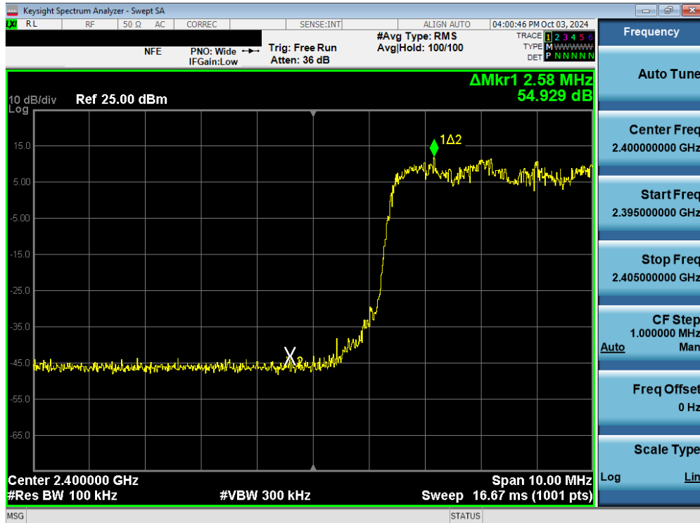
Plot 7-125. Band Edge Plot (Bluetooth with Hopping Enabled, 3 Mbps) – Dual Ant 2
