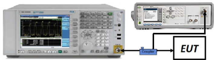
Figure 7-6. Test Instrument & Measurement Setup
