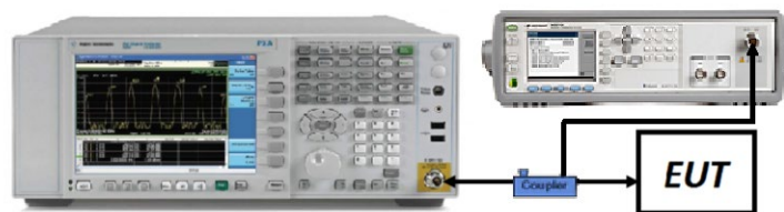
Figure 7-2. Test Instrument & Measurement Setup
