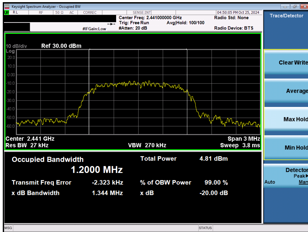
Plot 7-28. 20dB Bandwidth Plot (Bluetooth, 3Mbps – Ch. 39) – Dual Ant 1
