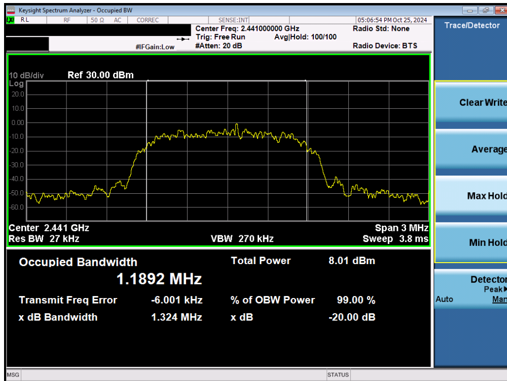
Plot 7-34. 20dB Bandwidth Plot (Bluetooth, 2Mbps – Ch. 39) – Dual Ant 2
