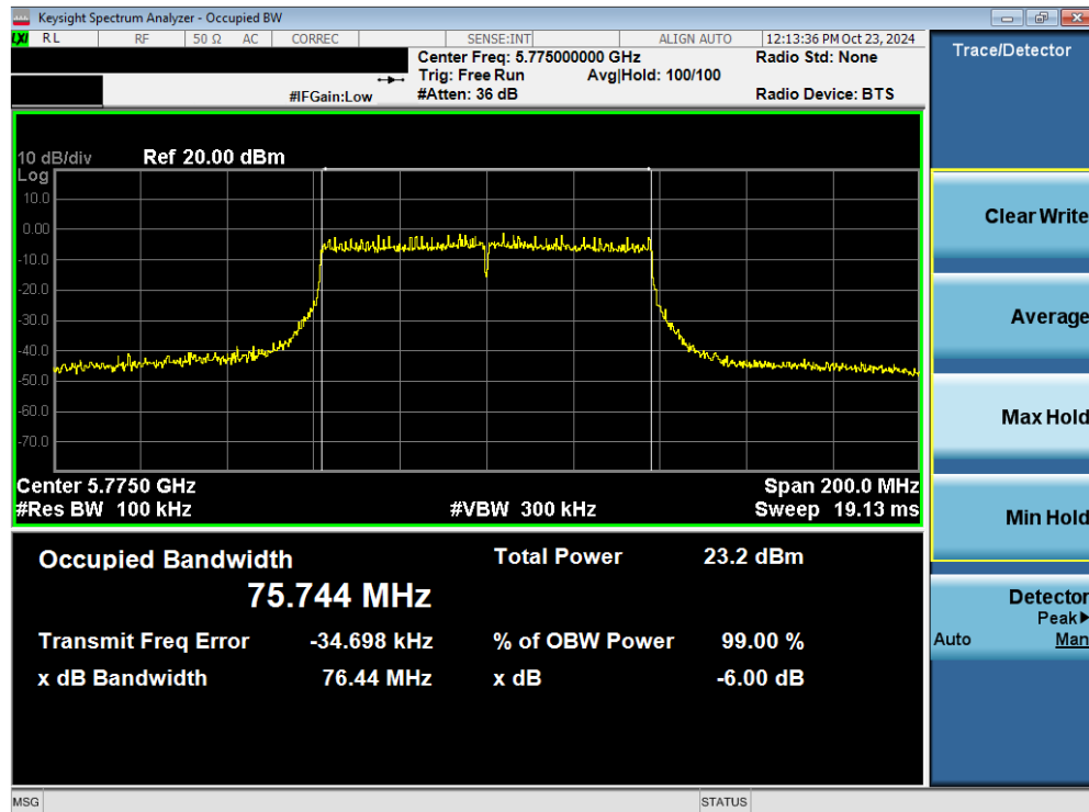
Plot 7-48. 6dB Bandwidth Plot MIMO ANT2 (80MHz 802.11ac (UNII Band 3) – Ch. 155)
