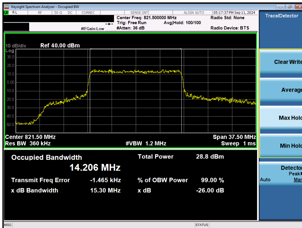
Plot 7-25. Occupied Bandwidth Plot (NR Band n26 - 15MHz 16-QAM - Full RB)
