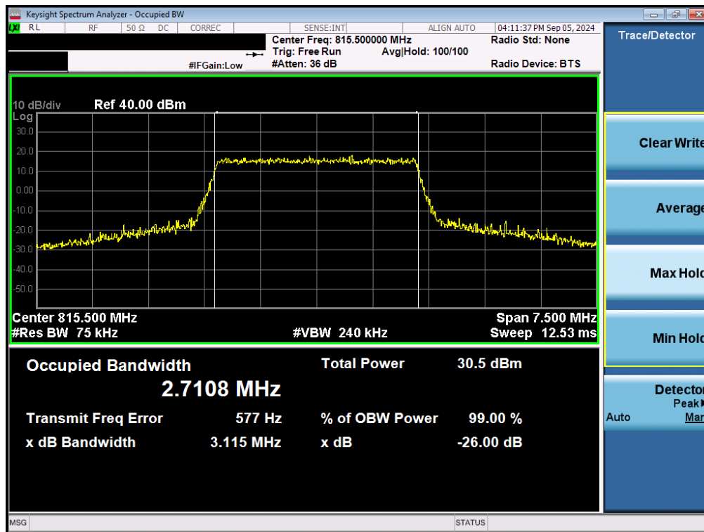
Plot 7-12. Occupied Bandwidth Plot (LTE Band 26 - 3MHz 16-QAM Low Channel - Full RB)
