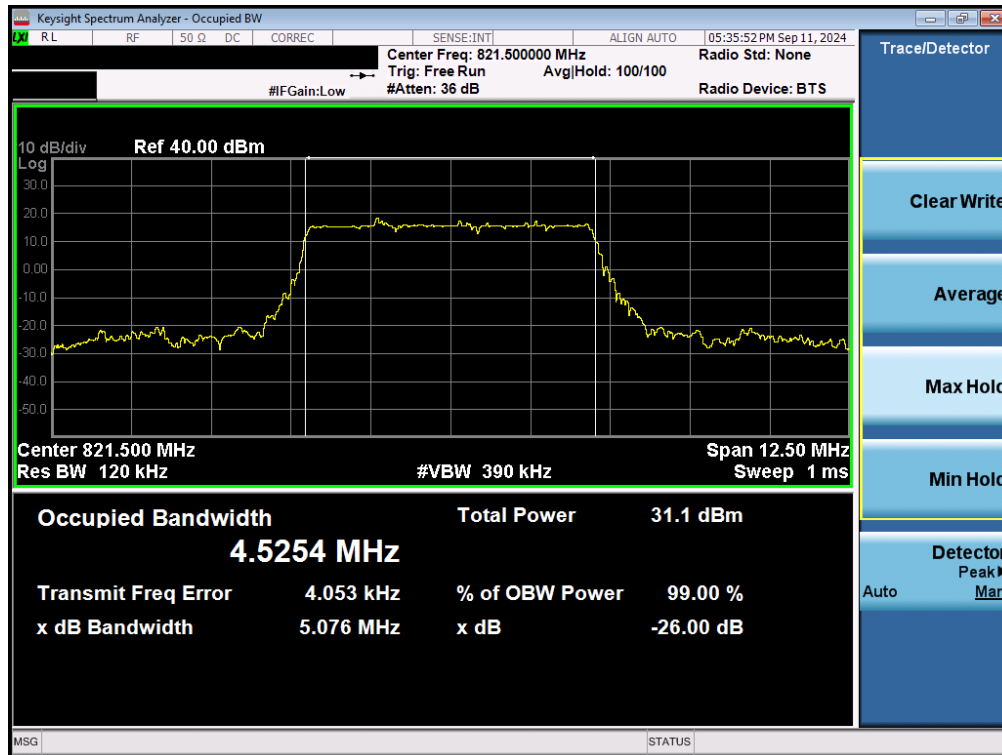
Plot 7-30. Occupied Bandwidth Plot (NR Band n26 - 5MHz \pi/2 BPSK High Channel - Full RB)
