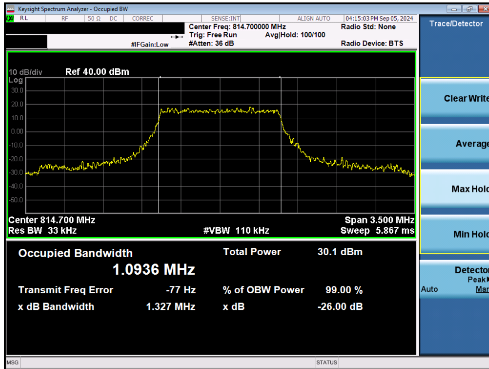
Plot 7-16. Occupied Bandwidth Plot (LTE Band 26 – 1.4MHz QPSK Low Channel- Full RB)
