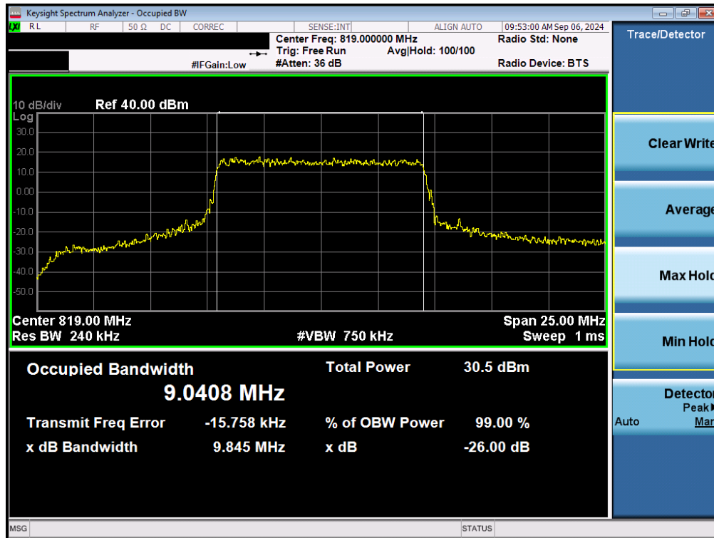
Plot 7-37. Occupied Bandwidth Plot (LTE Band 26 - 10MHz QPSK - Full RB)
