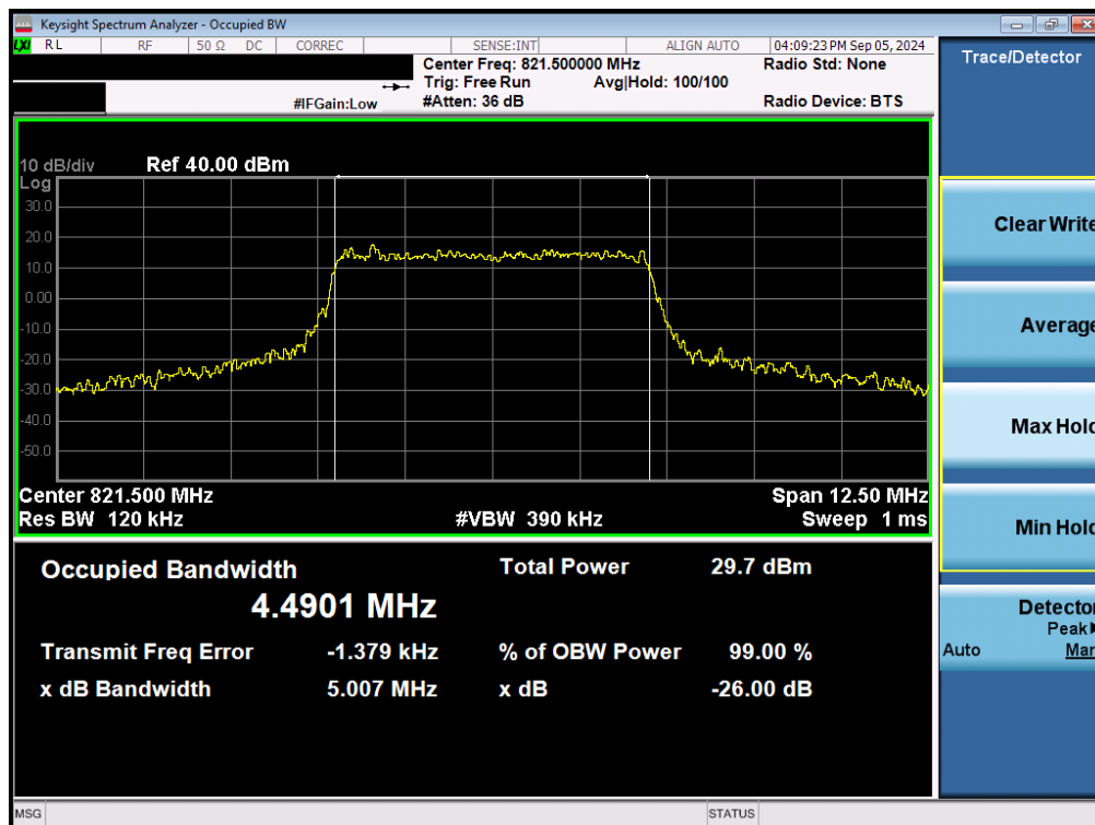
Plot 7-9. Occupied Bandwidth Plot (LTE Band 26 - 5MHz 16-QAM High Channel - Full RB)
