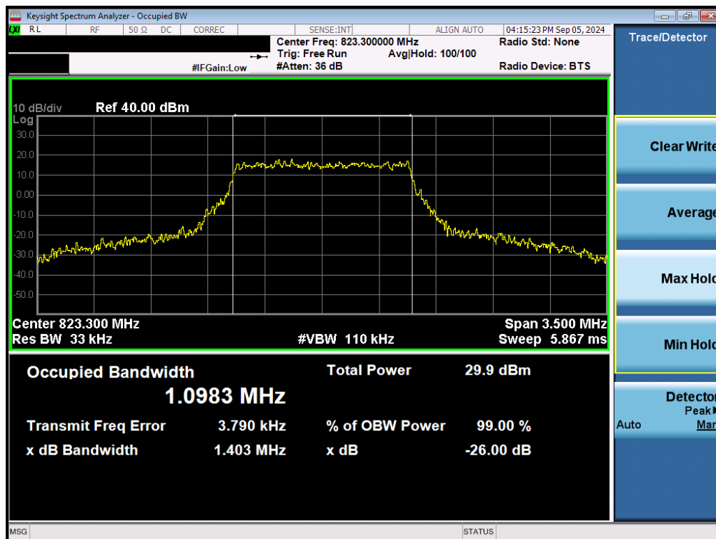
Plot 7-19. Occupied Bandwidth Plot (LTE Band 26 – 1.4MHz 16-QAM High Channel - Full RB)
