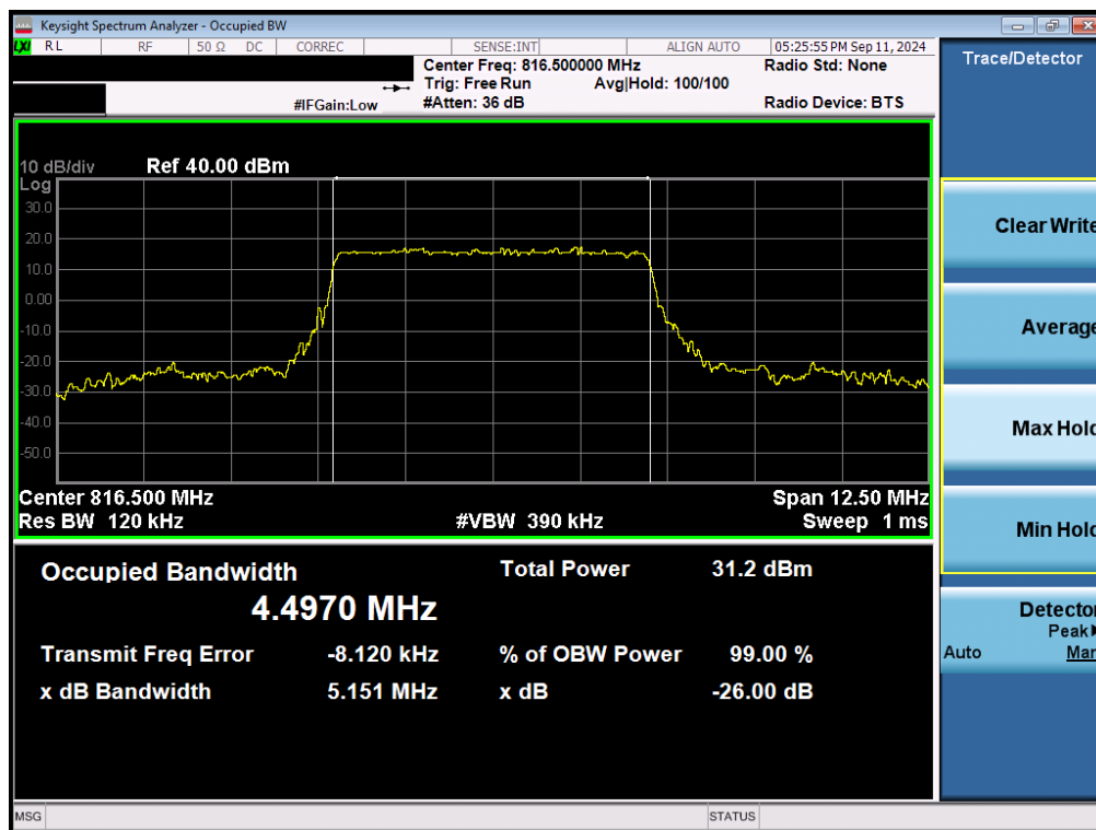
Plot 7-29. Occupied Bandwidth Plot (NR Band n26 - 5MHz \pi/2 BPSK Low Channel - Full RB)
