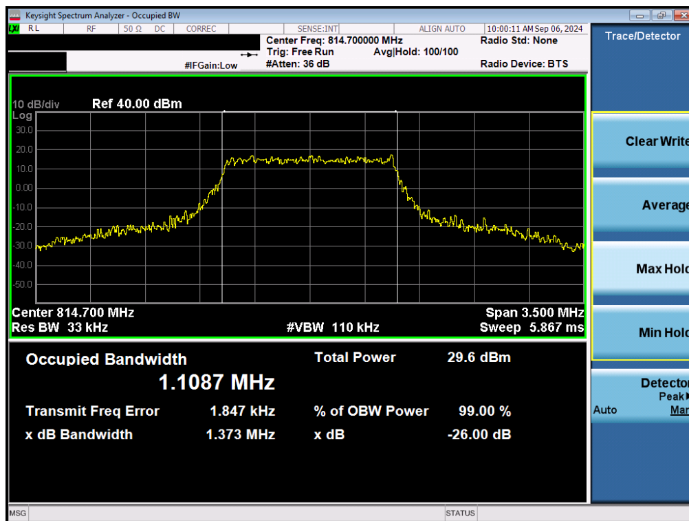
Plot 7-47. Occupied Bandwidth Plot (LTE Band 26 – 1.4MHz 16-QAM Low Channel - Full RB)
