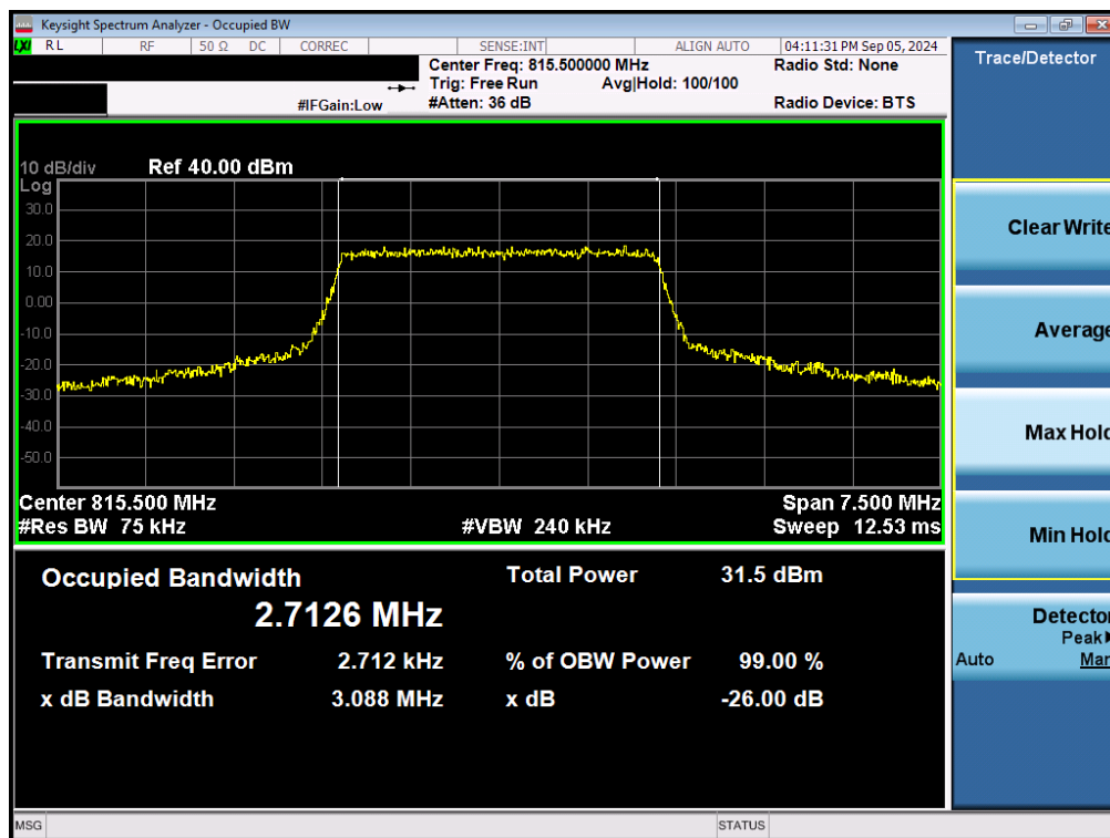
Plot 7-10. Occupied Bandwidth Plot (LTE Band 26 - 3MHz QPSK Low Channel- Full RB)
