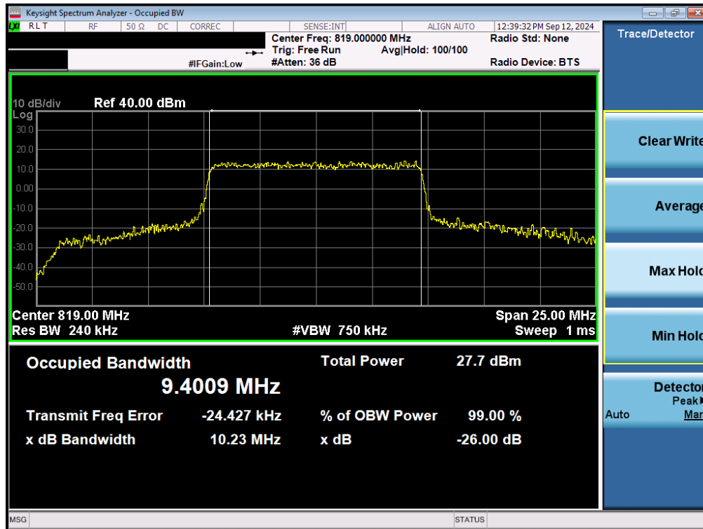
Plot 7-61. Occupied Bandwidth Plot (NR Band n26 - 10MHz 16-QAM - Full RB)
