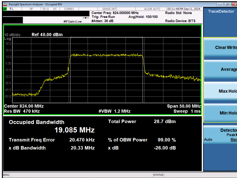
Plot 7-22. Occupied Bandwidth Plot (NR Band n26 - 20MHz 16-QAM - Full RB)
