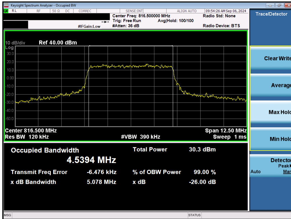
Plot 7-39. Occupied Bandwidth Plot (LTE Band 26 - 5MHz QPSK Low Channel- Full RB)
