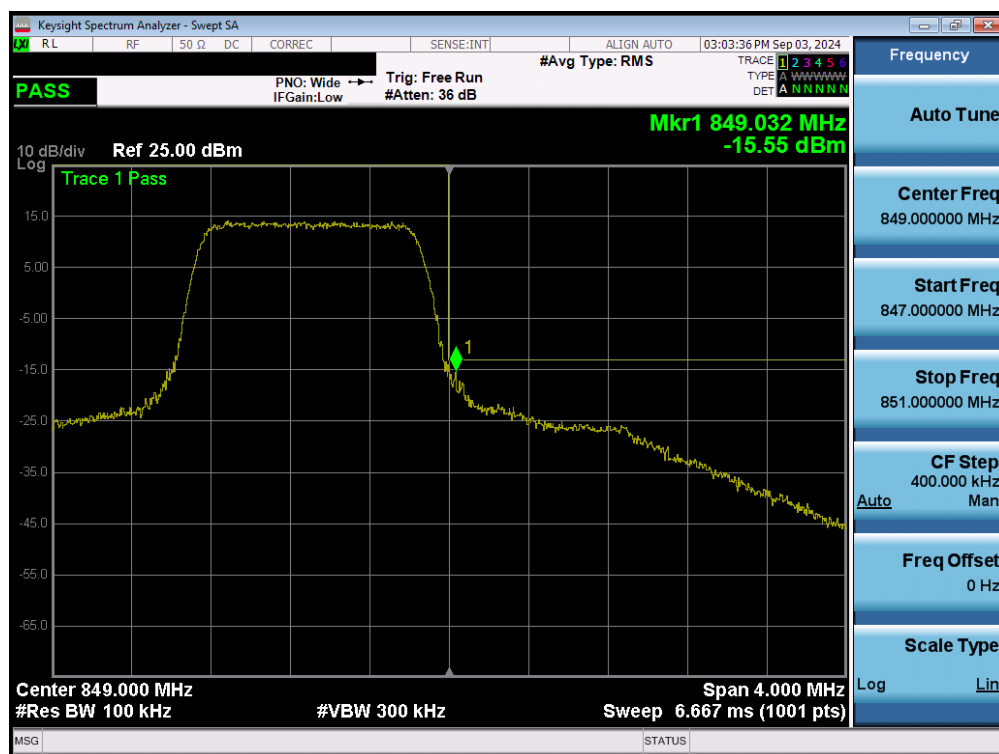
Plot 7-81. Upper Band Edge Plot (LTE Band 26/5 – 1.4MHz QPSK – Full RB - Ant1)
