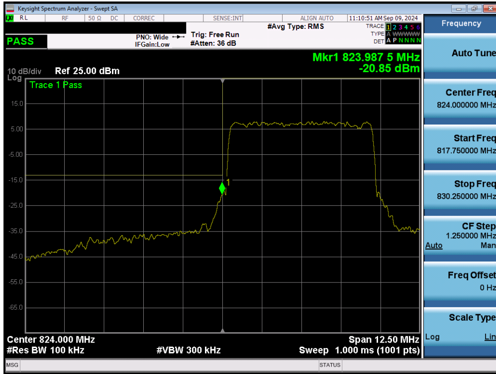
Plot 7-82. Lower Band Edge Plot (NR Band n26/5 – 5.0MHz - Full RB - Ant1)
