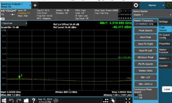
n77(3700~3980 MHz)\_50 M\_Band Edge\_Low\_BPSK\_1RB(3)
