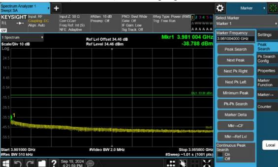
n77(3700~3980 MHz)\_50 M\_Band Edge\_High\_BPSK\_1RB(2)
