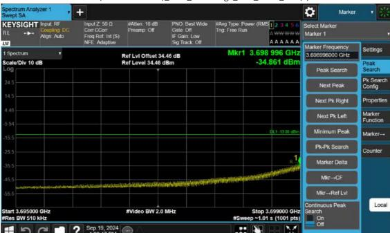
n77(3700~3980 MHz)\_40 M\_Band Edge\_Low\_BPSK\_1RB(2)
