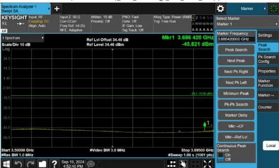
n77(3700~3980 MHz)\_80 M\_Band Edge\_Low\_BPSK\_1RB(3)
