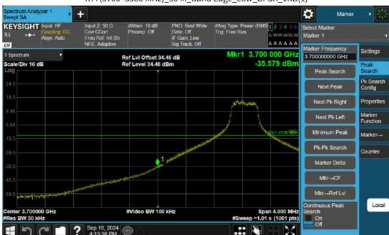
n77(3700~3980 MHz)\_50 M\_Band Edge\_Low\_BPSK\_1RB(1)
