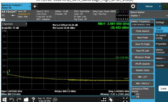
n77(3700~3980 MHz)\_80 M\_Band Edge\_High\_BPSK\_1RB(2)
