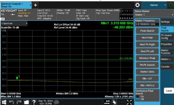
n77(3700~3980 MHz)\_40 M\_Band Edge\_Low\_BPSK\_1RB(3)
