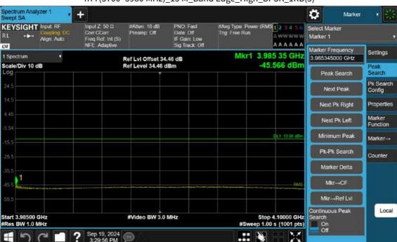
n77(3700~3980 MHz)\_15 M\_Band Edge\_High\_BPSK\_1RB(3)
