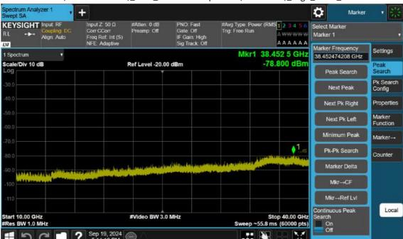
n77(3700~3980 MHz)\_90 M\_Conducted Spurious(Above10 G)\_High\_BPSK\_1RB
