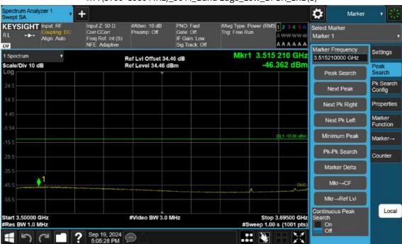
n77(3700~3980 MHz)\_90 M\_Band Edge\_Low\_BPSK\_1RB(3)
