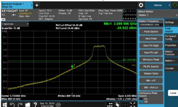
n77(3700~3980 MHz)\_15 M\_Band Edge\_Low\_BPSK\_1RB(1)
