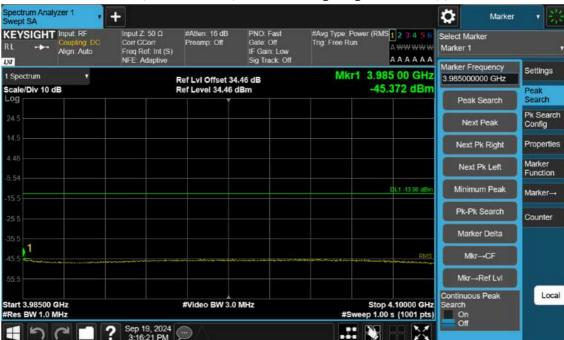
n77(3700~3980 MHz)\_10 M\_Band Edge\_High\_BPSK\_1RB(3)
