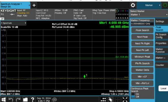
n77(3700~3980 MHz)\_60 M\_Band Edge\_High\_BPSK\_1RB(3)
