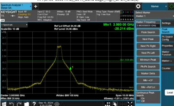
n77(3700~3980 MHz)\_10 M\_Band Edge\_High\_BPSK\_1RB(1)
