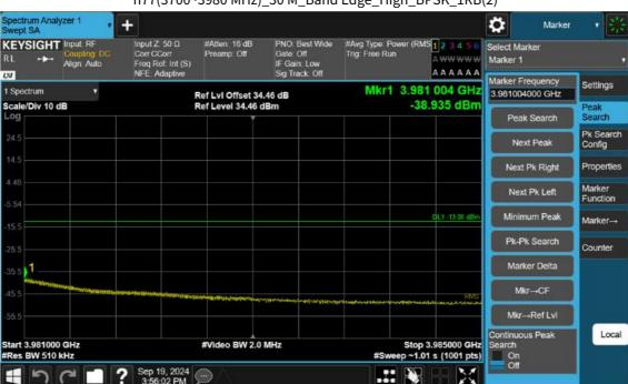
n77(3700~3980 MHz)\_30 M\_Band Edge\_High\_BPSK\_1RB(2)
