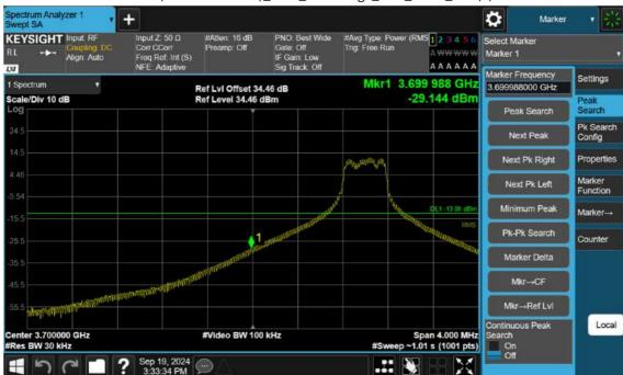
n77(3700~3980 MHz)\_20 M\_Band Edge\_Low\_BPSK\_1RB(1)
