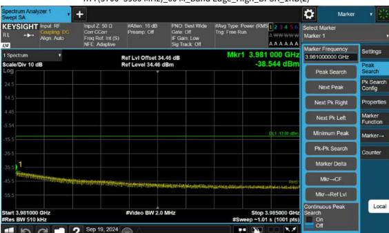
n77(3700~3980 MHz)\_60 M\_Band Edge\_High\_BPSK\_1RB(2)
