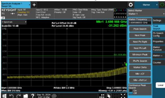
n77(3700~3980 MHz)\_10 M\_Band Edge\_Low\_BPSK\_1RB(2)
