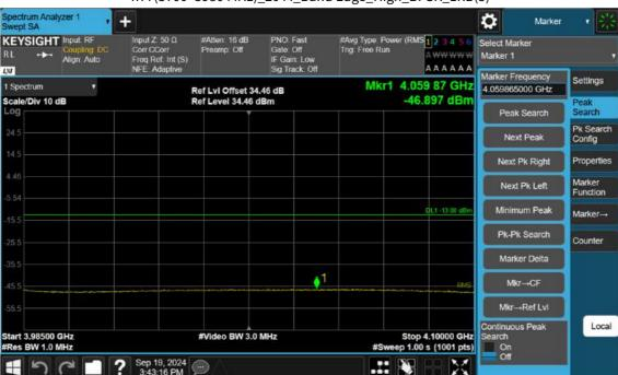
n77(3700~3980 MHz)\_20 M\_Band Edge\_High\_BPSK\_1RB(3)
