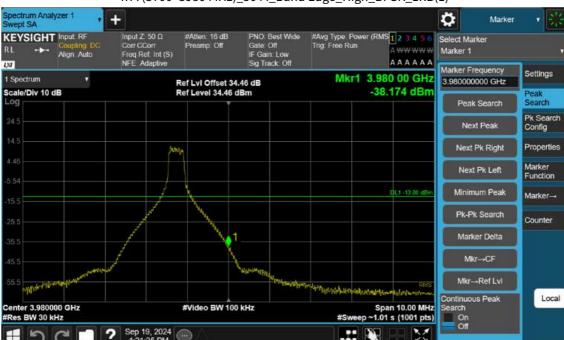
n77(3700~3980 MHz)\_50 M\_Band Edge\_High\_BPSK\_1RB(1)
