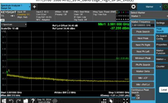
n77(3700~3980 MHz)\_20 M\_Band Edge\_High\_BPSK\_1RB(2)
