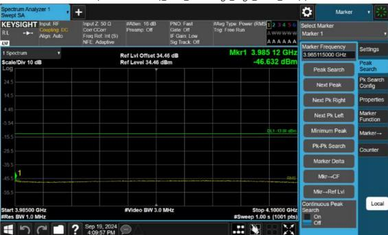
n77(3700~3980 MHz)\_40 M\_Band Edge\_High\_BPSK\_1RB(3)
