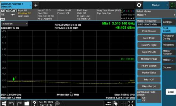
n77(3700~3980 MHz)\_60 M\_Band Edge\_Low\_BPSK\_1RB(3)
