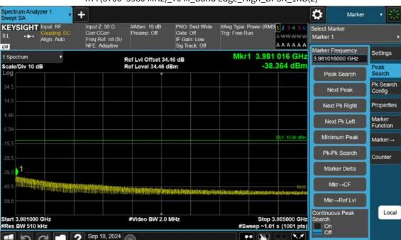
n77(3700~3980 MHz)\_70 M\_Band Edge\_High\_BPSK\_1RB(2)
