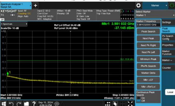
n77(3700~3980 MHz)\_40 M\_Band Edge\_High\_BPSK\_1RB(2)
