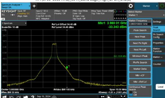
n77(3700~3980 MHz)\_60 M\_Band Edge\_High\_BPSK\_1RB(1)
