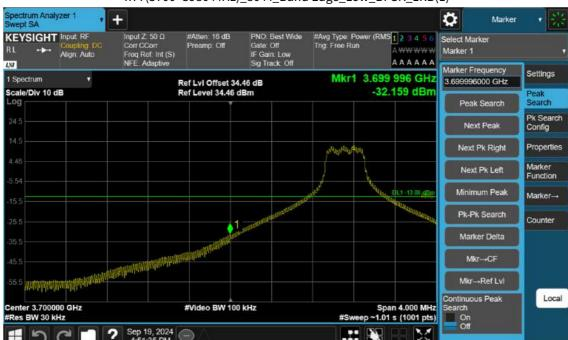
n77(3700~3980 MHz)\_80 M\_Band Edge\_Low\_BPSK\_1RB(1)
