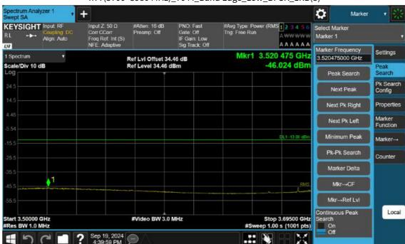
n77(3700~3980 MHz)\_70 M\_Band Edge\_Low\_BPSK\_1RB(3)
