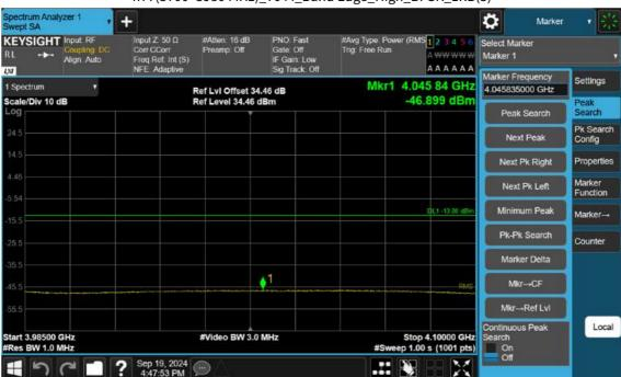
n77(3700~3980 MHz)\_70 M\_Band Edge\_High\_BPSK\_1RB(3)
