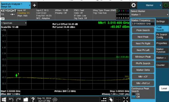
n77(3700~3980 MHz)\_15 M\_Band Edge\_Low\_BPSK\_1RB(3)
