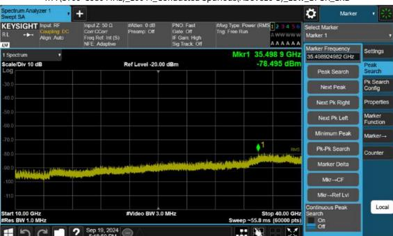
n77(3700~3980 MHz)\_100 M\_Conducted Spurious(Above10 G)\_Low\_BPSK\_1RB
