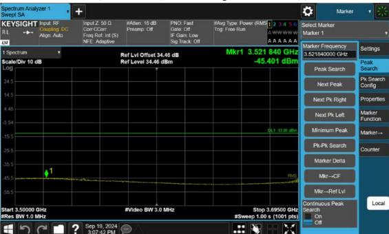
n77(3700~3980 MHz)\_10 M\_Band Edge\_Low\_BPSK\_1RB(3)
