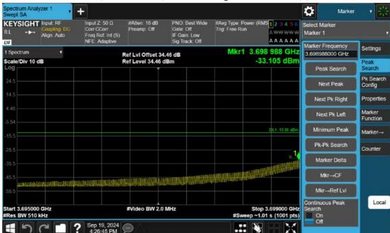
n77(3700~3980 MHz)\_60 M\_Band Edge\_Low\_BPSK\_1RB(2)
