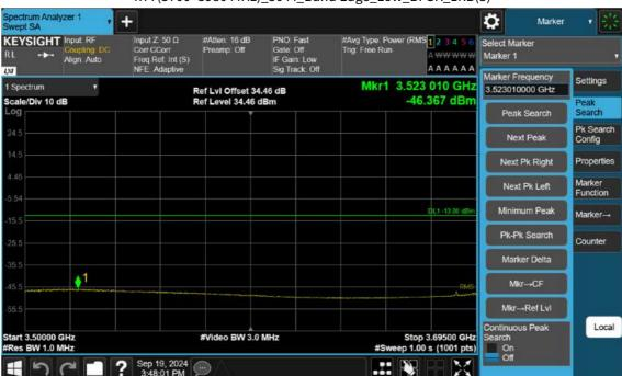
n77(3700~3980 MHz)\_30 M\_Band Edge\_Low\_BPSK\_1RB(3)
