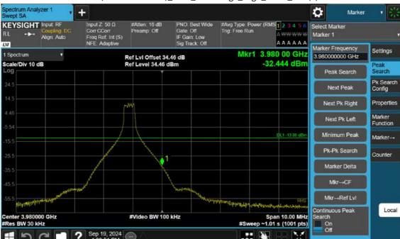
n77(3700~3980 MHz)\_40 M\_Band Edge\_High\_BPSK\_1RB(1)
