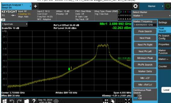
n77(3700~3980 MHz)\_40 M\_Band Edge\_Low\_BPSK\_1RB(1)
