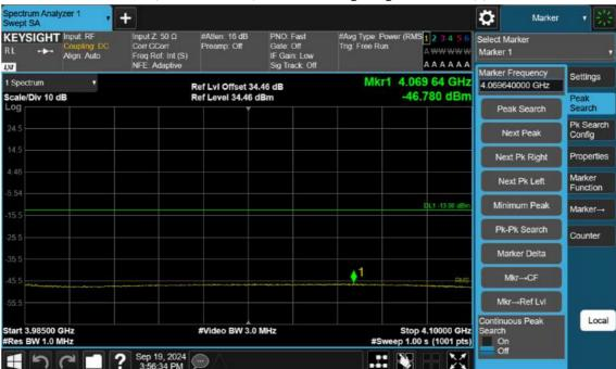
n77(3700~3980 MHz)\_30 M\_Band Edge\_High\_BPSK\_1RB(3)
