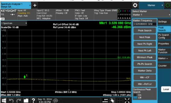
n77(3700~3980 MHz)\_20 M\_Band Edge\_Low\_BPSK\_1RB(3)
