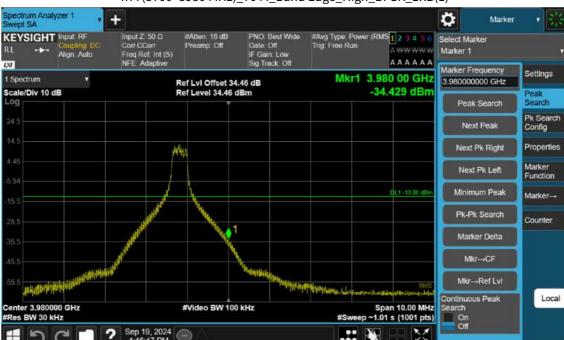
n77(3700~3980 MHz)\_70 M\_Band Edge\_High\_BPSK\_1RB(1)
