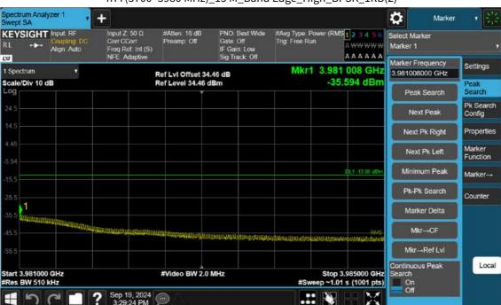
n77(3700~3980 MHz)\_15 M\_Band Edge\_High\_BPSK\_1RB(2)
