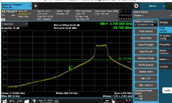
n77(3700~3980 MHz)\_60 M\_Band Edge\_Low\_BPSK\_1RB(1)
