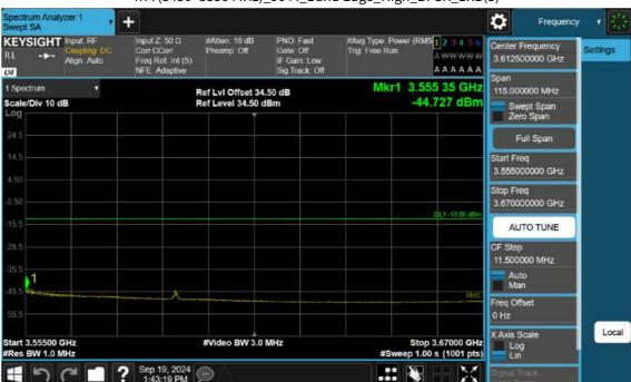
n77(3450~3550 MHz)\_90 M\_Band Edge\_High\_BPSK\_1RB(3)
