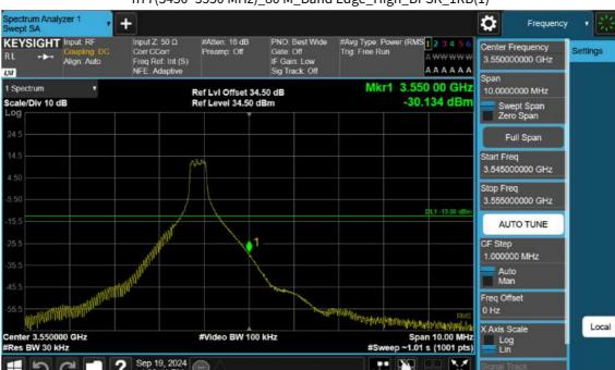
n77(3450~3550 MHz)\_80 M\_Band Edge\_High\_BPSK\_1RB(1)
