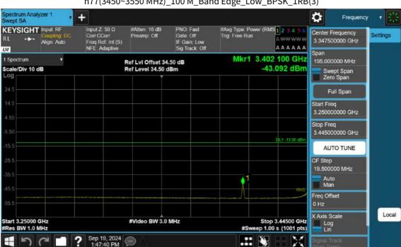
n77(3450~3550 MHz)\_100 M\_Band Edge\_Low\_BPSK\_1RB(3)
