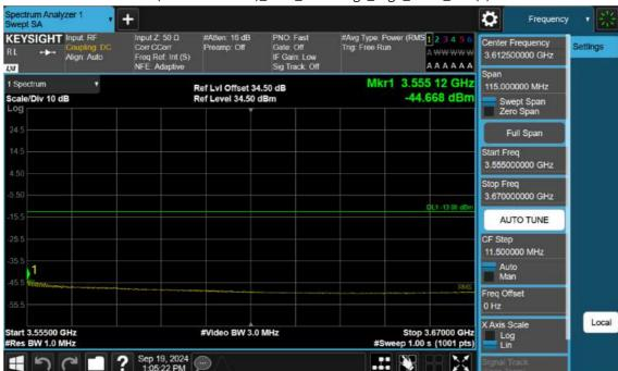
n77(3450~3550 MHz)\_60 M\_Band Edge\_High\_BPSK\_1RB(3)
