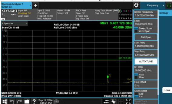
n77(3450~3550 MHz)\_90 M\_Band Edge\_Low\_BPSK\_1RB(3)
