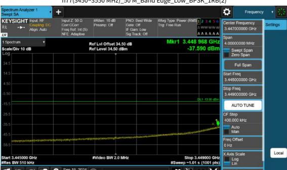
n77(3450~3550 MHz)\_50 M\_Band Edge\_Low\_BPSK\_1RB(2)
