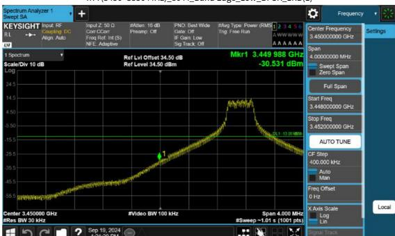
n77(3450~3550 MHz)\_80 M\_Band Edge\_Low\_BPSK\_1RB(1)
