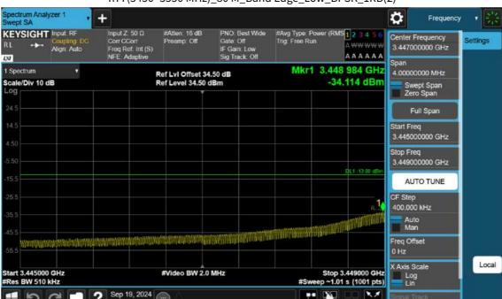
n77(3450~3550 MHz)\_80 M\_Band Edge\_Low\_BPSK\_1RB(2)
