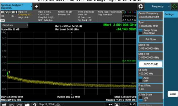
n77(3450~3550 MHz)\_90 M\_Band Edge\_High\_BPSK\_1RB(2)
