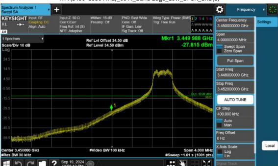
n77(3450~3550 MHz)\_60 M\_Band Edge\_Low\_BPSK\_1RB(1)
