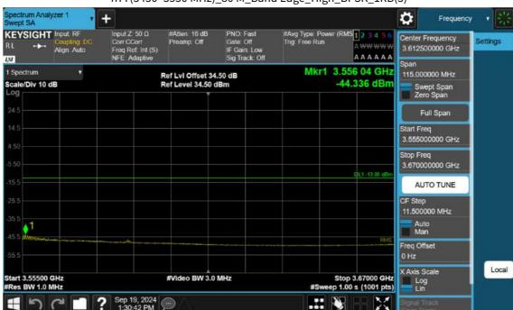
n77(3450~3550 MHz)\_80 M\_Band Edge\_High\_BPSK\_1RB(3)
