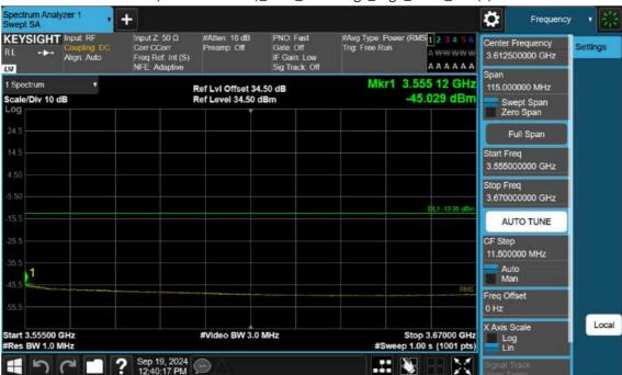
n77(3450~3550 MHz)\_40 M\_Band Edge\_High\_BPSK\_1RB(3)
