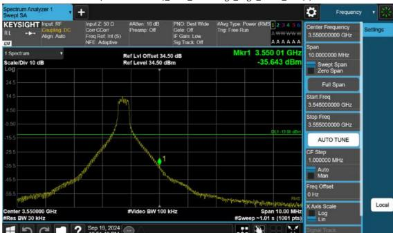
n77(3450~3550 MHz)\_50 M\_Band Edge\_High\_BPSK\_1RB(1)
