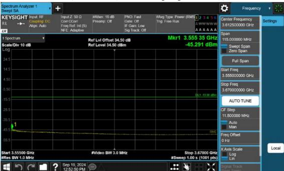
n77(3450~3550 MHz)\_50 M\_Band Edge\_High\_BPSK\_1RB(3)
