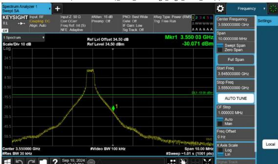
n77(3450~3550 MHz)\_90 M\_Band Edge\_High\_BPSK\_1RB(1)
