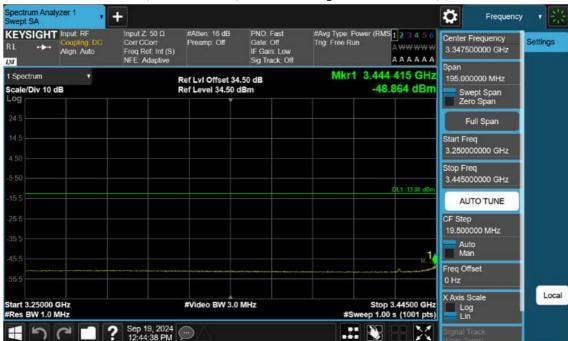
n77(3450~3550 MHz)\_50 M\_Band Edge\_Low\_BPSK\_1RB(3)
