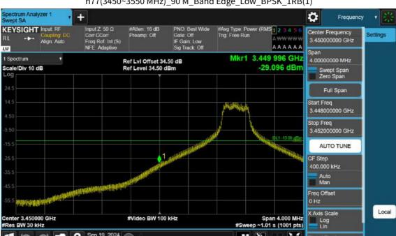
n77(3450~3550 MHz)\_90 M\_Band Edge\_Low\_BPSK\_1RB(1)
