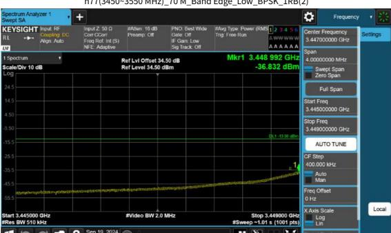
n77(3450~3550 MHz)\_70 M\_Band Edge\_Low\_BPSK\_1RB(2)
