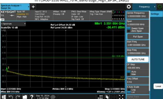
n77(3450~3550 MHz)\_70 M\_Band Edge\_High\_BPSK\_1RB(2)
