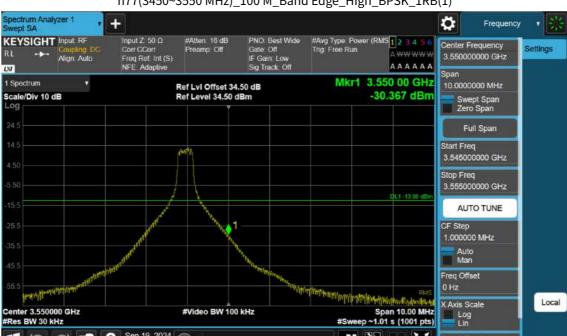
n77(3450~3550 MHz)\_100 M\_Band Edge\_High\_BPSK\_1RB(1)
