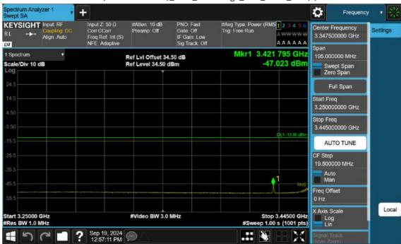
n77(3450~3550 MHz)\_60 M\_Band Edge\_Low\_BPSK\_1RB(3)
