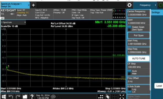
n77(3450~3550 MHz)\_60 M\_Band Edge\_High\_BPSK\_1RB(2)
