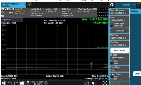
n77(3450~3550 MHz)\_80 M\_Band Edge\_Low\_BPSK\_1RB(3)
