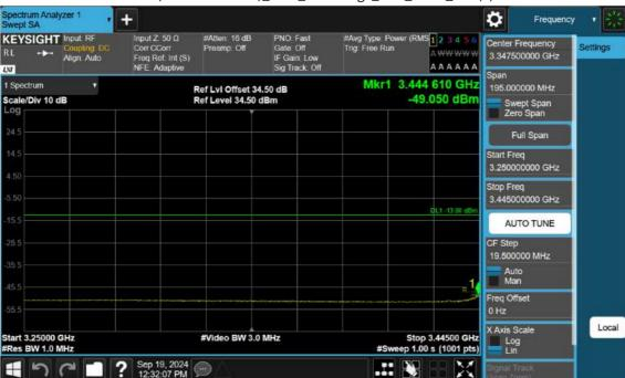
n77(3450~3550 MHz)\_40 M\_Band Edge\_Low\_BPSK\_1RB(3)
