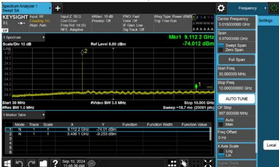
n77(3450~3550 MHz)\_10 M\_Conducted Spurious(30 M-10 G)\_Mid\_BPSK\_1RB
