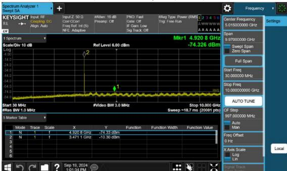
n77(3450~3550 MHz)\_60 M\_Conducted Spurious(30 M-10 G)\_Mid\_BPSK\_1RB
