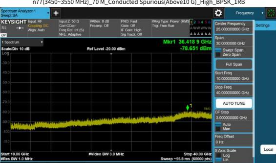
n77(3450~3550 MHz)\_70 M\_Conducted Spurious(Above10 G)\_High\_BPSK\_1RB
