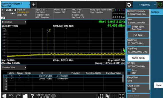
n77(3450~3550 MHz)\_70 M\_Conducted Spurious(30 M-10 G)\_Mid\_BPSK\_1RB
