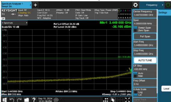
n77(3450~3550 MHz)\_40 M\_Band Edge\_Low\_BPSK\_1RB(2)
