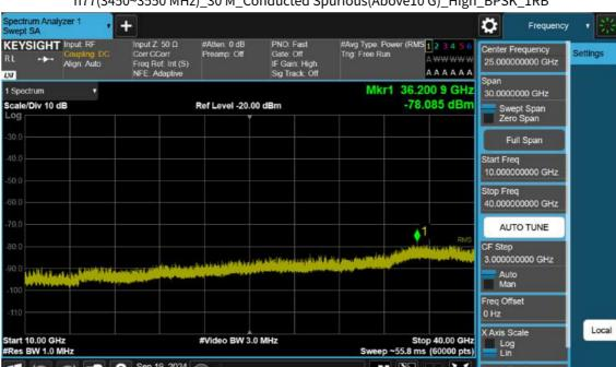
n77(3450~3550 MHz)\_30 M\_Conducted Spurious(Above10 G)\_High\_BPSK\_1RB
