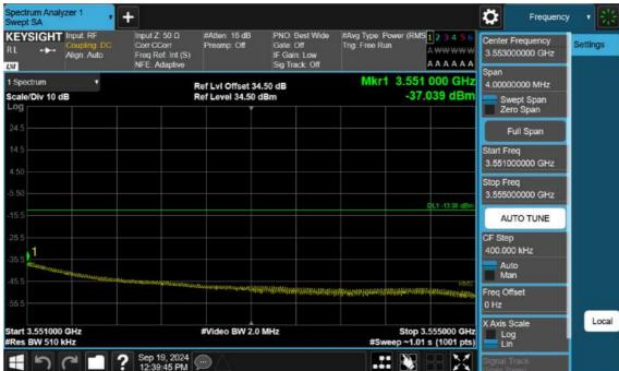
n77(3450~3550 MHz)\_40 M\_Band Edge\_High\_BPSK\_1RB(2)
