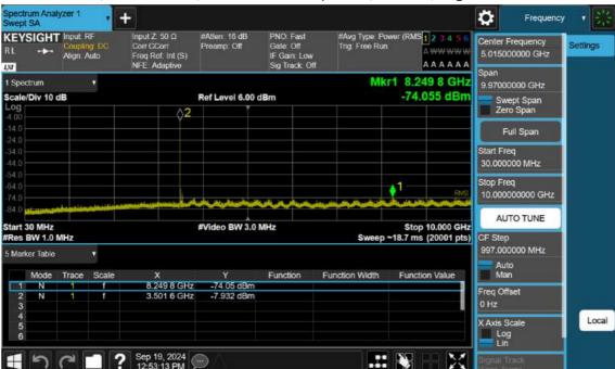
n77(3450~3550 MHz)\_50 M\_Conducted Spurious(30 M-10 G)\_High\_BPSK\_1RB
