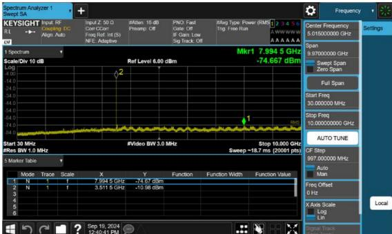
n77(3450~3550 MHz)\_40 M\_Conducted Spurious(30 M-10 G)\_High\_BPSK\_1RB
