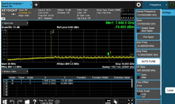
n77(3450~3550 MHz)\_100 M\_Conducted Spurious(30 M-10 G)\_Low\_BPSK\_1RB
