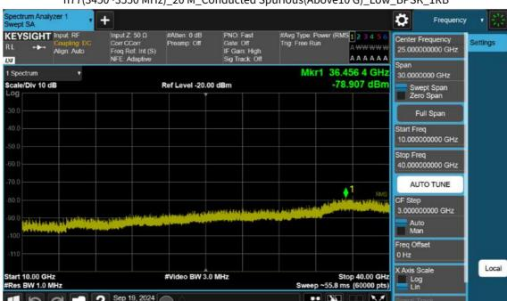
n77(3450~3550 MHz)\_20 M\_Conducted Spurious(Above10 G)\_Low\_BPSK\_1RB
