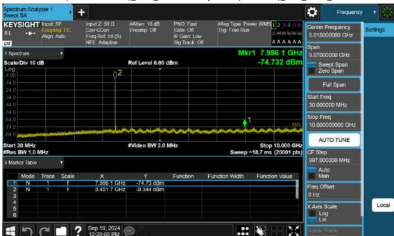
n77(3450~3550 MHz)\_30 M\_Conducted Spurious(30 M-10 G)\_Low\_BPSK\_1RB
