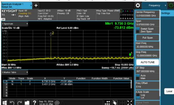
n77(3450~3550 MHz)\_40 M\_Conducted Spurious(30 M-10 G)\_Low\_BPSK\_1RB
