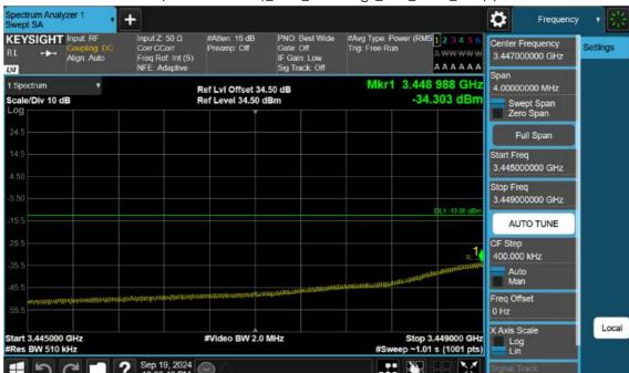
n77(3450~3550 MHz)\_20 M\_Band Edge\_Low\_BPSK\_1RB(2)
