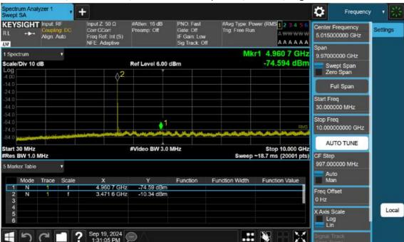
n77(3450~3550 MHz)\_80 M\_Conducted Spurious(30 M-10 G)\_High\_BPSK\_1RB
