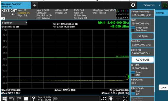
n77(3450~3550 MHz)\_15 M\_Band Edge\_Low\_BPSK\_1RB(3)
