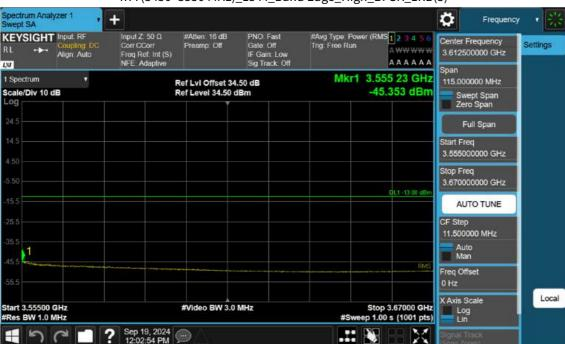
n77(3450~3550 MHz)\_15 M\_Band Edge\_High\_BPSK\_1RB(3)
