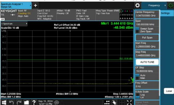
n77(3450~3550 MHz)\_20 M\_Band Edge\_Low\_BPSK\_1RB(3)
