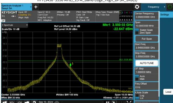
n77(3450~3550 MHz)\_15 M\_Band Edge\_High\_BPSK\_1RB(1)
