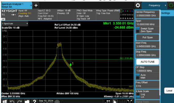
n77(3450~3550 MHz)\_10 M\_Band Edge\_High\_BPSK\_1RB(1)
