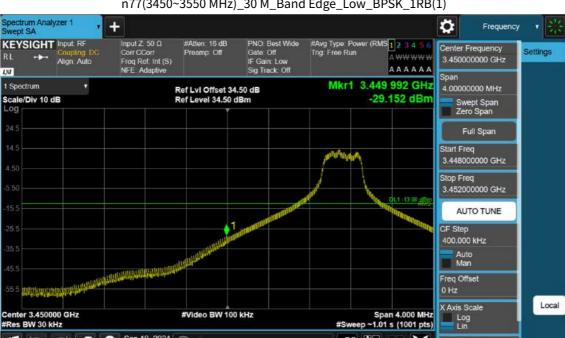
n77(3450~3550 MHz)\_30 M\_Band Edge\_Low\_BPSK\_1RB(1)
