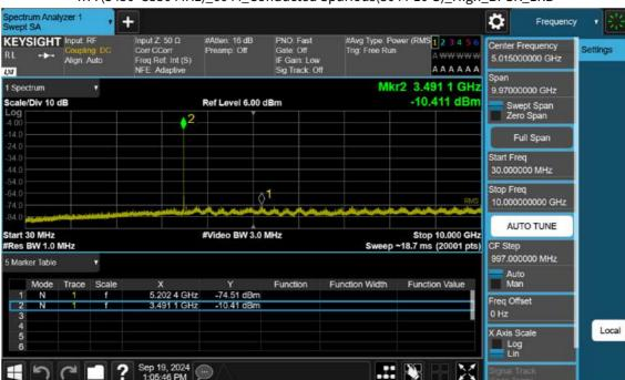
n77(3450~3550 MHz)\_60 M\_Conducted Spurious(30 M-10 G)\_High\_BPSK\_1RB
