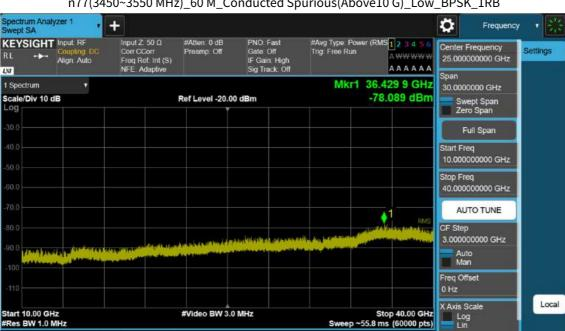
n77(3450~3550 MHz)\_60 M\_Conducted Spurious(Above10 G)\_Low\_BPSK\_1RB
