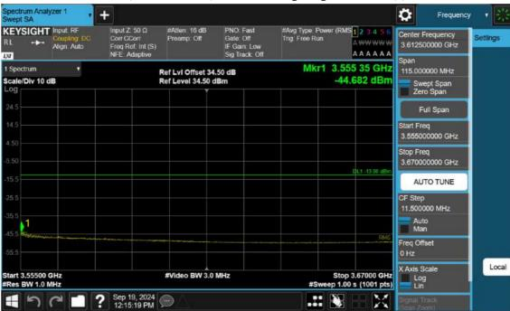
n77(3450~3550 MHz)\_20 M\_Band Edge\_High\_BPSK\_1RB(3)
