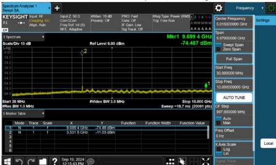
n77(3450~3550 MHz)\_20 M\_Conducted Spurious(30 M-10 G)\_High\_BPSK\_1RB
