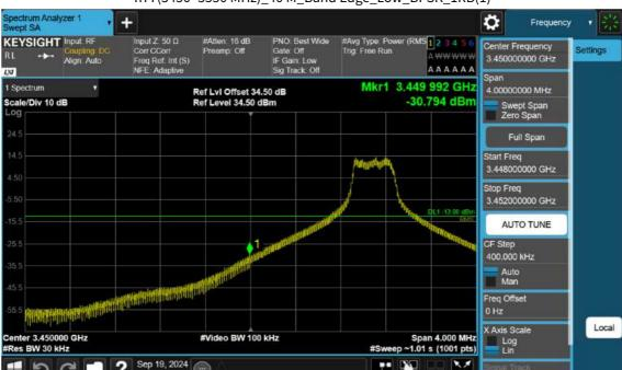
n77(3450~3550 MHz)\_40 M\_Band Edge\_Low\_BPSK\_1RB(1)
