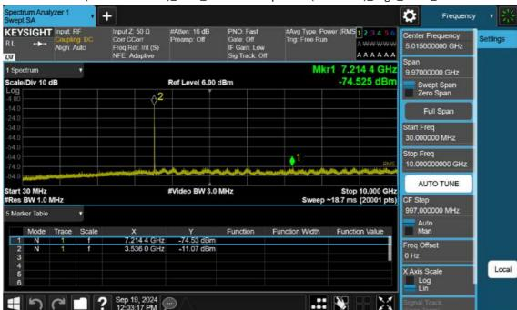
n77(3450~3550 MHz)\_15 M\_Conducted Spurious(30 M-10 G)\_High\_BPSK\_1RB
