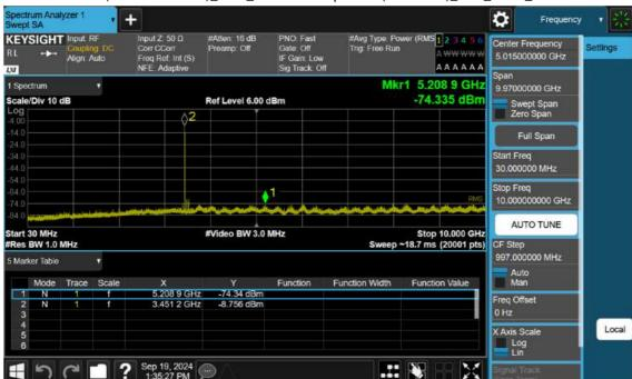
n77(3450~3550 MHz)\_90 M\_Conducted Spurious(30 M-10 G)\_Low\_BPSK\_1RB
