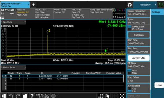
n77(3450~3550 MHz)\_80 M\_Conducted Spurious(30 M-10 G)\_Low\_BPSK\_1RB
