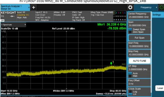
n77(3450~3550 MHz)\_80 M\_Conducted Spurious(Above10 G)\_High\_BPSK\_1RB
