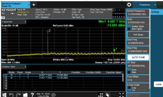
n77(3450~3550 MHz)\_90 M\_Conducted Spurious(30 M-10 G)\_High\_BPSK\_1RB
