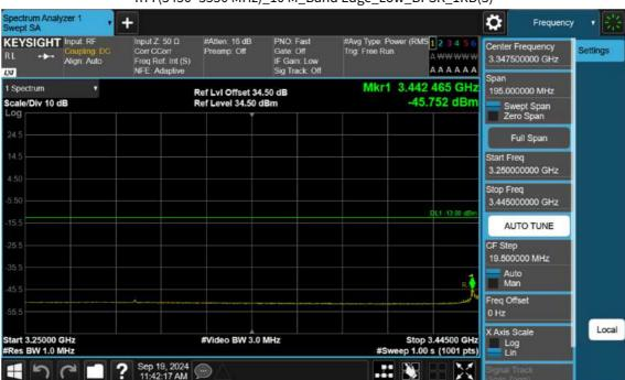
n77(3450~3550 MHz)\_10 M\_Band Edge\_Low\_BPSK\_1RB(3)
