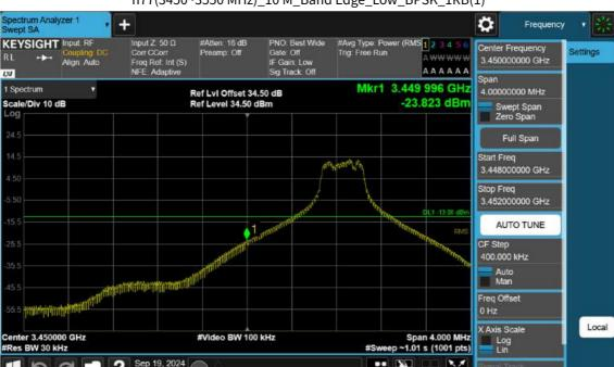
n77(3450~3550 MHz)\_10 M\_Band Edge\_Low\_BPSK\_1RB(1)
