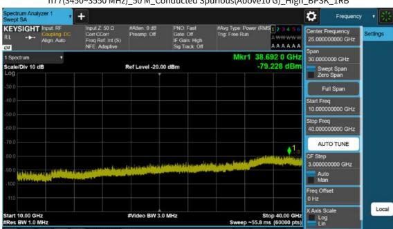
n77(3450~3550 MHz)\_50 M\_Conducted Spurious(Above10 G)\_High\_BPSK\_1RB
