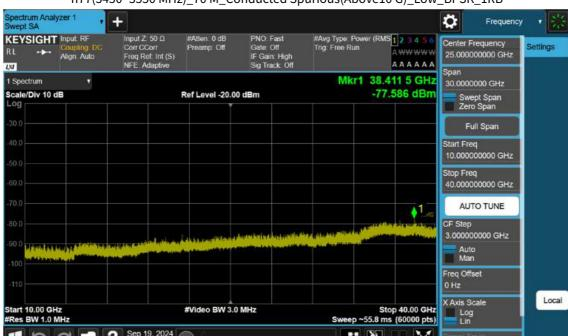
n77(3450~3550 MHz)\_70 M\_Conducted Spurious(Above10 G)\_Low\_BPSK\_1RB
