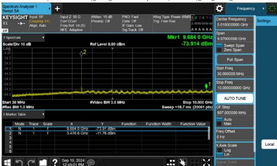
n77(3450~3550 MHz)\_50 M\_Conducted Spurious(30 M-10 G)\_Mid\_BPSK\_1RB
