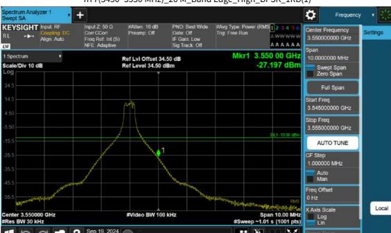
n77(3450~3550 MHz)\_20 M\_Band Edge\_High\_BPSK\_1RB(1)
