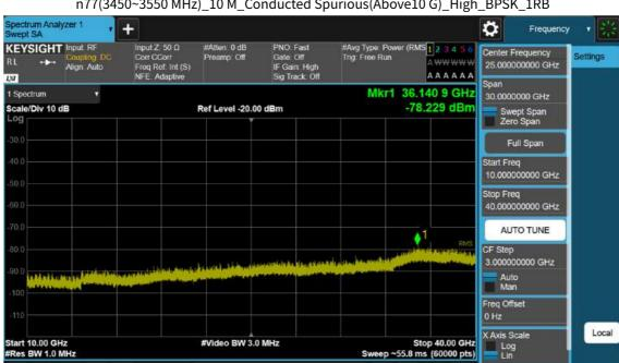
n77(3450~3550 MHz)\_10 M\_Conducted Spurious(Above10 G)\_High\_BPSK\_1RB
