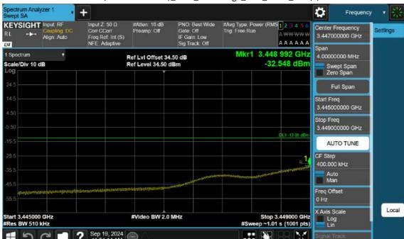
n77(3450~3550 MHz)\_15 M\_Band Edge\_Low\_BPSK\_1RB(2)
