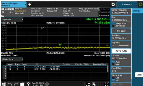
n77(3450~3550 MHz)\_80 M\_Conducted Spurious(30 M-10 G)\_Mid\_BPSK\_1RB
