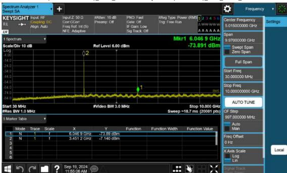
n77(3450~3550 MHz)\_15 M\_Conducted Spurious(30 M-10 G)\_Low\_BPSK\_1RB
