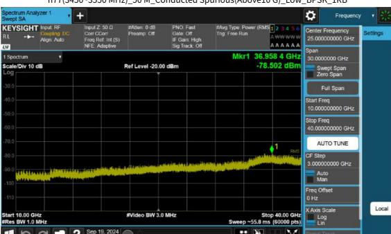
n77(3450~3550 MHz)\_50 M\_Conducted Spurious(Above10 G)\_Low\_BPSK\_1RB
