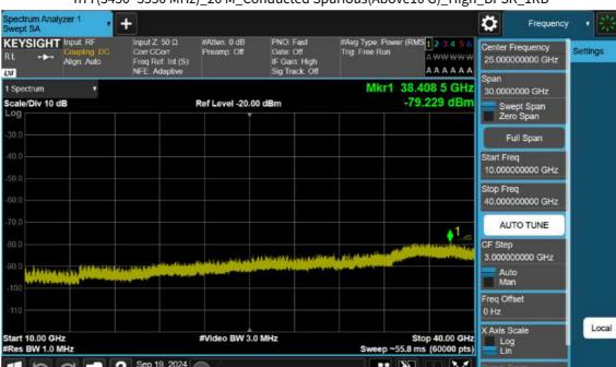
n77(3450~3550 MHz)\_20 M\_Conducted Spurious(Above10 G)\_High\_BPSK\_1RB
