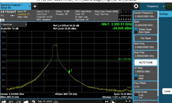
n77(3450~3550 MHz)\_40 M\_Band Edge\_High\_BPSK\_1RB(1)
