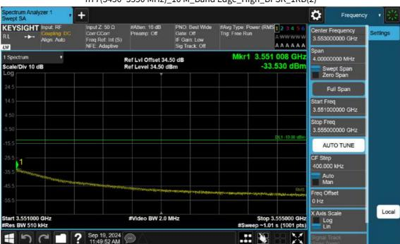
n77(3450~3550 MHz)\_10 M\_Band Edge\_High\_BPSK\_1RB(2)
