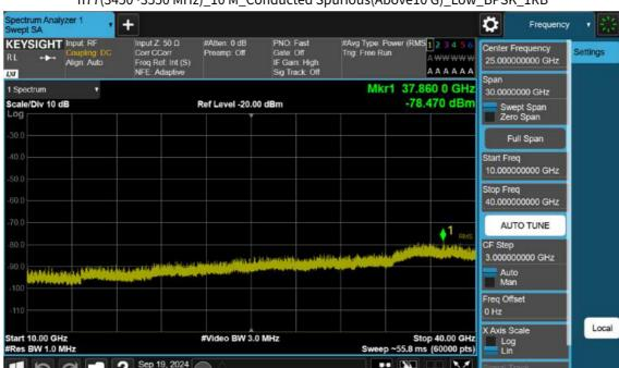
n77(3450~3550 MHz)\_10 M\_Conducted Spurious(Above10 G)\_Low\_BPSK\_1RB
