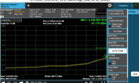
n77(3450~3550 MHz)\_10 M\_Band Edge\_Low\_BPSK\_1RB(2)
