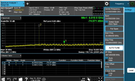
n77(3450~3550 MHz)\_90 M\_Conducted Spurious(30 M-10 G)\_Mid\_BPSK\_1RB
