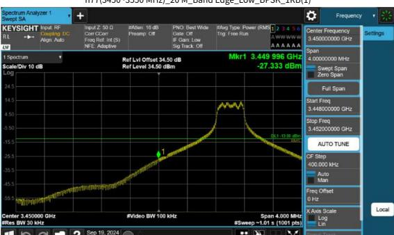
n77(3450~3550 MHz)\_20 M\_Band Edge\_Low\_BPSK\_1RB(1)
