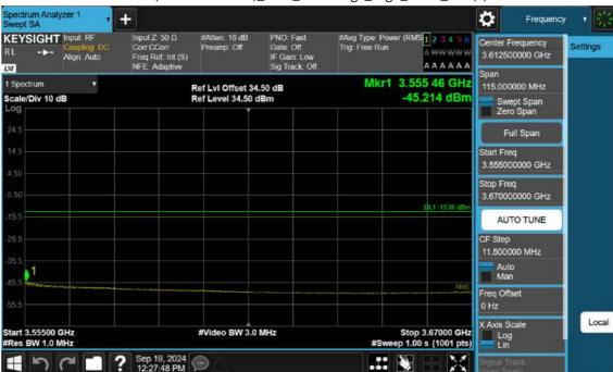
n77(3450~3550 MHz)\_30 M\_Band Edge\_High\_BPSK\_1RB(3)
