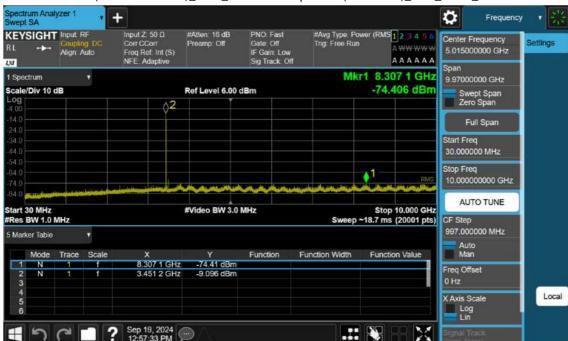
n77(3450~3550 MHz)\_60 M\_Conducted Spurious(30 M-10 G)\_Low\_BPSK\_1RB
