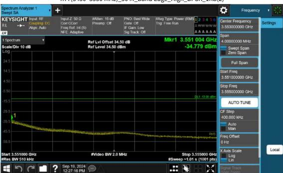
n77(3450~3550 MHz)\_30 M\_Band Edge\_High\_BPSK\_1RB(2)
