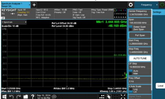
n77(3450~3550 MHz)\_30 M\_Band Edge\_Low\_BPSK\_1RB(3)
