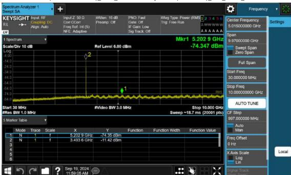
n77(3450~3550 MHz)\_15 M\_Conducted Spurious(30 M-10 G)\_Mid\_BPSK\_1RB
