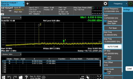
n77(3450~3550 MHz)\_20 M\_Conducted Spurious(30 M-10 G)\_Low\_BPSK\_1RB
