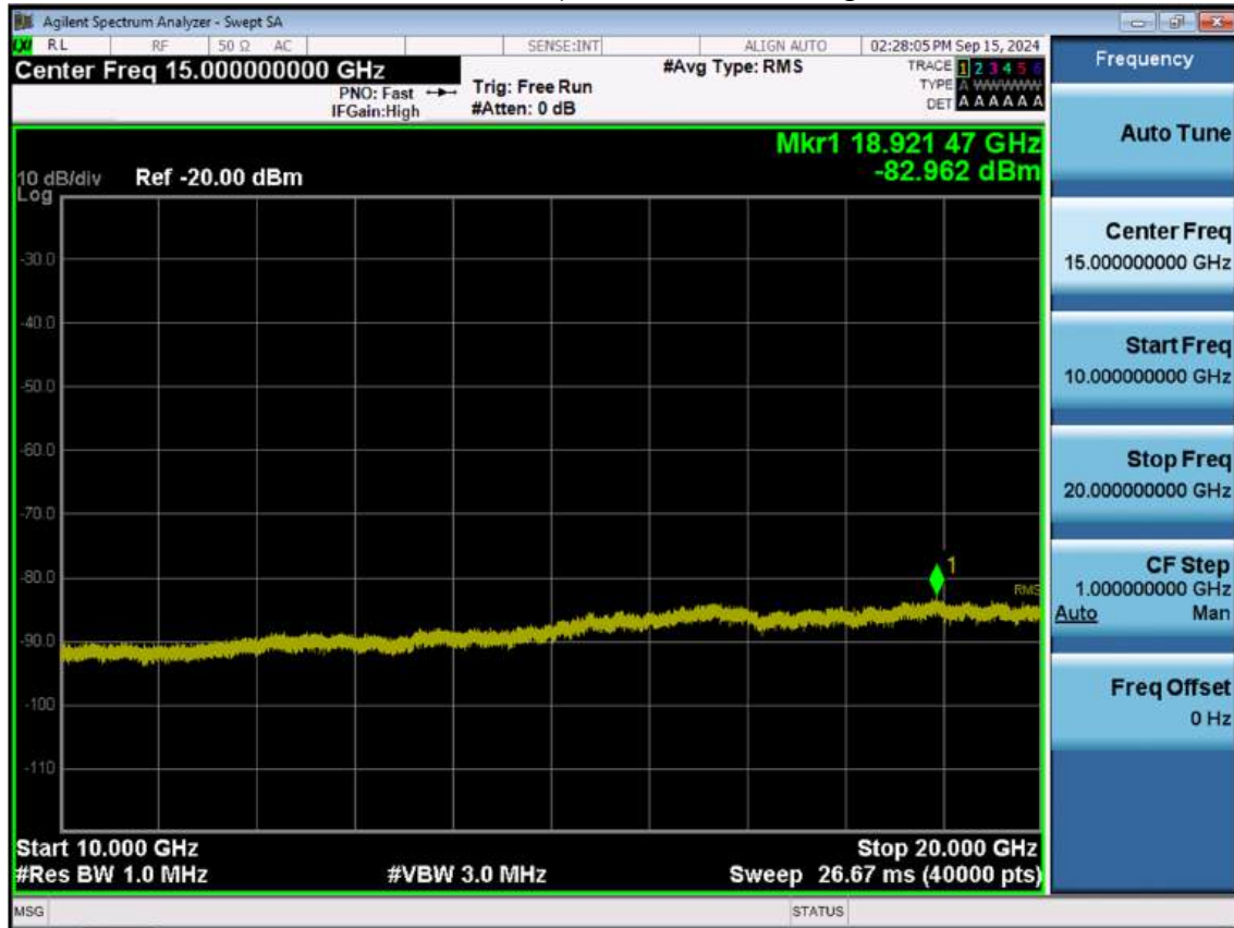
LTE B66_3 M_Conducted Spurious(10 G-26.5 G)_High_QPSK_1RB
