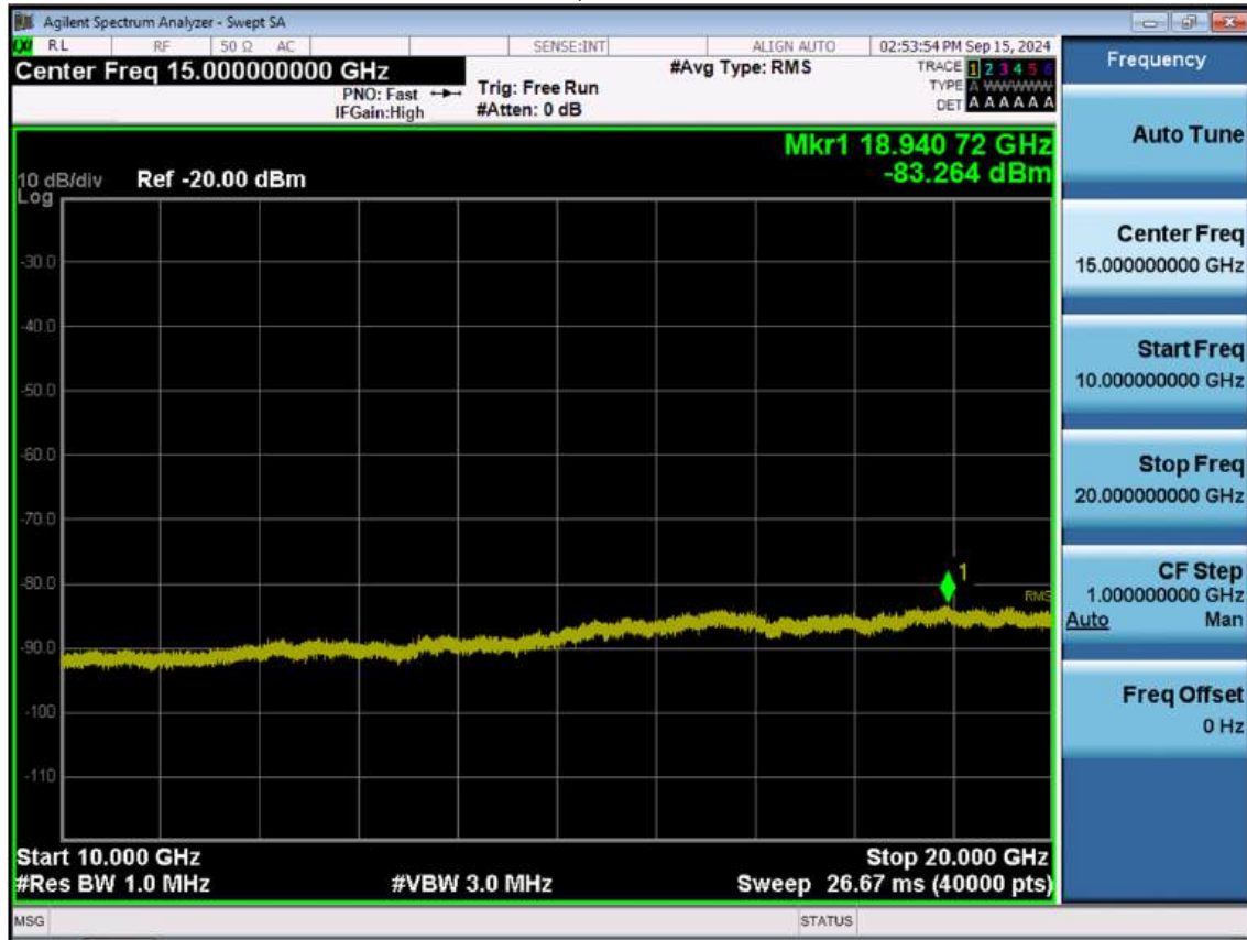
LTE B66_20 M_Conducted Spurious(10 G-26.5 G)_Mid_QPSK_1RB
