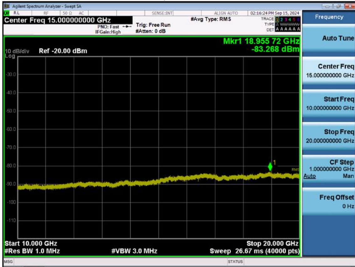
LTE B66_1.4M_Conducted Spurious(10 G-26.5 G)_Low_QPSK_1RB
