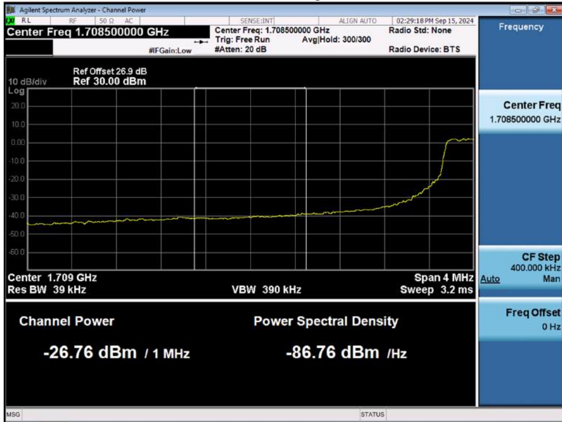
LTE B66_5 M_Extended Band Edge_Low_QPSK_FullRB
