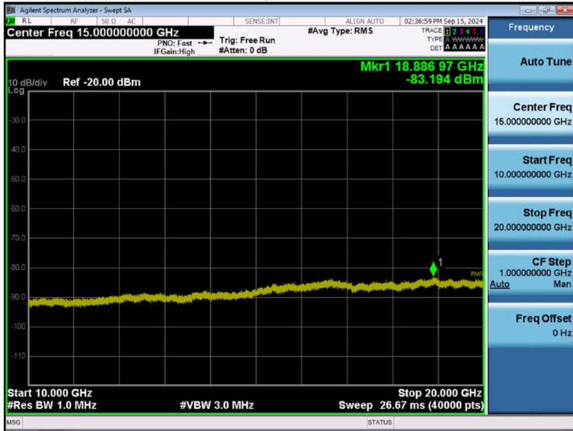
LTE B66_10 M_Conducted Spurious(10 G-26.5 G)_Low_QPSK_1RB
