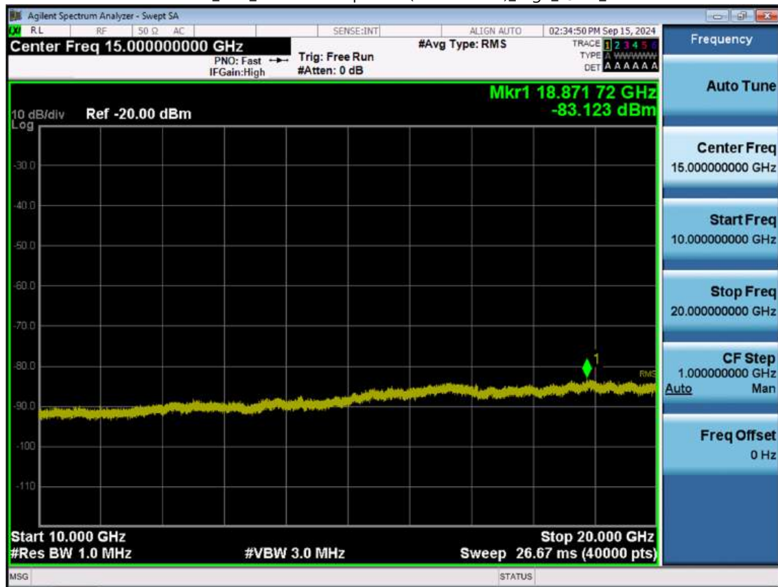
LTE B66_5 M_Conducted Spurious(10 G-26.5 G)_High_QPSK_1RB
