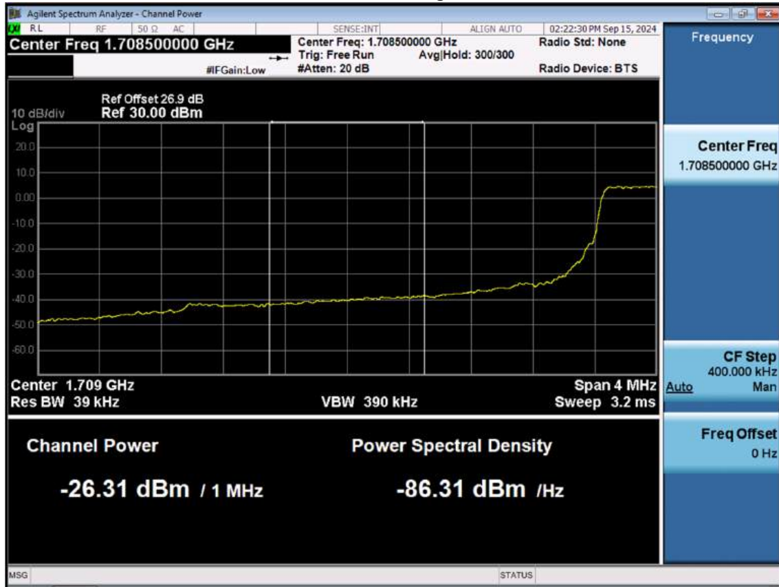
LTE B66_3 M_Extended Band Edge_Low_QPSK_FullRB
