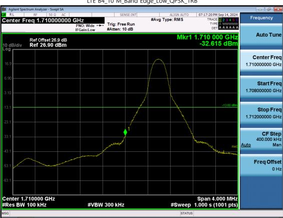
LTE B4\_10 M\_Band Edge\_Low\_QPSK\_1RB
