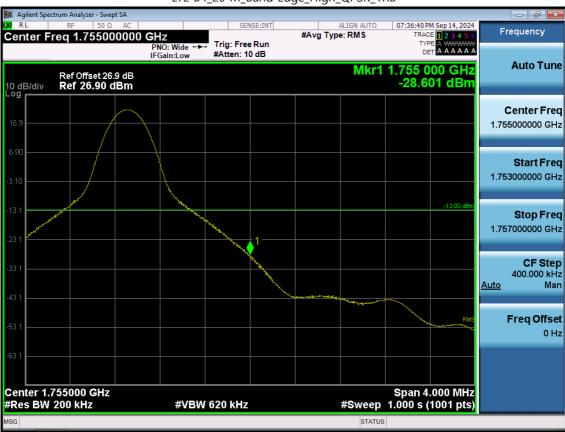
LTE B4\_20 M\_Band Edge\_High\_QPSK\_1RB
