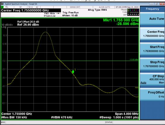
LTE B4\_15 M\_Band Edge\_High\_QPSK\_1RB
