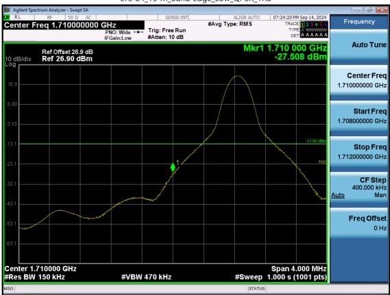
LTE B4\_15 M\_Band Edge\_Low\_QPSK\_1RB
