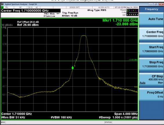
LTE B4\_5 M\_Band Edge\_Low\_QPSK\_1RB
