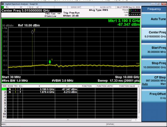
LTE B2\_10 M\_Conducted Spurious(30 M-10 G)\_Mid\_QPSK\_1RB
