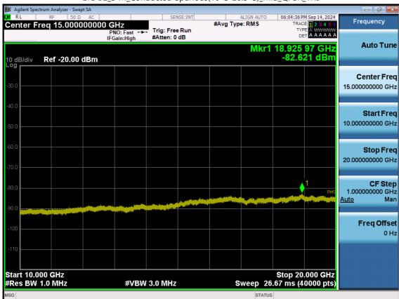
LTE B2\_3 M\_Conducted Spurious(10 G-26.5 G)\_Mid\_QPSK\_1RB
