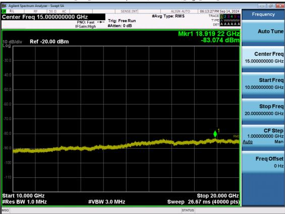
LTE B2\_5 M\_Conducted Spurious(10 G-26.5 G)\_High\_QPSK\_1RB
