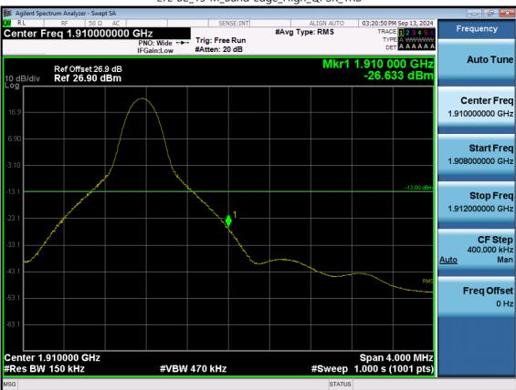
LTE B2\_15 M\_Band Edge\_High\_QPSK\_1RB
