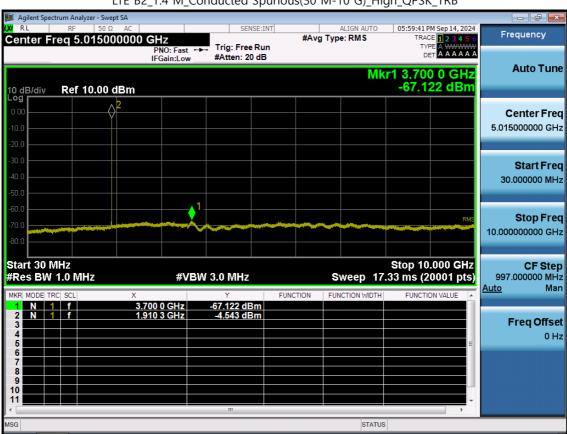
LTE B2\_1.4 M\_Conducted Spurious(30 M-10 G)\_High\_QPSK\_1RB
