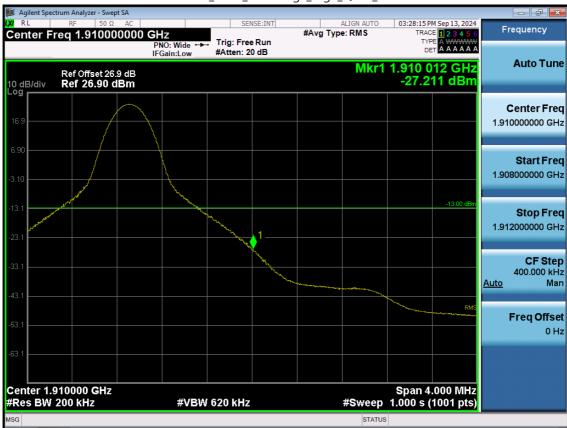
LTE B2\_20 M\_Band Edge\_High\_QPSK\_1RB
