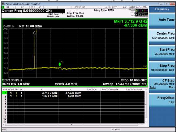
LTE B2\_5 M\_Conducted Spurious(30 M-10 G)\_Mid\_QPSK\_1RB
