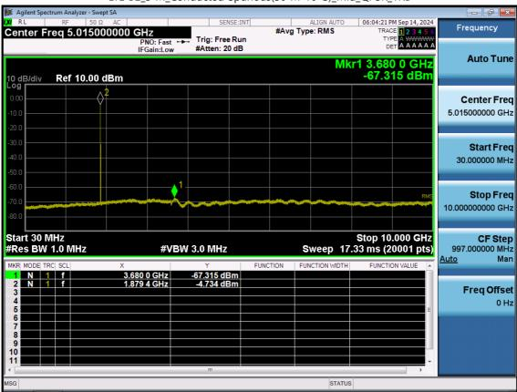
LTE B2\_3 M\_Conducted Spurious(30 M-10 G)\_Mid\_QPSK\_1RB
