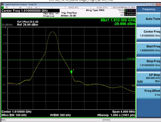
LTE B2\_10 M\_Band Edge\_High\_QPSK\_1RB
