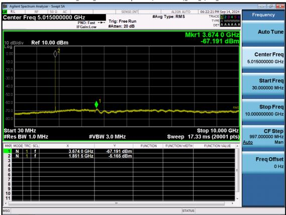
LTE B2\_15 M\_Conducted Spurious(30 M-10 G)\_Low\_QPSK\_1RB
