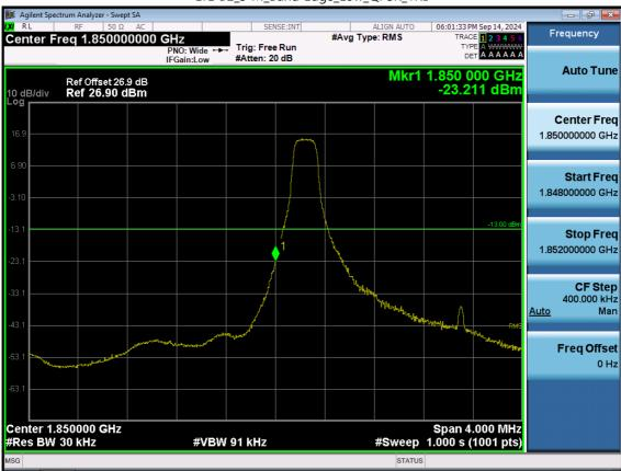
LTE B2\_3 M\_Band Edge\_Low\_QPSK\_1RB
