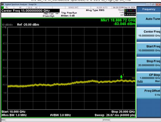
LTE B2\_10 M\_Conducted Spurious(10 G-26.5 G)\_High\_QPSK\_1RB
