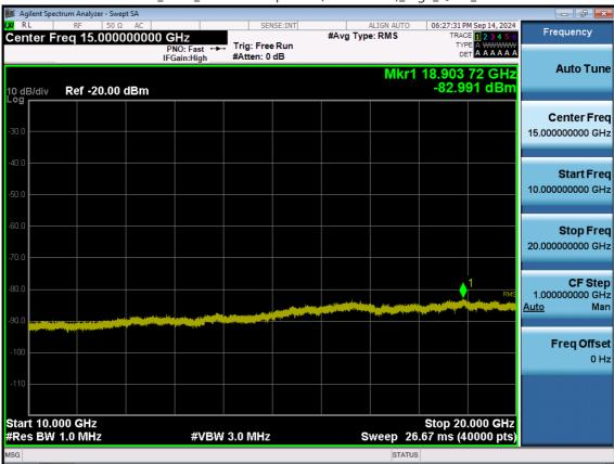
LTE B2\_15 M\_Conducted Spurious(10 G-26.5 G)\_High\_QPSK\_1RB
