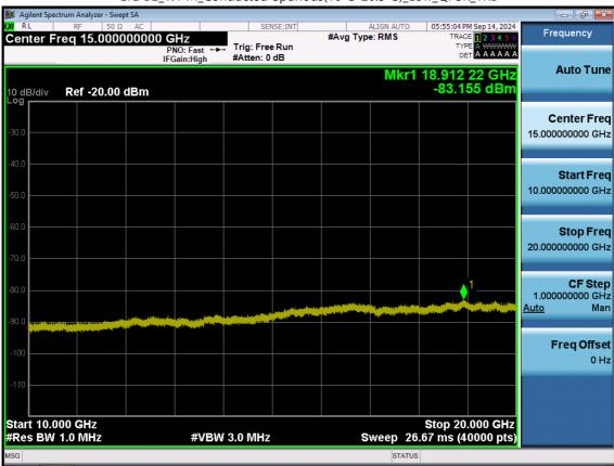
LTE B2\_1.4 M\_Conducted Spurious(10 G-26.5 G)\_Low\_QPSK\_1RB
