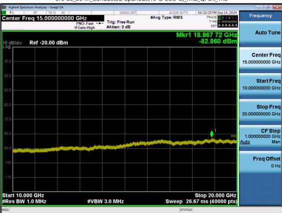
LTE B2\_20 M\_Conducted Spurious(10 G-26.5 G)\_Mid\_QPSK\_1RB
