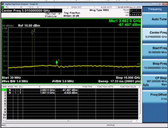
LTE B2\_5 M\_Conducted Spurious(30 M-10 G)\_Low\_QPSK\_1RB
