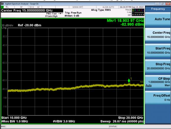
LTE B2\_20 M\_Conducted Spurious(10 G-26.5 G)\_High\_QPSK\_1RB
