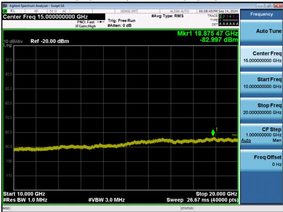
LTE B2\_5 M\_Conducted Spurious(10 G-26.5 G)\_Low\_QPSK\_1RB
