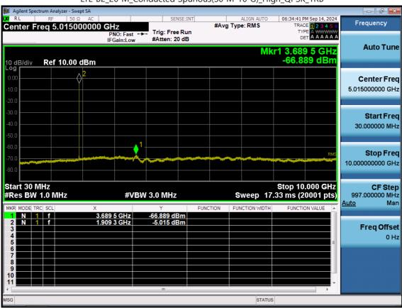
LTE B2\_20 M\_Conducted Spurious(30 M-10 G)\_High\_QPSK\_1RB
