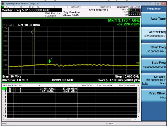
LTE B2\_20 M\_Conducted Spurious(30 M-10 G)\_Low\_QPSK\_1RB
