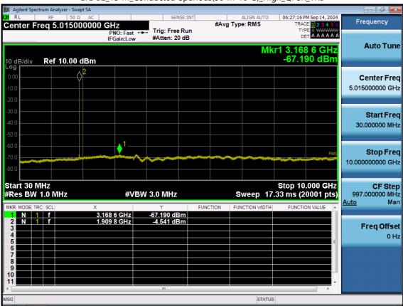
LTE B2\_15 M\_Conducted Spurious(30 M-10 G)\_High\_QPSK\_1RB
