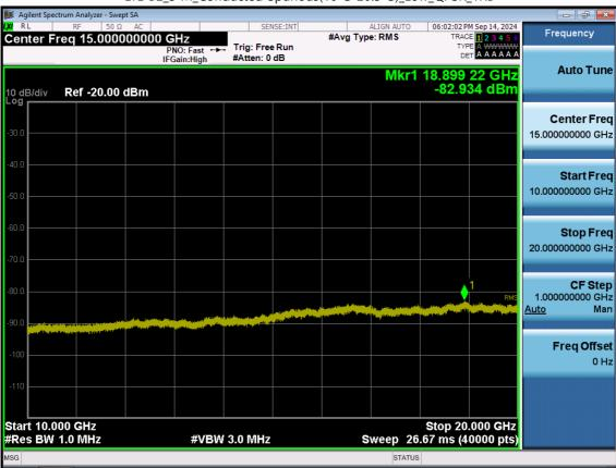
LTE B2\_3 M\_Conducted Spurious(10 G-26.5 G)\_Low\_QPSK\_1RB
