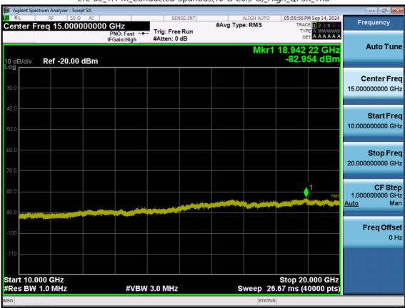
LTE B2\_1.4 M\_Conducted Spurious(10 G-26.5 G)\_High\_QPSK\_1RB
