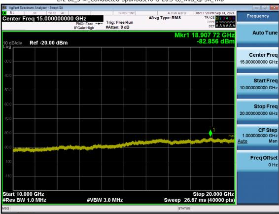
LTE B2\_5 M\_Conducted Spurious(10 G-26.5 G)\_Mid\_QPSK\_1RB
