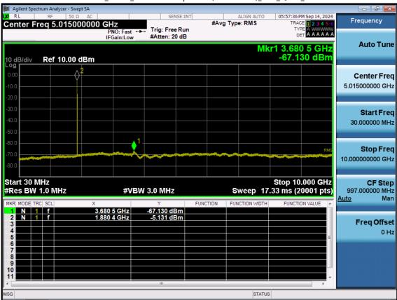
LTE B2\_1.4 M\_Conducted Spurious(30 M-10 G)\_Mid\_QPSK\_1RB
