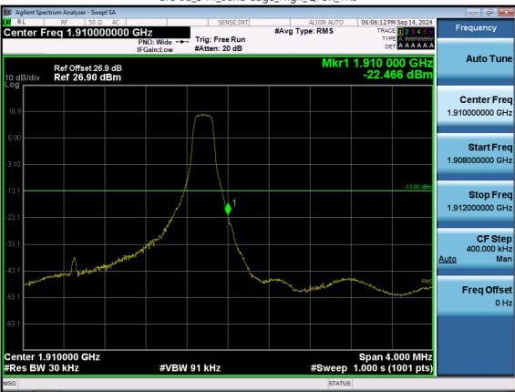
LTE B2\_3 M\_Band Edge\_High\_QPSK\_1RB
