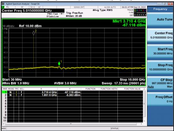
LTE B2\_3 M\_Conducted Spurious(30 M-10 G)\_Low\_QPSK\_1RB
