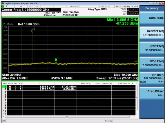
LTE B2\_20 M\_Conducted Spurious(30 M-10 G)\_Mid\_QPSK\_1RB
