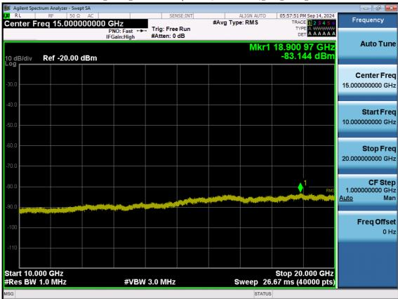
LTE B2\_1.4 M\_Conducted Spurious(10 G-26.5 G)\_Mid\_QPSK\_1RB
