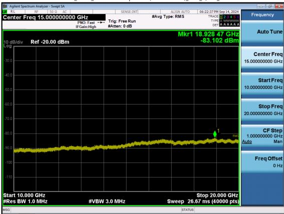
LTE B2\_15 M\_Conducted Spurious(10 G-26.5 G)\_Low\_QPSK\_1RB
