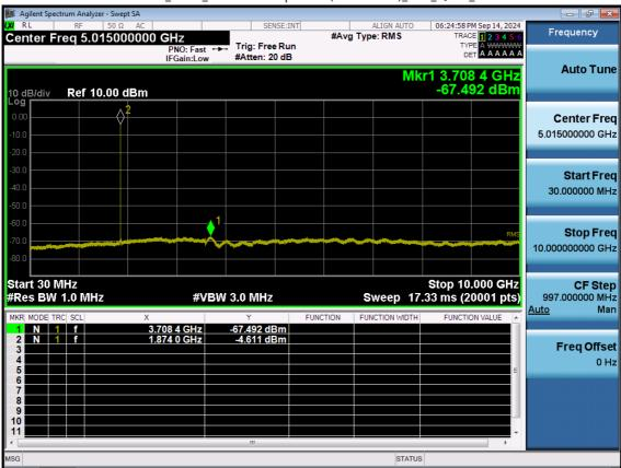
LTE B2\_15 M\_Conducted Spurious(30 M-10 G)\_Mid\_QPSK\_1RB
