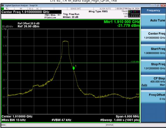
LTE B2\_1.4 M\_Band Edge\_High\_QPSK\_1RB
