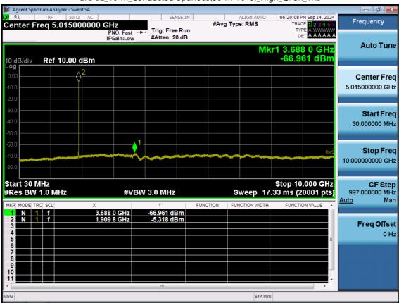
LTE B2\_10 M\_Conducted Spurious(30 M-10 G)\_High\_QPSK\_1RB
