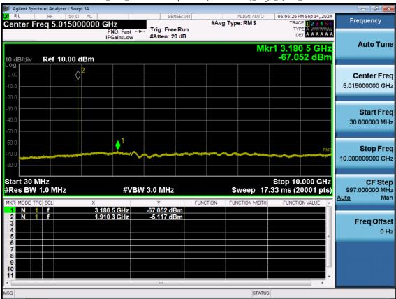
LTE B2\_3 M\_Conducted Spurious(30 M-10 G)\_High\_QPSK\_1RB
