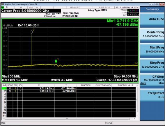
LTE B2\_10 M\_Conducted Spurious(30 M-10 G)\_Low\_QPSK\_1RB
