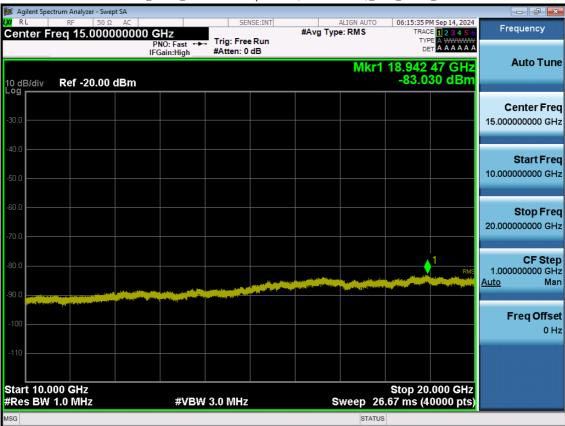
LTE B2\_10 M\_Conducted Spurious(10 G-26.5 G)\_Low\_QPSK\_1RB
