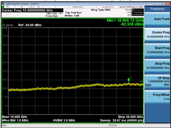
LTE B2\_15 M\_Conducted Spurious(10 G-26.5 G)\_Mid\_QPSK\_1RB
