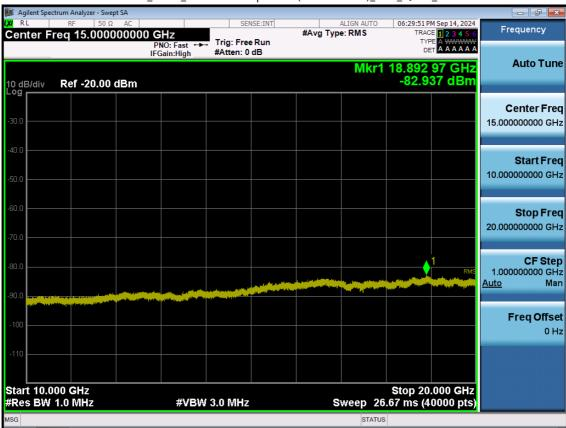
LTE B2\_20 M\_Conducted Spurious(10 G-26.5 G)\_Low\_QPSK\_1RB
