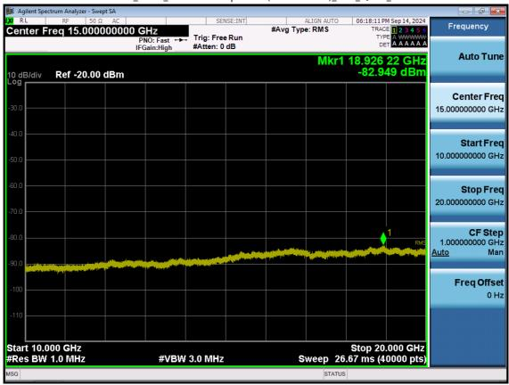
LTE B2\_10 M\_Conducted Spurious(10 G-26.5 G)\_Mid\_QPSK\_1RB
