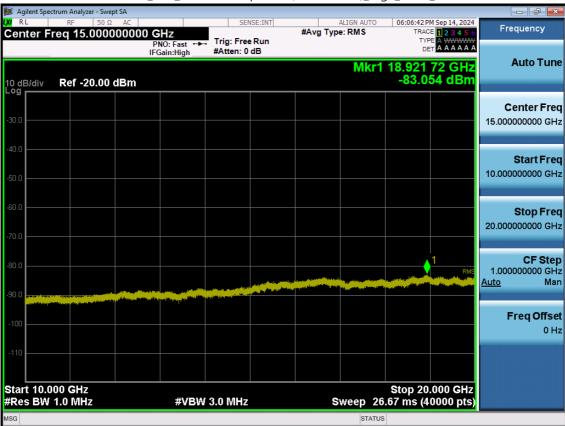
LTE B2\_3 M\_Conducted Spurious(10 G-26.5 G)\_High\_QPSK\_1RB
