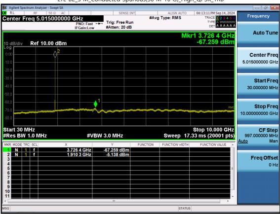
LTE B2\_5 M\_Conducted Spurious(30 M-10 G)\_High\_QPSK\_1RB
