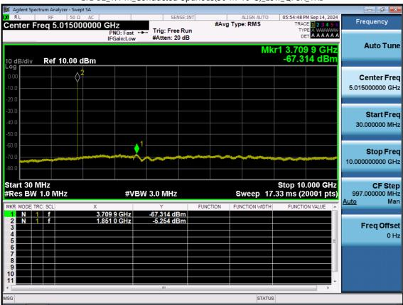
LTE B2\_1.4 M\_Conducted Spurious(30 M-10 G)\_Low\_QPSK\_1RB
