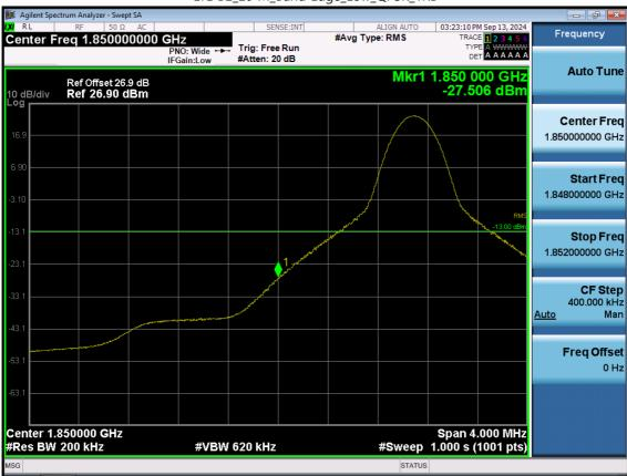
LTE B2\_20 M\_Band Edge\_Low\_QPSK\_1RB
