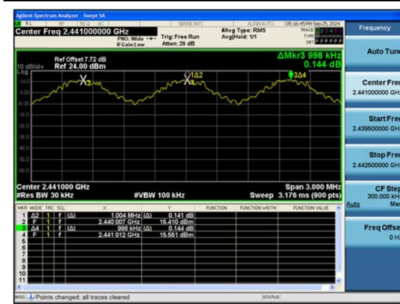
ANT. 1 8DPSK : Channel Separation
