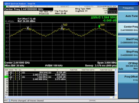
Dual ANT. 2 8DPSK : Channel Separation
