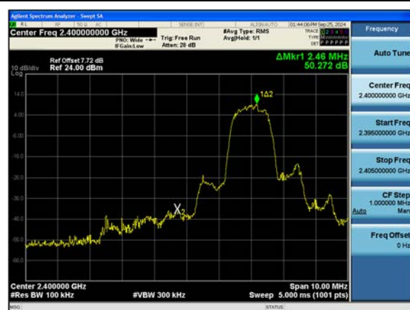
Dual ANT.2 8DPSK Band Edge(Ch. 0)
