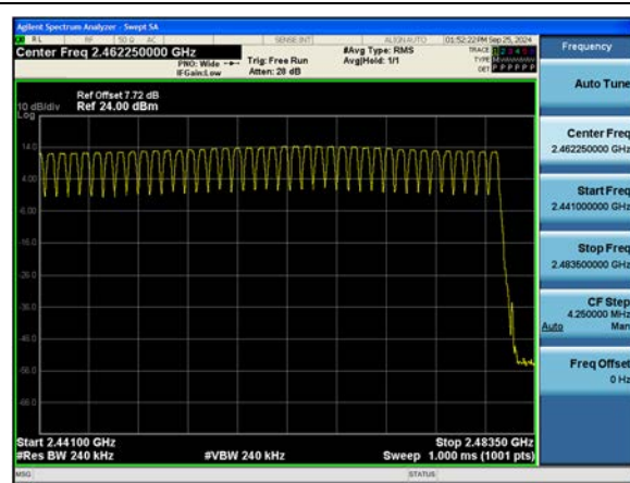
Dual ANT.1 8DPSK (2.441 GHz - 2.483.5 GHz)
