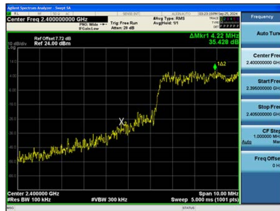
Dual ANT.2 8DPSK Band Edge(Ch. 0)
