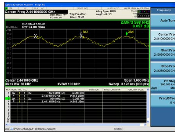
Dual ANT. 1 8DPSK : Channel Separation
