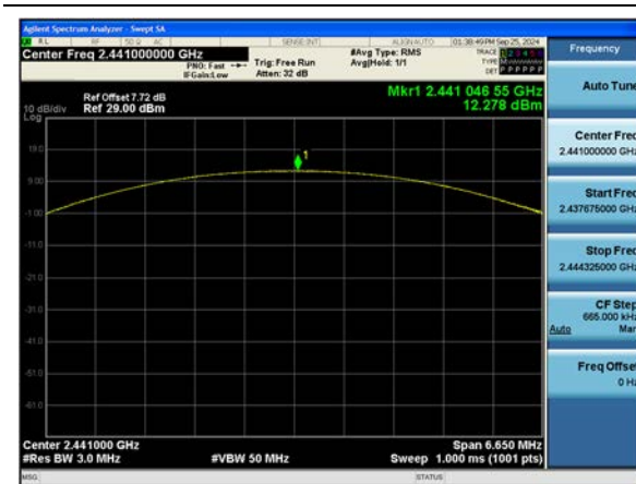
Dual ANT.1 \pi /4DQPSK : Peak Power (Ch. 39)
