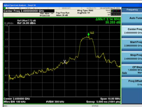
Dual ANT.2 8DPSK Band Edge(Ch. 0)
