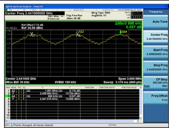
ANT. 2 8DPSK : Channel Separation
