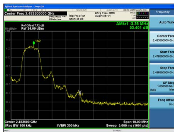
Dual ANT.2 8DPSK Band Edge(Ch. 78)
