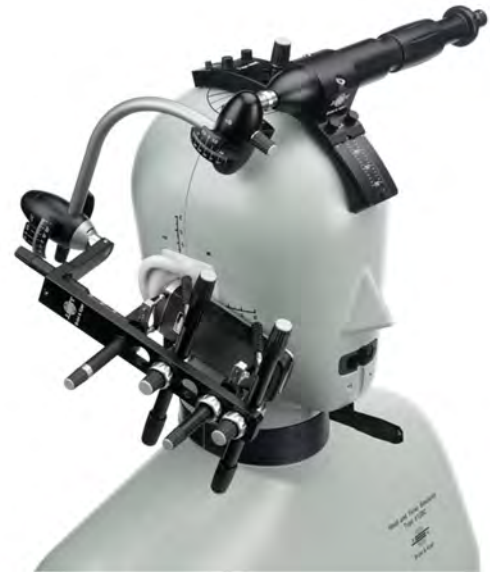
Figure 4-3 Heat and Torso Simulator (with Handset Positioner)
