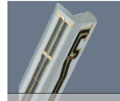
Figure 4-1 E-field Free-space Probe
