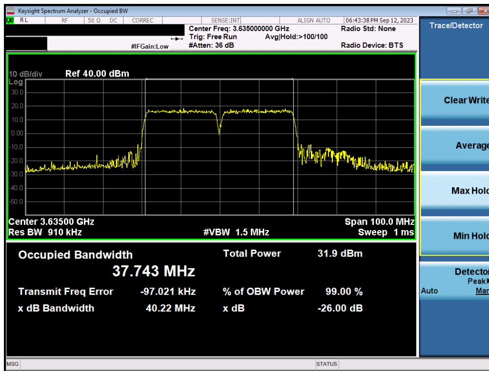
Plot 7-1. Occupied Bandwidth Plot (ULCA LB48 - 20+20MHz QPSK - Full RB Configuration)
