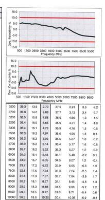
Figure B-1-2 600 – 5800 MHz Head Tissue Equivalent Matter
