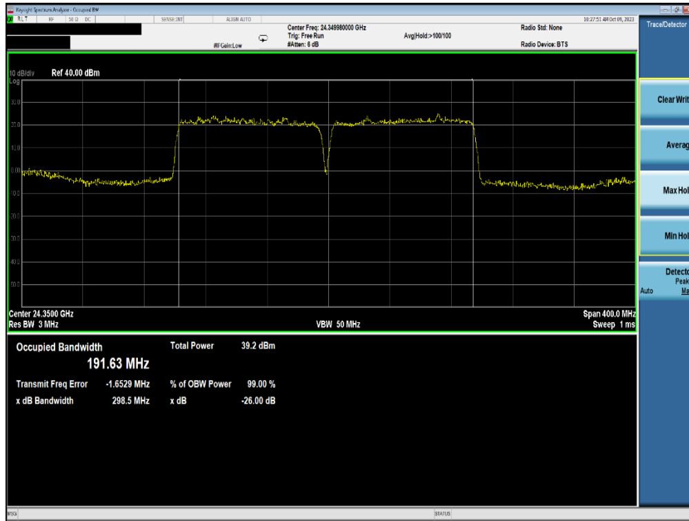
Plot 7-10. Occupied Bandwidth Plot (100MHz-2CC – DFT-s-OFDM \pi/2 BPSK – Mid Channel)
