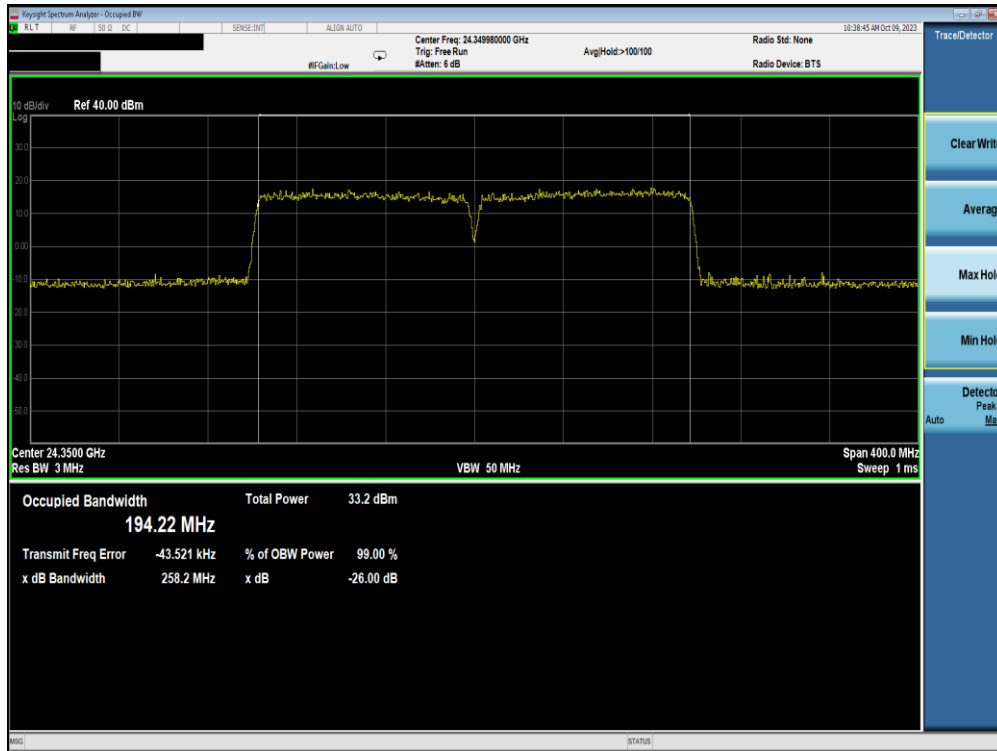
Plot 7-12. Occupied Bandwidth Plot (100MHz-2CC – DFT-s-OFDM 64QAM – Mid Channel)
