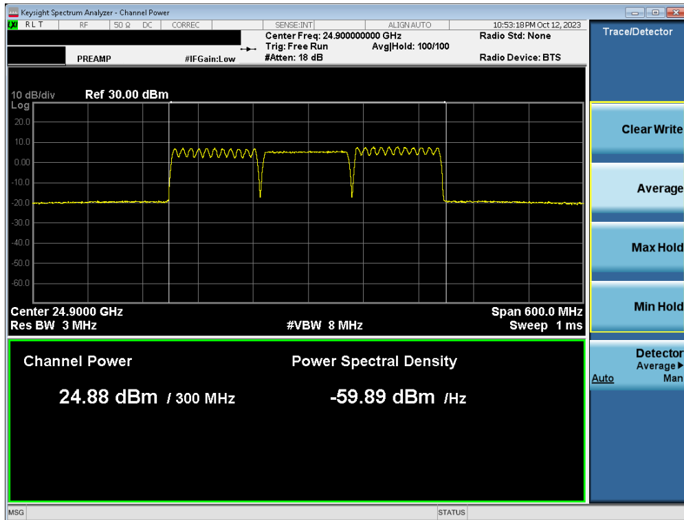
Plot 7-87. Ant 2 EIRP Plot (Band n258-R2 – 100MHz-3CC Low Channel DFT-s-OFDM QPSK)
