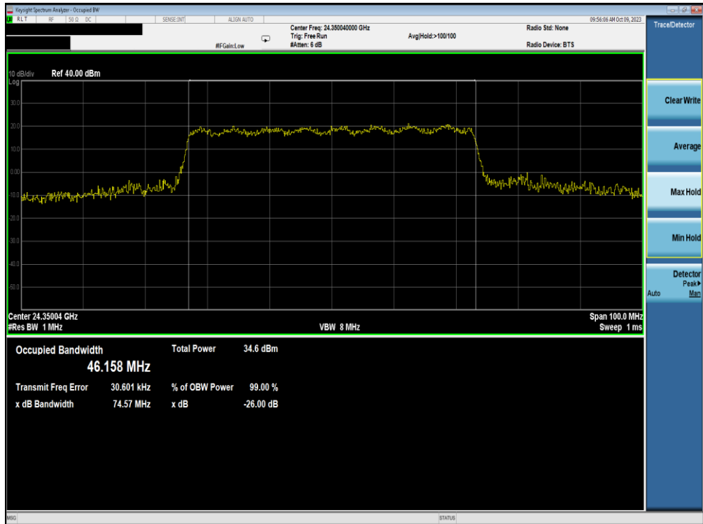
Plot 7-1. Occupied Bandwidth Plot (50MHz-1CC – CP-OFDM QPSK – Mid Channel)
