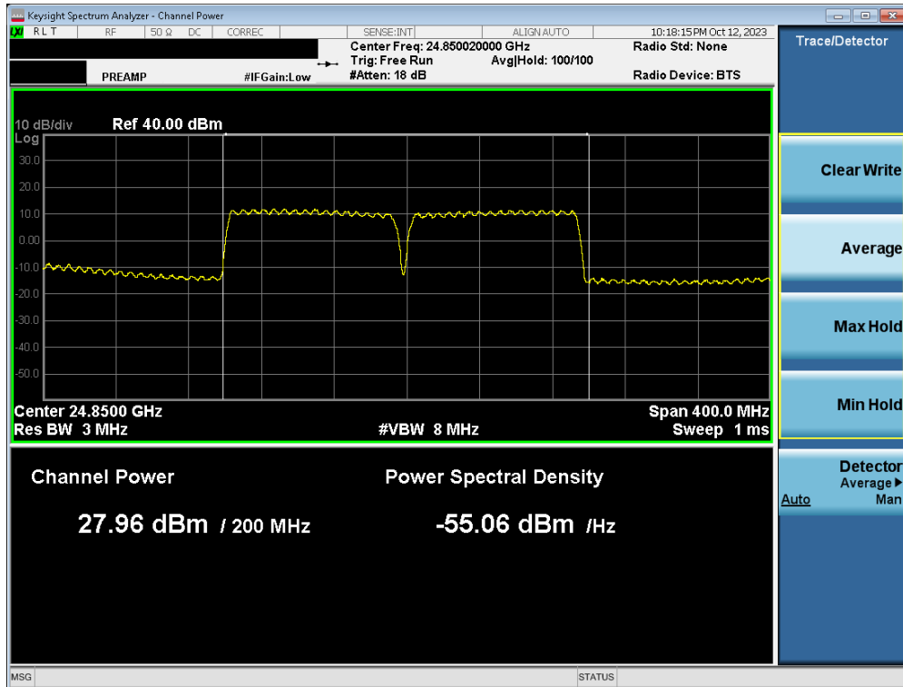
Plot 7-86. Ant 2 EIRP Plot (Band n258-R2 – 100MHz-2CC Low Channel DFT-s-OFDM QPSK)
