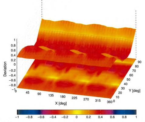
Probe isotropy for  $E_{tot}$ : probe rotated  $\phi = 0^{\circ}$  to 360°, tilted from field propagation direction  $\vec{k}$ Parallel to the field propagation ( $\psi = 0^{\circ} - 90^{\circ}$ ) at 30 GHz: deviation within ±0.37 dB Parallel to the field propagation ( $\psi = 0^{\circ} - 90^{\circ}$ ) at 60 GHz: deviation within ±0.44 dB
