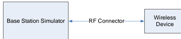
Figure 10-4 Power Measurement Setup – NR FDD
